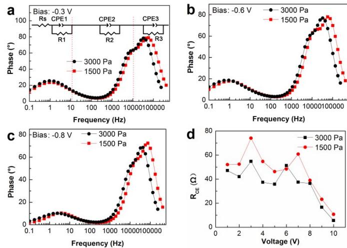
**Figure S6.** Electronic impedance spectroscopy characteristics of the PSCs under illumination. Bode phase plots of devices based on perovskite films fabricated at the pressure of 1500 Pa and 3000 Pa under illumination with a bias at (a) -0.8 V, (b) -0.6 V and (c) -0.3 V. (d) The charge transfer resistance of devices at different biases.
