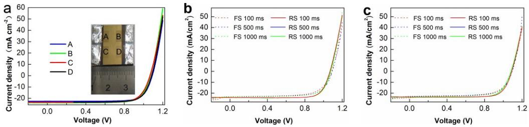
**Figure S5.** (a) The  $J$ - $V$  curves of four devices at the pressure of 1500 Pa on a  $2.5 \times 2.5$  cm substrate. The  $J$ - $V$  curves obtained by reverse and forward scans at a scan step of 23.7 mV and delay time of 100 ms, 500 ms and 1000 ms under a simulated AM 1.5G solar illumination of  $100 \text{ mW/cm}^2$  respectively for the champion cells fabricated at the pressure of (b) 500 Pa and (c) 1500 Pa.
