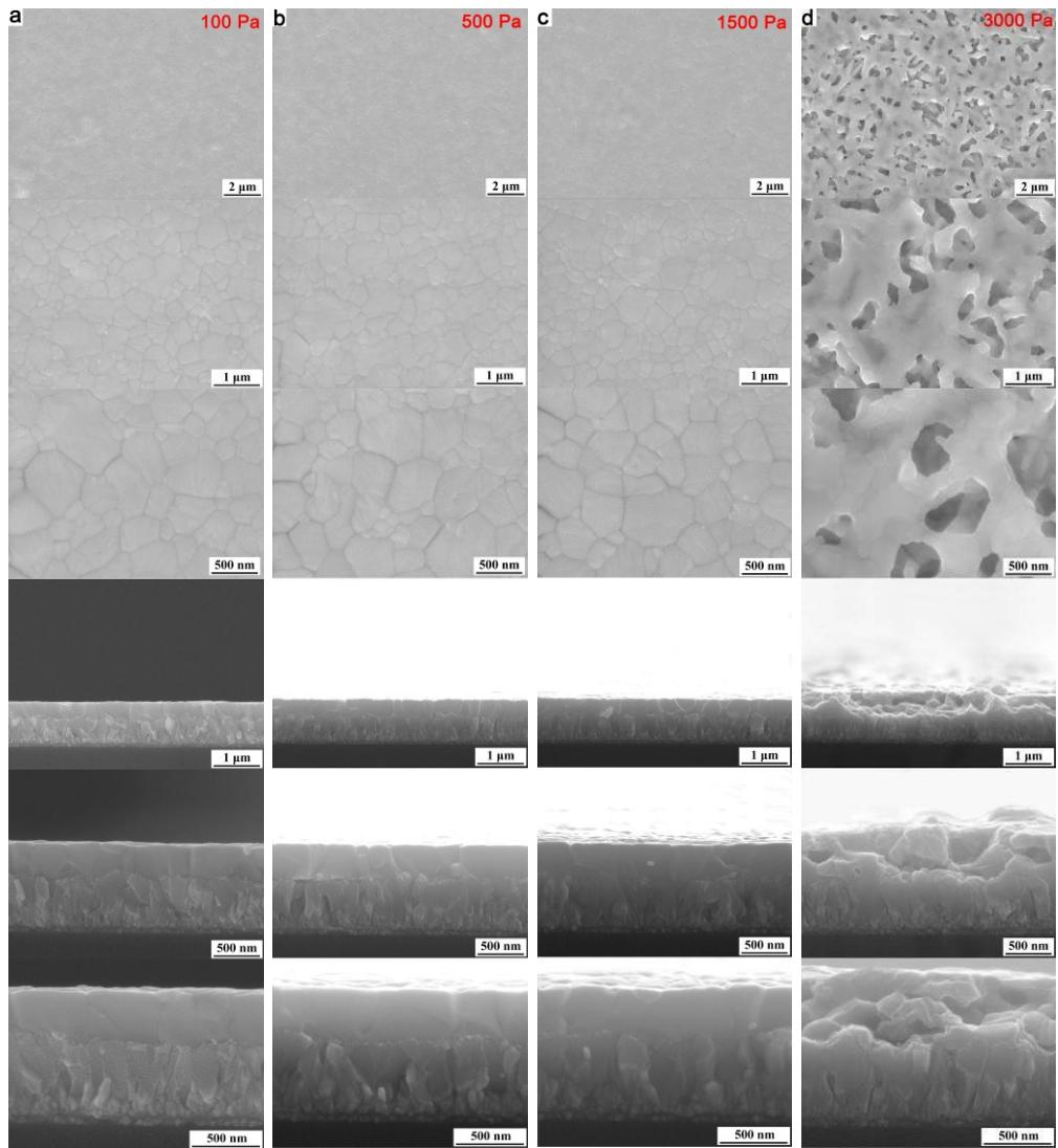
**Figure S2.** Different magnification of the surface and cross-sectional view morphologies for the perovskite films obtained by the GGPM at the pressure of (a) 100 Pa, (b) 500 Pa, (c) 1500 Pa and (d) 3000 Pa.
