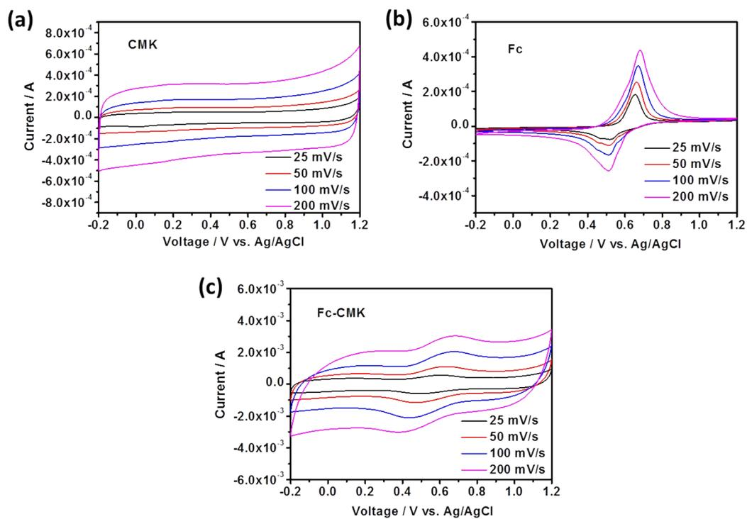
Fig. S4 CV curves of (a) CMK-3, (b) Fc, and (c) Fc-CMK in 0.1 M PBS.
