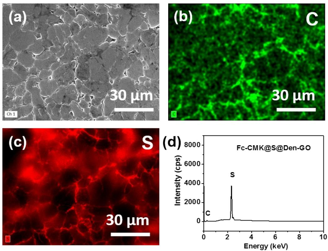
Fig. S13 SEM-EDX analysis of the cycled Li anode paired with the Fc-CMK@S@Den-GO cathode. (a)
