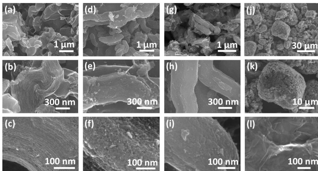
**Fig. S2** SEM images of (a, b, c) CMK-3, (d, e, f) Fc-CMK, (g, h, i) Fc-CMK@S, and (j, k, l) Fc-CMK@S@Den-GO.
