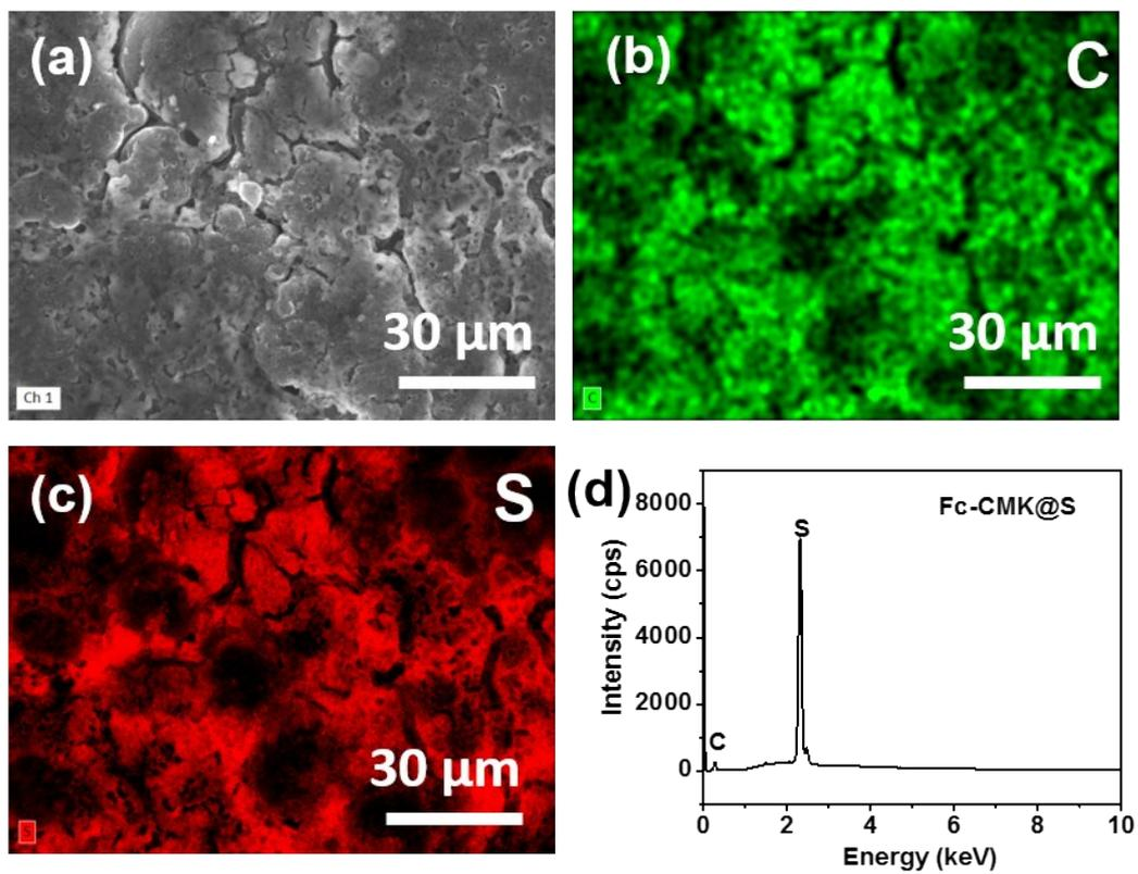
**Fig. S14 SEM-EDX analysis of the cycled Li anode paired with the Fc-CMK@S cathode.** (a) SEM image; elemental maps of (b) C and (c) S; (d) the corresponding EDX spectrum.
