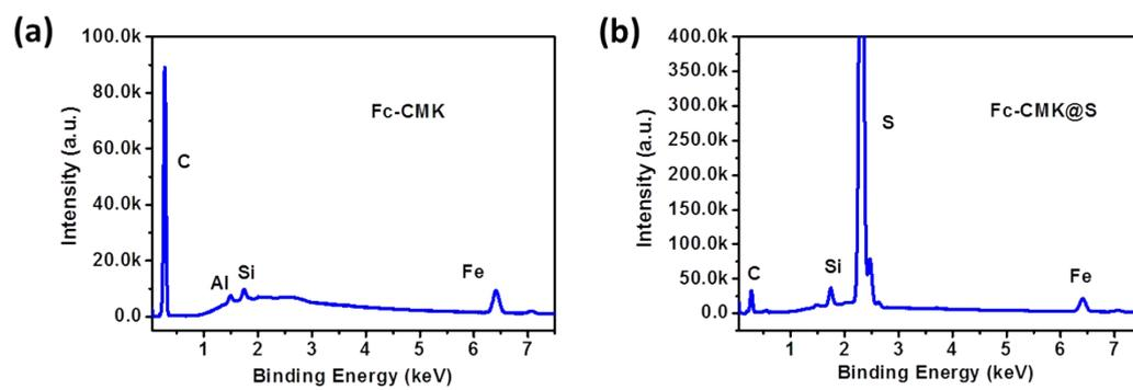
Fig. S3 EDX spectra of (a) Fc-CMK and (b) Fc-CMK@S.
