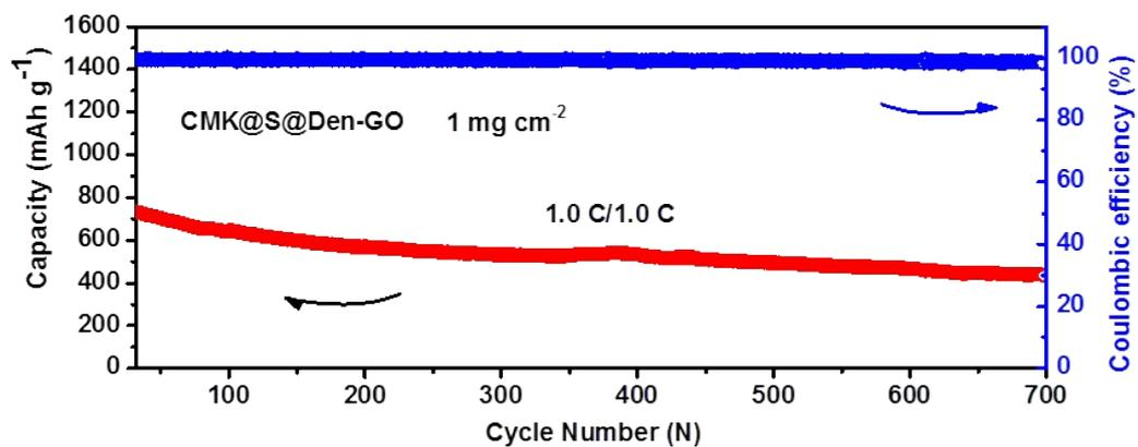
**Fig. S11** Long-term cycling stability of CMK@S@Den-GO at 1.0 C. The S mass loading on the electrodes is  $\sim 1 \text{ mg cm}^{-2}$ .
