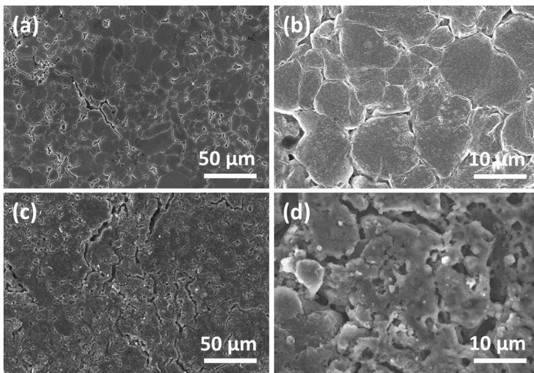
**Fig. S12** SEM images of the Li anodes paired with the (a, b) Fc-CMK@S@Den-GO and (c, d) Fc-CMK@S electrodes after 750 cycles.
