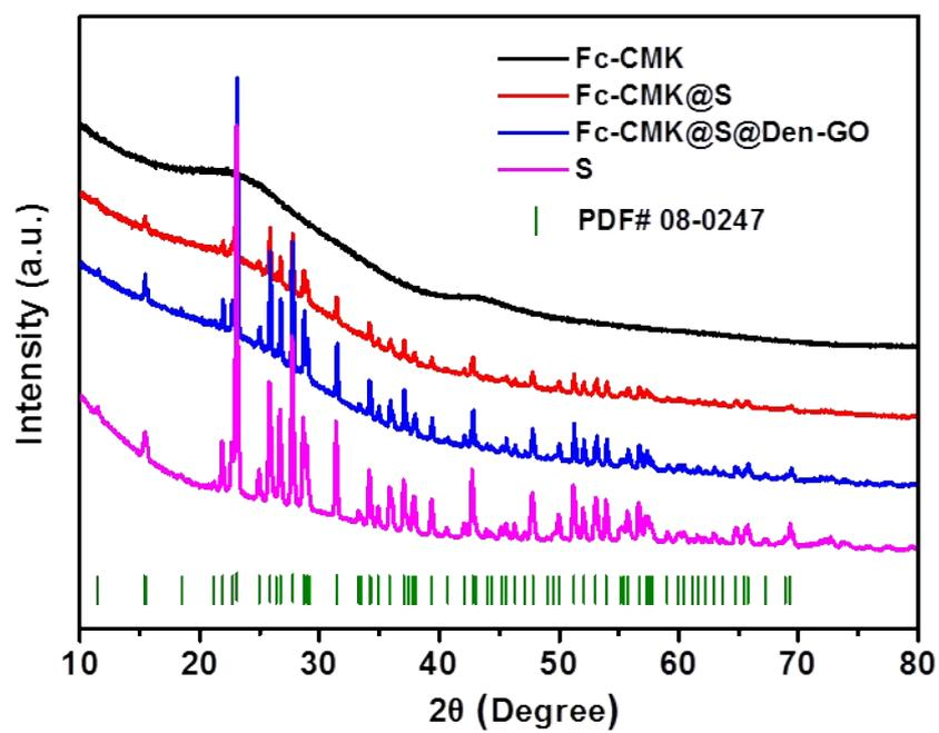
Fig. S6 XRD patterns of Fc-CMK, Fc-CMK@S, Fc-CMK@S@Den-GO, and S (PDF#08-0247).
