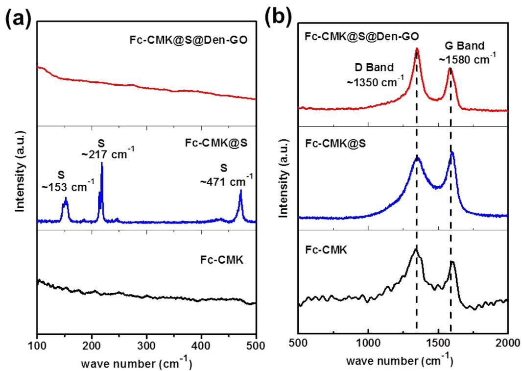
Fig. S7 Raman spectroscopy of Fc-CMK, Fc-CMK@S, and Fc-CMK@S@Den-GO.
