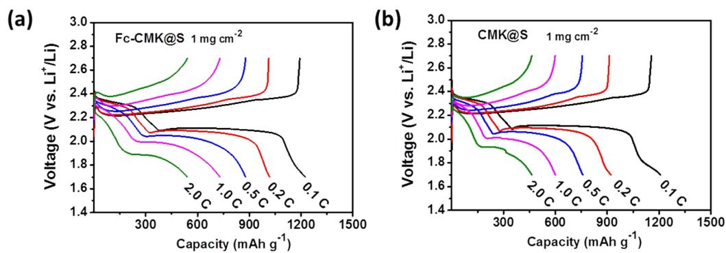
**Fig. S10** Discharging/charging voltage profiles of (a) Fc-CMK@S and (b) CMK@S. The S content of the materials are 76.7 wt% and 67.0 wt% for Fc-CMK@S and CMK@S, respectively. The S mass loading on the electrodes is  $\sim 1 \text{ mg cm}^{-2}$ .
