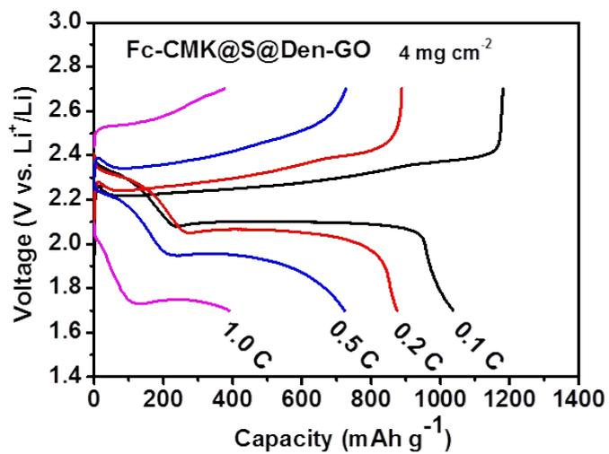
**Fig. S17** Discharging/charging voltage profiles of Fc-CMK@S@Den-GO with S mass loading of 4 mg cm<sup>-2</sup>
