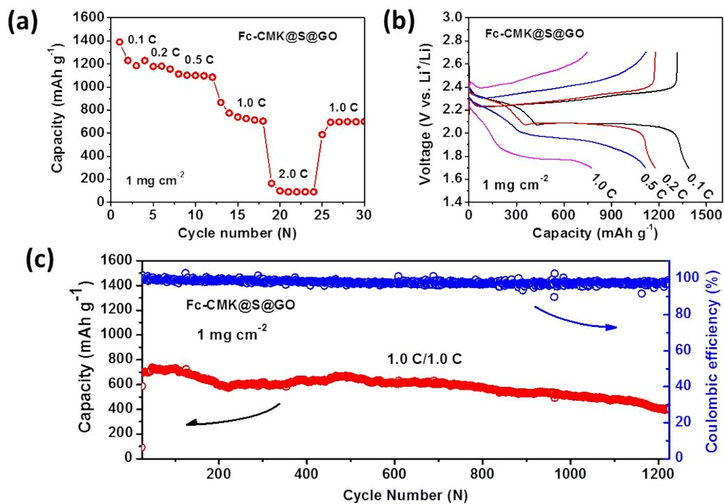
Fig. S16 Electrochemical performance of a Li-S cell with the Fc-CMK@S@GO material as the cathode.
