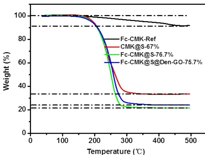
**Fig. S9** The TGA curves of Fc-CMK, CMK@S, Fc-CMK@S, and Fc-CMK@S@Den-GO. The weight loss for
