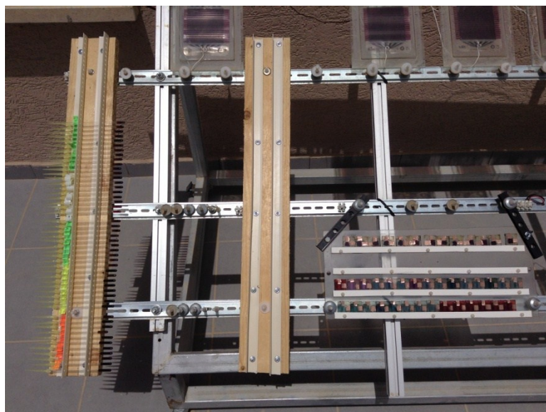
Fig. S1. Photograph of the sample stage for outdoor aging of organic solar cells and thin films sealed between the glass plates or inside the glass tubes.
