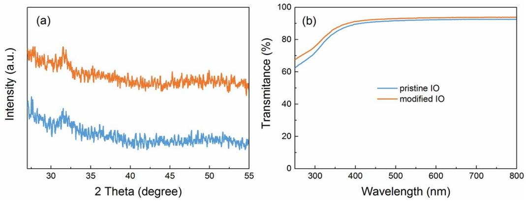
Figure S3. (a) XRD patterns and (b) UV-vis transmittance spectra of the pristine and modified IO films (annealed at 200 °C).
