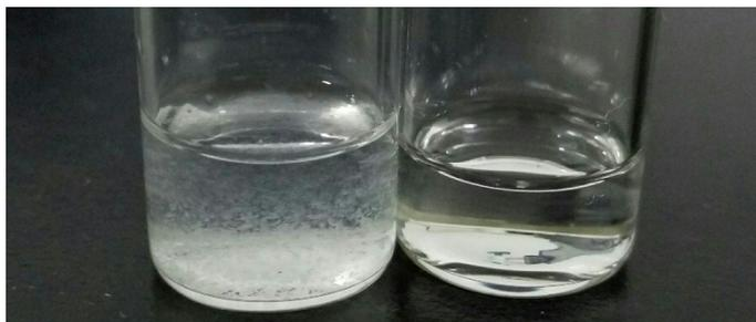
Figure S1. Photographs of  $\text{In}_2\text{O}_3$  precursors with (right) and without (left) acetone stored for days.
