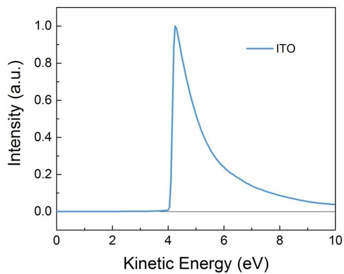
Figure S5. Ultraviolet photoelectron spectrum of the dried ITO substrate without any treatment.
