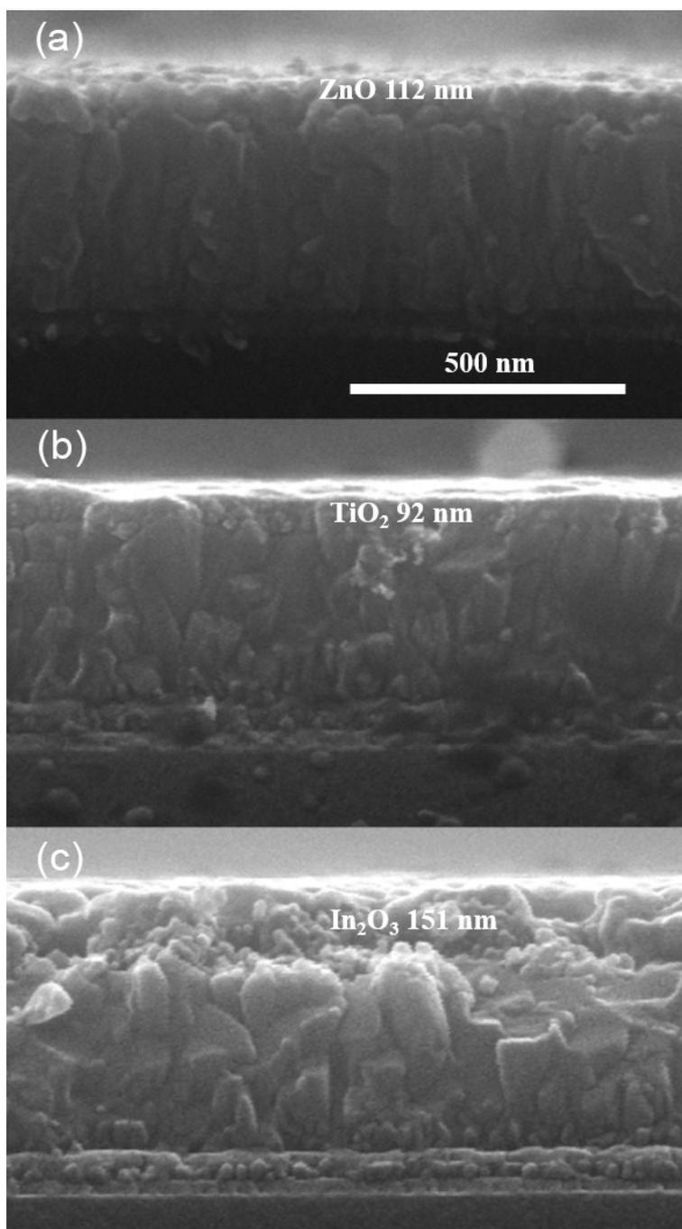
Figure S8. Cross-sectional SEM images of (a) ZnO, (b) TiO<sub>2</sub> and (c) In<sub>2</sub>O<sub>3</sub> films on FTO substrates for the PEC test.
