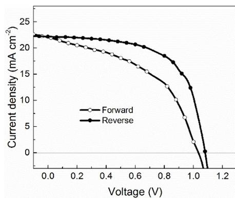
Figure S7. J-V curves of IO based perovskite solar cells measured by reverse and forward scans.
