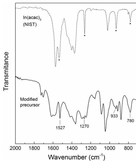
Figure S2. FI-IR spectrum of the modified IO precursor and the standard spectrum of In(acac)<sub>3</sub> from National Institute of Standard and Technology (NIST).
