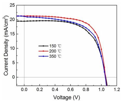
Figure S4. J-V curves of PSCs based on IO films annealed at 150 °C, 200 °C and 350°C.
