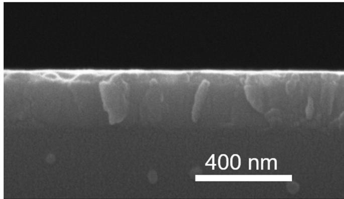
Figure S6. Cross-sectional SEM image of IO film spin-coated on ITO substrate with a thickness of ~40 nm.
