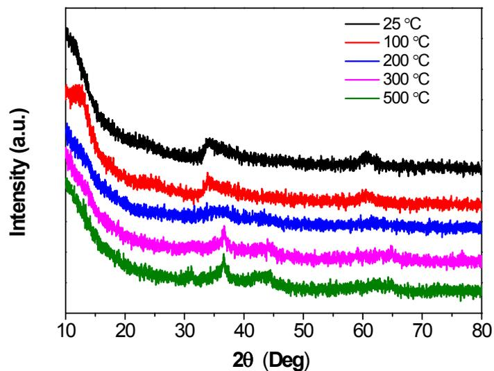
Fig. S8 XRD patterns of samples annealed in N<sub>2</sub> for 2 h at different temperatures.
