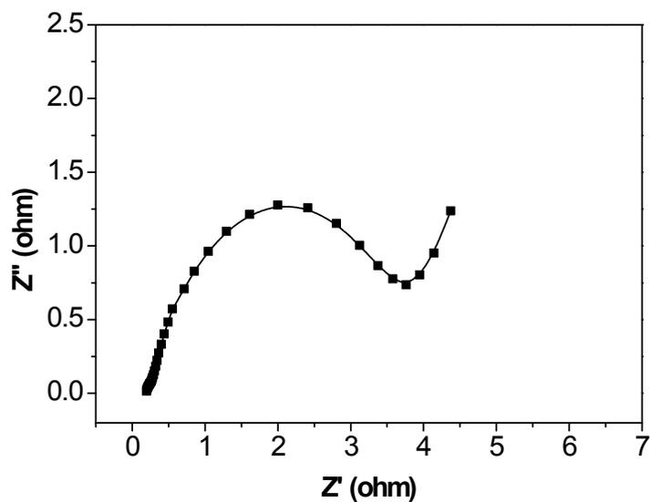
**Fig. S12** Nyquist plot of the Co-Ni-W-B-O/20rGO//rGO asymmetric supercapacitor.
