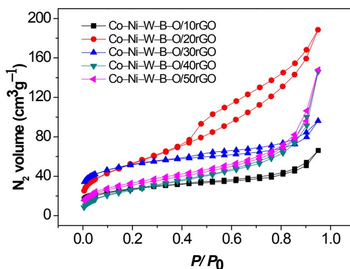
**Fig. S5** Nitrogen adsorption isotherms of Co-Ni-W-B-O/rGO samples containing different amounts of rGO.
