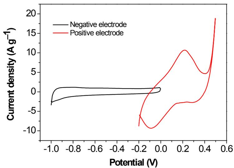
Fig. S9 CV curves of the negative electrode and positive electrode at the scan rate of 5 mV s<sup>-1</sup>
