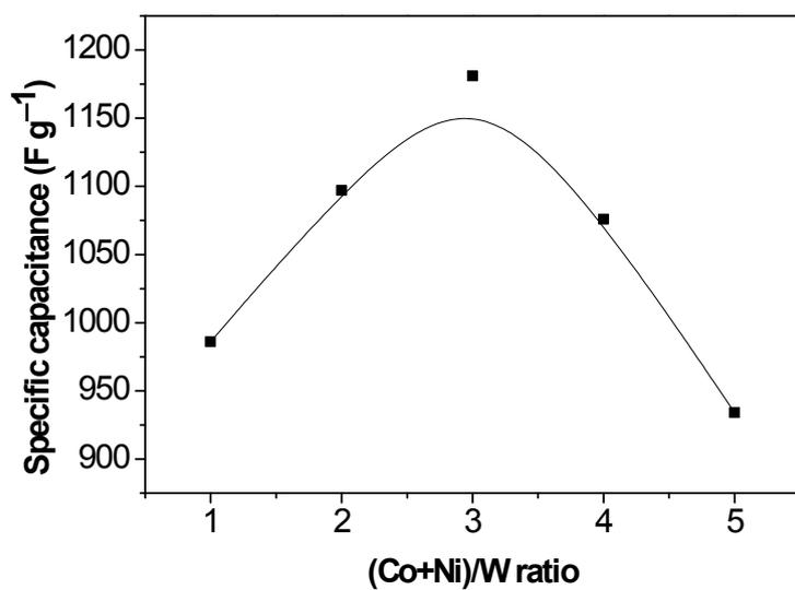
**Fig. S7** Effect of (Co+Ni)/W molar ratio on the specific capacitance of the Co–Ni–W–B–O/20 rGO electrode.
