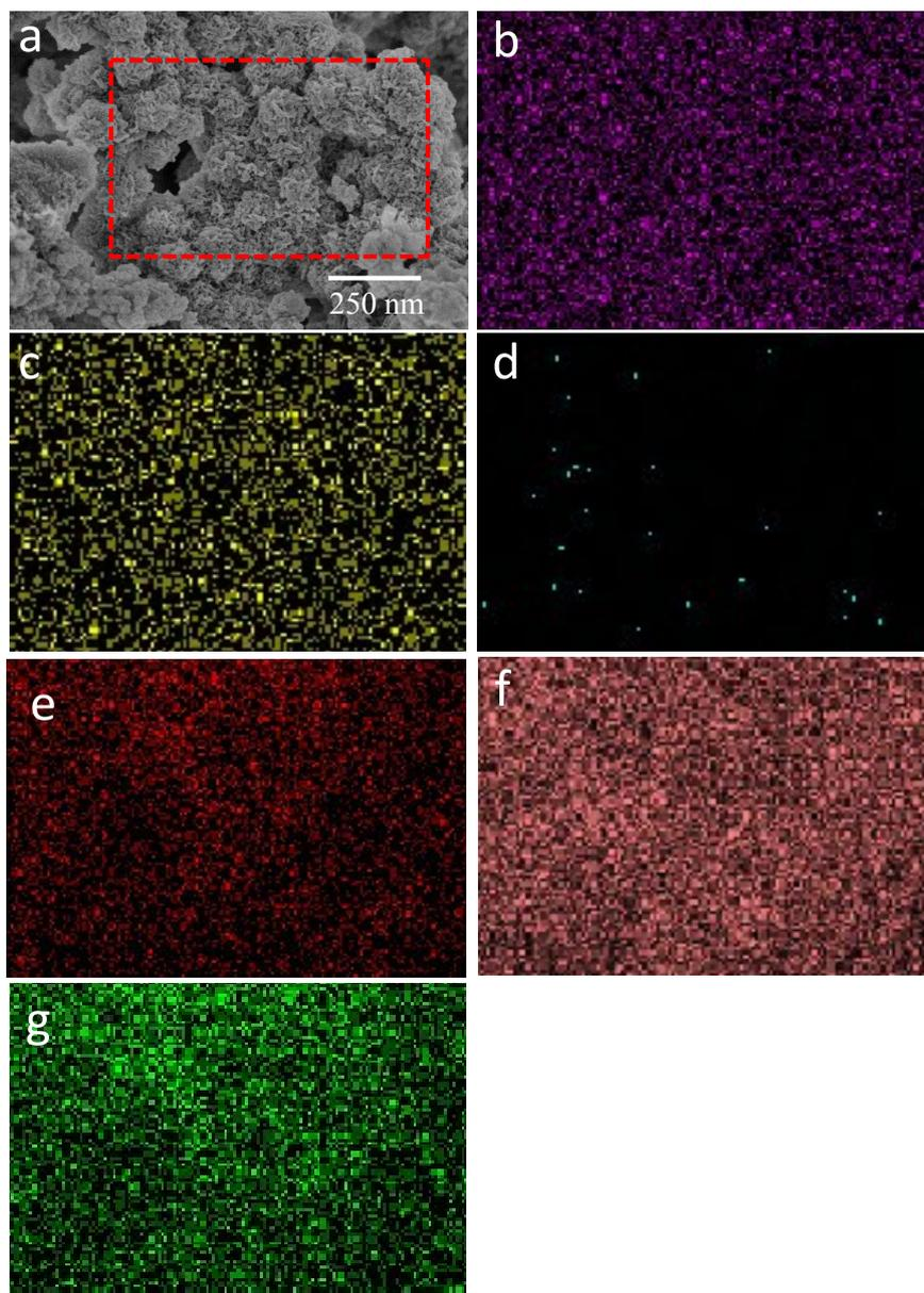
**Fig. S1** SEM images of Co–Ni–W–O/rGO and EDX mapping images of (b) Co, (c) Ni, (d) W, (e) B, (f) O, and (g) C.
