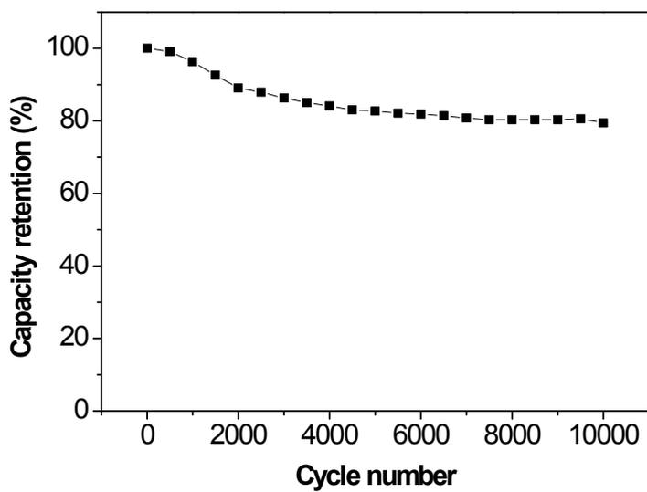
**Fig. S13** Cycle stability of the Co-Ni-W-B-O/20rGO//rGO asymmetric supercapacitor at a current density of  $5 \text{ A g}^{-1}$  for 10000 cycles.
