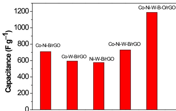
**Fig S4** Capacitance of Co-Ni-B/rGO, Co-W-B/rGO, Ni-W-B/rGO, Co-Ni-W-B/rGO, and Co-Ni-W-B-O/rGO, obtained from their charge-discharge curves.
