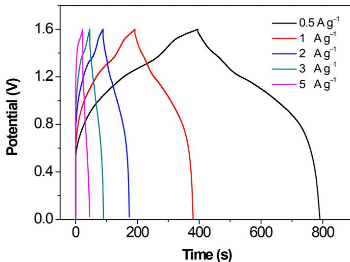
**Fig. S10** Galvanostatic charge–discharge curves of the Co–Ni–W–B–O/20rGO//rGO asymmetric supercapacitor, measured at different current densities.
