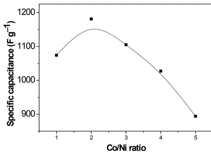
**Fig. S6** Effect of Co/Ni molar ratio on the specific capacitance of the Co–Ni–W–B–O/20rGO electrode.
