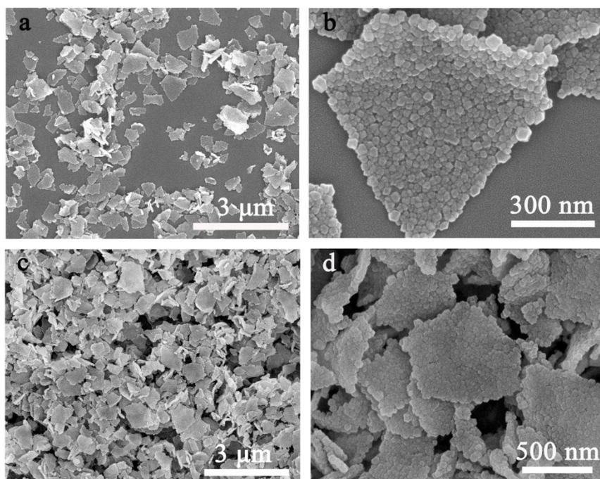
**Figure S4** SEM images of (a, b) GO/ZIF-8@ZIF-67-L and (c, d) GO/ZIF-8@ZIF-67-H using different concentrations of Co ions solution as a Co source.
