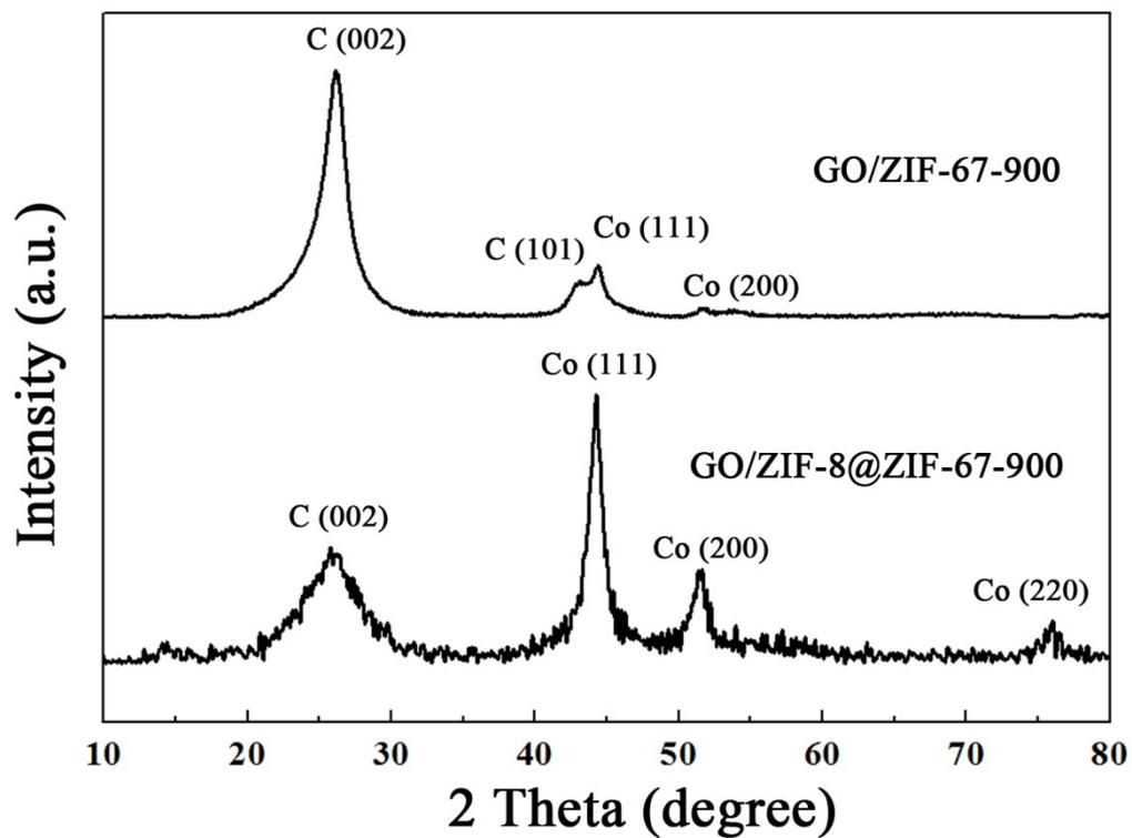
**Figure S8** XRD patterns of cobalt/carbon composites synthesized by carbonization of GO/ZIF-8@ZIF-67 and GO/ZIF-67 at 900 °C respectively.
