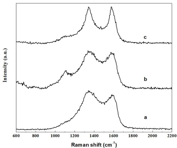
**Figure S11** Raman spectra of (a) GO/ZIF-8-900, (b) GO/ZIF-8-67-900 and (c) GO/ZIF-67-900. As the ratio of cobalt to zinc increases, the  $I_D/I_G$  decreases, indicating the increasing graphitization degree of the carbon composites. The band at around 1100 cm<sup>-1</sup> is from the glass substrate for loading of the samples.
