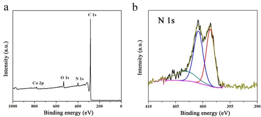
**Figure S10** (a) XPS spectrum and (b) high resolution N 1s spectrum for GO/ZIF-67-900.
