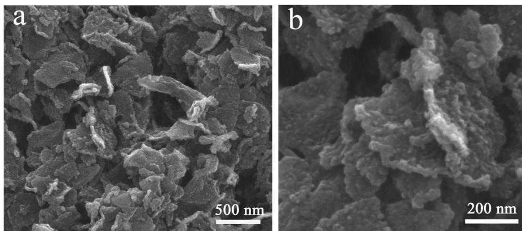
**Figure S6** SEM images of GO/ZIF-8@ZIF-67-900 synthesized by carbonization of GO/ZIF-8@ZIF-67 at 900 °C in Ar followed by acid etching.
