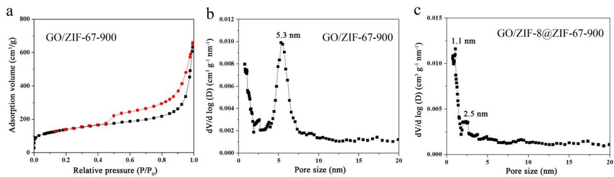
**Figure S12** (a) N<sub>2</sub> sorption isotherms and (b) NLDFT pore size distributions for GO/ZIF-67-900. (c) NLDFT pore size distributions for GO/ZIF-8@ZIF-67-900.
