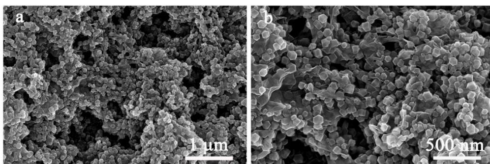
**Figure S1** (a, b) SEM images of GO/ZIF-67 synthesized by direct deposition of ZIF-67 on GO.
