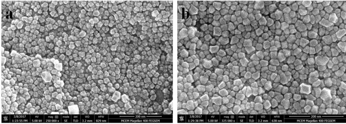
**Figure S2** High resolution SEM images of (a) GO/ZIF-8 and (b) GO/ZIF-8@ZIF-67. The SEM images reveal that the distance between the ZIF crystals become smaller after coating of ZIF-67, indicating a successful deposition of ZIF-67 on the surface of ZIF-8.
