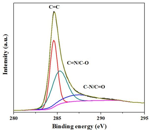
**Figure S9** The high-resolution C 1s spectrum of GO/ZIF-8@ZIF-67-900. For C 1s spectrum, the dominated peak positioned at 284.58 eV is attributed to C=C, while the peaks at 285.24 and 287.25 eV are ascribed to C=N/C-O and C-N/C=O respectively.
