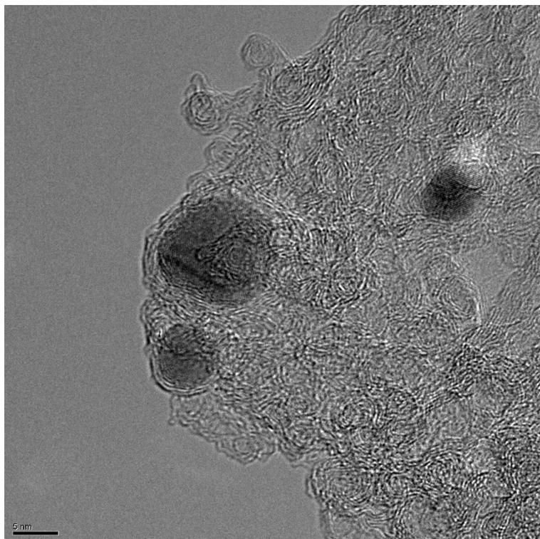
**Figure S7** High-resolution TEM image of GO/ZIF-8@ZIF-67-900. The high crystalline cobalt nanoparticles were encased by the graphitic carbon layer.
