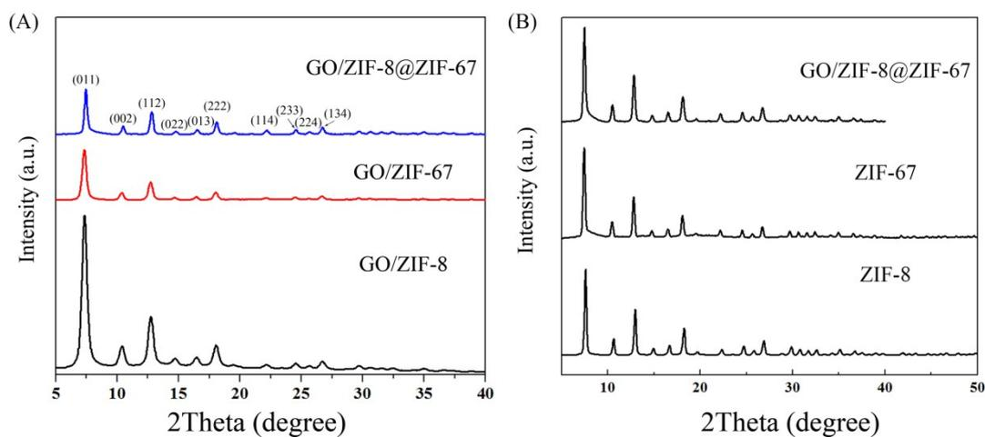
**Figure S3** XRD patterns of (A) GO/ZIF-8, GO/ZIF-67 and GO/ZIF-8@ZIF-67; and (B) ZIF-8, ZIF-67 and GO/ZIF-8@ZIF-67, respectively. All the materials reveal the typical diffraction peaks of ZIF.
