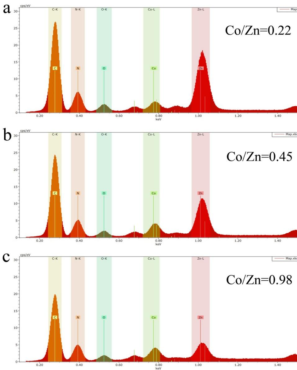
**Figure S5** EDX spectra for (a) GO/ZIF-8@ZIF-67-L, (b) GO/ZIF-8@ZIF-67 and (c) GO/ZIF-8@ZIF-67-H from the SEM images. The atom ratio of Co to Zn in the GO/MOF composites increases as the initial concentrations of Co ions solution increase.
