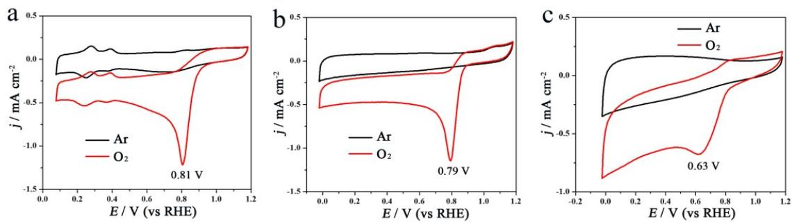
**Figure S14** CV curves for Pt/C, GO/ZIF-67-900 and GO/ZIF-8-900 respectively in Ar (or O<sub>2</sub>)-saturated 0.1 M KOH solution
