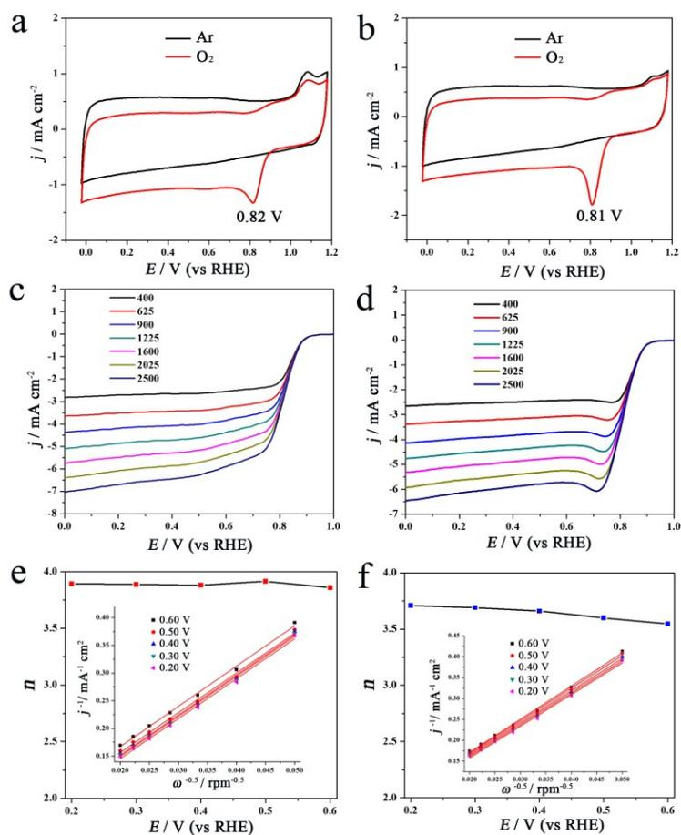
**Figure S15** CV curves for (a) GO/ZIF-8@ZIF-67-L-900 and (b) GO/ZIF-8@ZIF-67-H-900 in 0.1 M KOH solution. LSV curves for (c) GO/ZIF-8@ZIF-67-L-900 and (d) GO/ZIF-8@ZIF-67-H-900 at different rotating speeds (400-2500 rpm). Electron transfer number for (e) GO/ZIF-8@ZIF-67-L-900 and (f) GO/ZIF-8@ZIF-67-H-900 calculated from K-L plots (insets).
