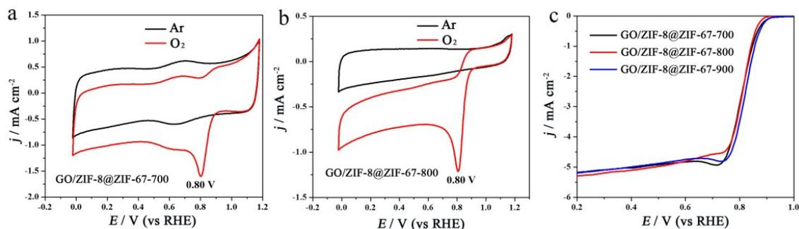
**Figure S13** Cyclic voltammetry (CV) curves for (a) GO/ZIF-8@ZIF-67-700 and (b) GO/ZIF-8@ZIF-67-800 in Ar (or O<sub>2</sub>)-saturated 0.1 M KOH solution. (c) Linear scan voltammogram (LSV) curves for GO/ZIF-8@ZIF-67-700, GO/ZIF-8@ZIF-67-800 and GO/ZIF-8@ZIF-67-900 respectively in O<sub>2</sub>-saturated 0.1 M KOH solution with a rotating speed of 1600 rpm.
