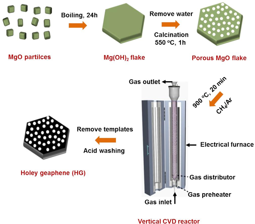
**Fig. S1.** Schematic illustration of preparation process of holey graphene (HG).
