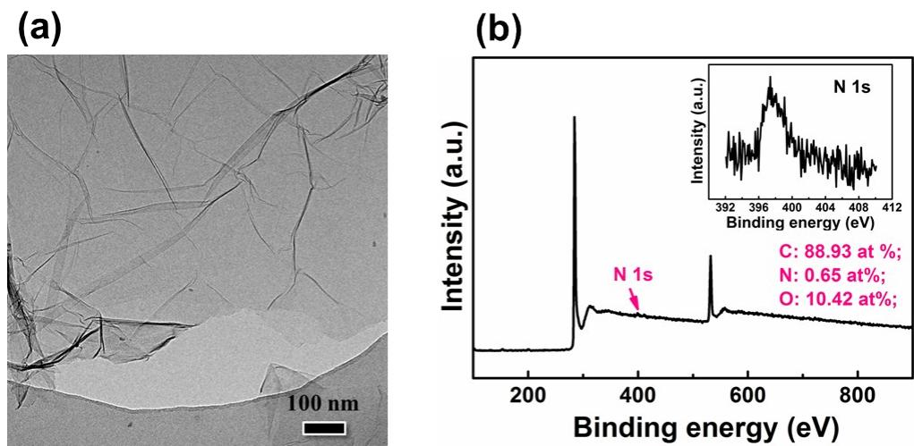
**Fig. S5.** (a) A TEM image of N-rGO, showing few in-plane edges in the graphene layers. (b)
