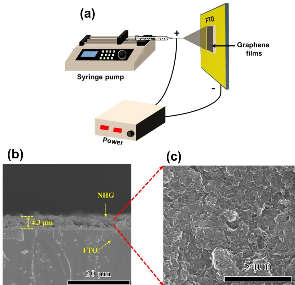
**Fig. S6.** A schematic diagram of the e-spray setup used for NHG counter electrode film fabrication (a) and SEM images of NHG CEs on FTO substrates (b, c).
