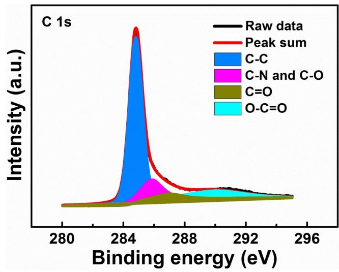
**Fig. S4.** A high resolution spectra of C1s for NHG-2.
