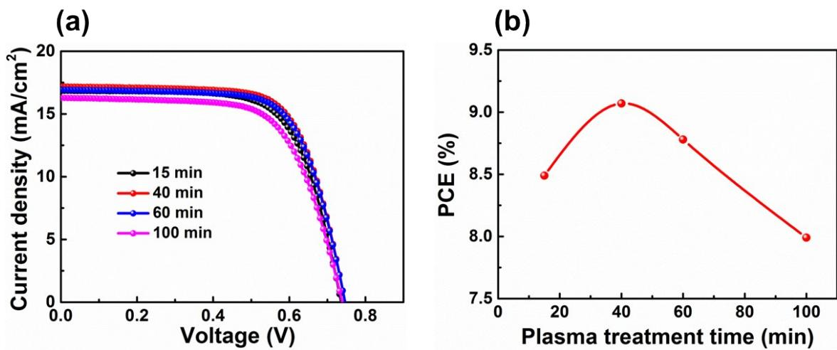
**Fig. S11.** (a) Current-voltage characteristics of the DSSCs based on NHG electrodes with different plasma treatment time. (b) Plot of the PCE versus N2 plasma treatment time.
