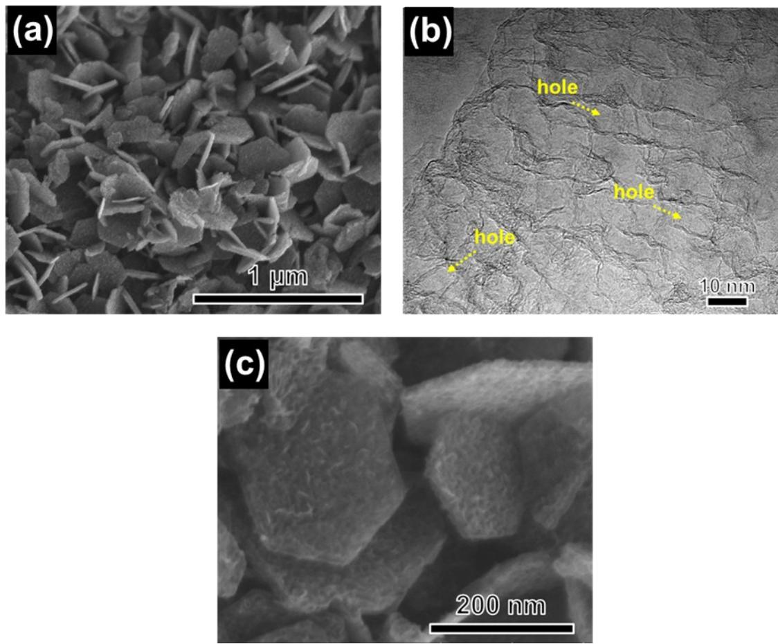
**Fig. S2.** SEM (a) and TEM (b) images of pristine HG. c) A SEM image of NHG.
