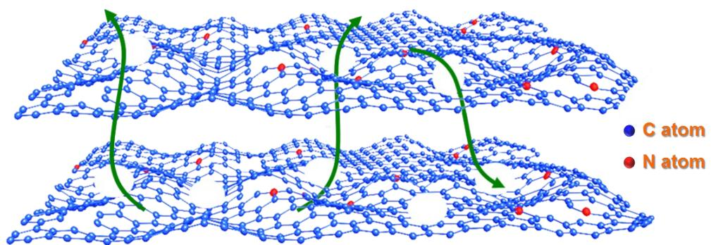
**Fig. S3.** The schematic illustration of the ion-diffusion pathway across the hole.
