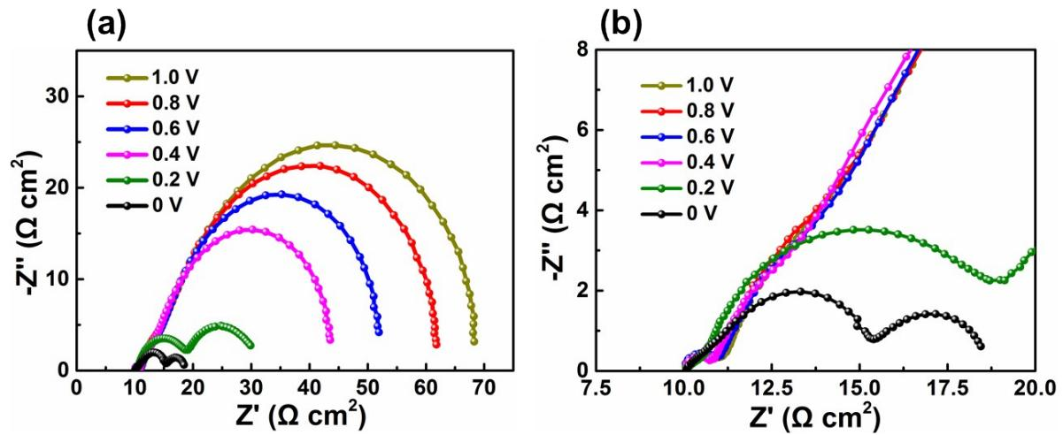
**Fig. S9.** (a) Nyquist plots of impedance spectra on symmetrical dummy cell with NHG-2 electrode at various applied biases. (b) An expansion of the high frequency region. The legend in (b) is for (a) as well.
