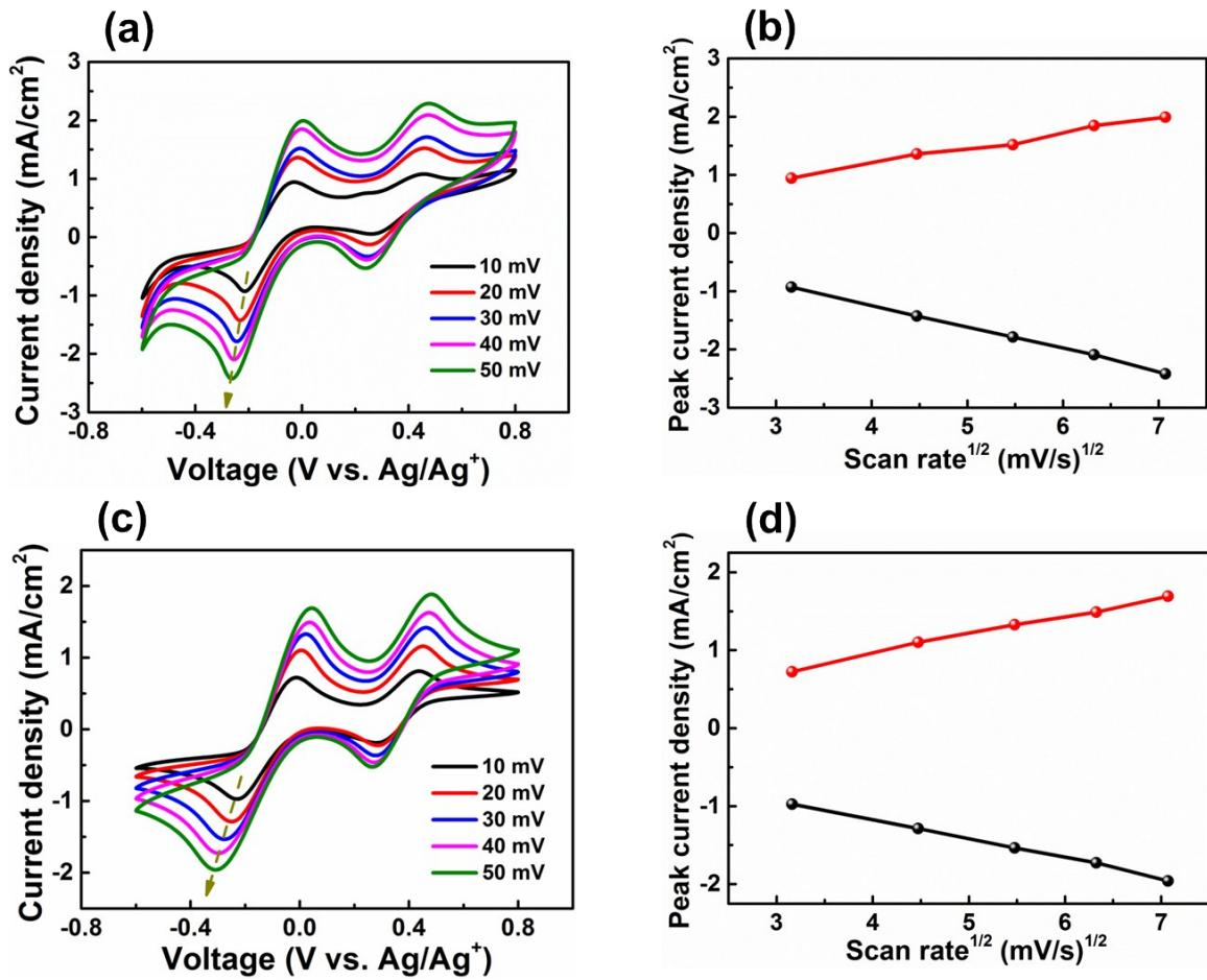
**Fig. S7.** Cyclic voltammograms curves of (a) NHG-2 electrode and (c) Pt electrode at various scanning rates (10, 20, 30, 40, and 50 mV/s), respectively. The peak current density of the left peak pairs as a function of the square root of the scan rates for NHG-2 (b) and Pt (d) electrode, respectively.
