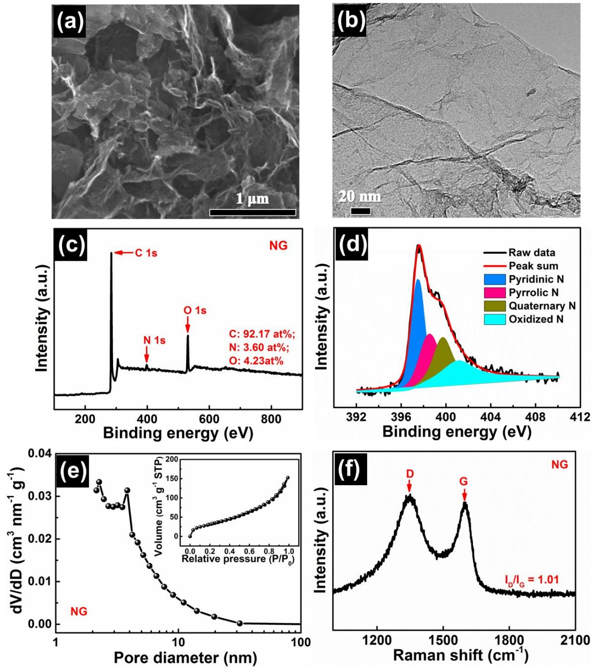
**Fig. S13.** (a) SEM and (b) TEM images of NG, showing few in-plane holes in the graphene layers. (c) The XPS survey of NG. (d) The high-resolution N1s XPS spectrum of NG. (e) The N<sub>2</sub> sorption isotherms and pore size distribution of NG (inset). (f) Raman spectra of NG.
