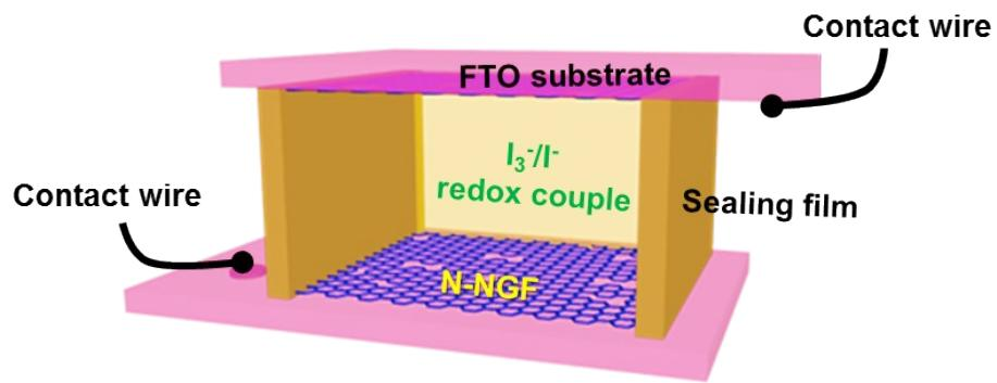
**Fig. S8.** Schematic structure of a symmetric cell symmetrical dummy cell using two identical electrodes.
