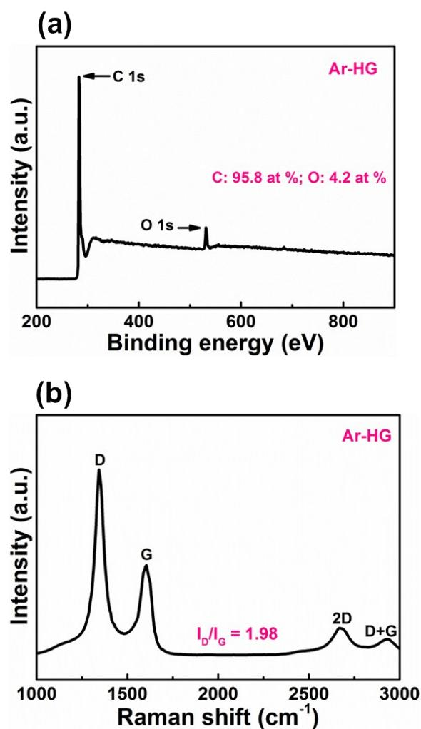
**Fig. S12.** (a) XPS survey of Ar-HG. (b) Raman spectra of Ar-HG.
