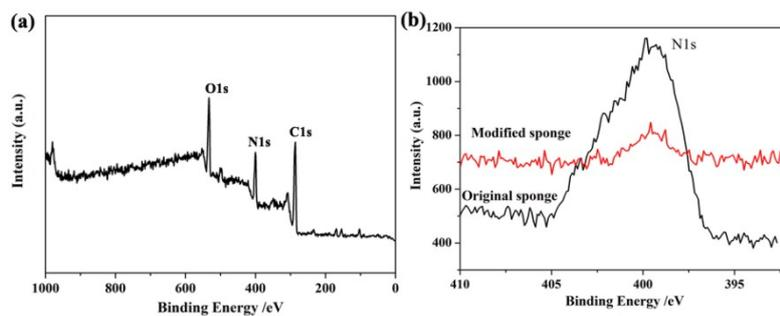
**Figure S2** (a) XPS survey spectra of the pristine melamine sponge. (b) N1s high resolution spectrum of the original and the modified melamine sponge.
