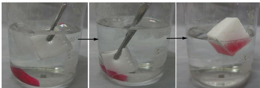
**Figure S6** The prepared superhydrophobic sponge can selective collect oils from ice water mixtures.
