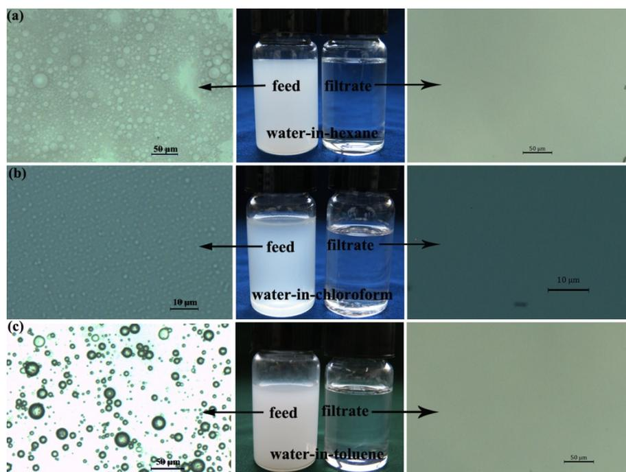
**Figure S11.** Microscope images and digital photos of the separation results for other three types of water-in-oil emulsions, including (a) water-in-hexane emulsion, (b) water-in-chloroform emulsion and (c) water-in-toluene emulsion
