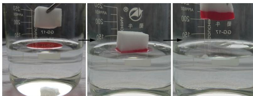
**Figure S4** Selective collection of floating oils with superhydrophobic sponge.
