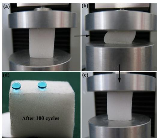
**Figure S3** (a-c) Sequential digital images showing compressibility of the superhydrophobic melamine sponge. (d) The melamine sponge still shows superhydrophobicity and no fracture or collapse of the sponge was observed even after 100 cycles
