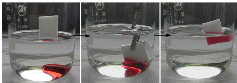
**Figure S5** Selective collection of underwater oils with superhydrophobic sponge.
