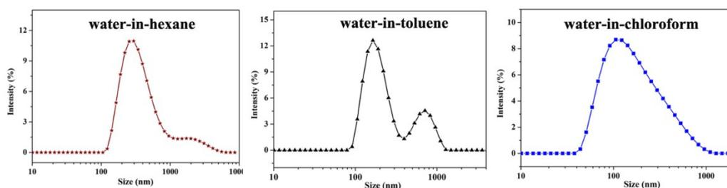
**Figure S10** Droplet size of (a) water-in-hexane emulsion, (b) water-in-toluene emulsion and (c) water-in-chloroform emulsion via DLS measurements.
