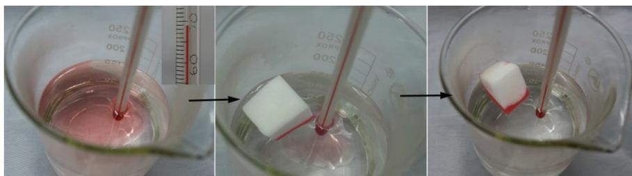
**Figure S7** Hexadecane can be successfully removed from hot water surface with prepared superhydrophobic sponge.
