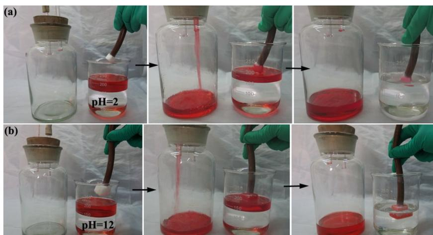
**Figure S8** The designed oil-collecting device using superhydrophobic sponges can
