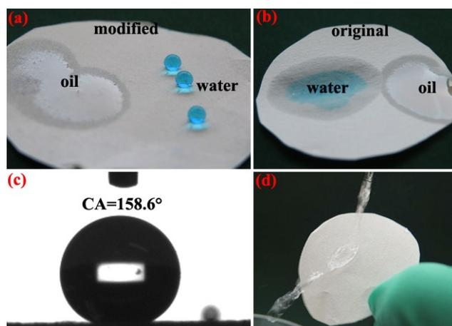
**Figure S9** (a, c)The prepared superhydrophobic filter paper shows a high contact angle of  $158.6^\circ$  and can only be selectively wetted by oil. (d)A jet of water could perfectly bounce off the surface. In contrast, both water and oil can wet the raw filter paper (b).
