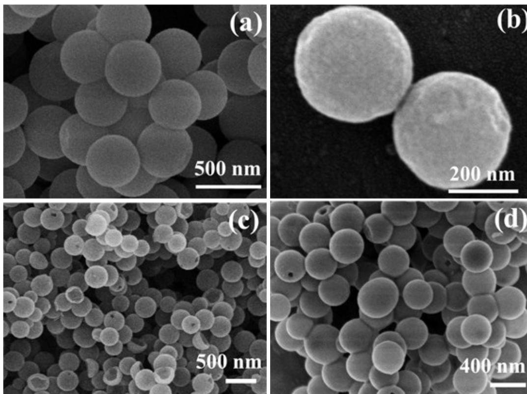
**Figure S1.** FESEM images of (a, b) SiO<sub>2</sub>@PDA spheres and (c, d) NHCS.
