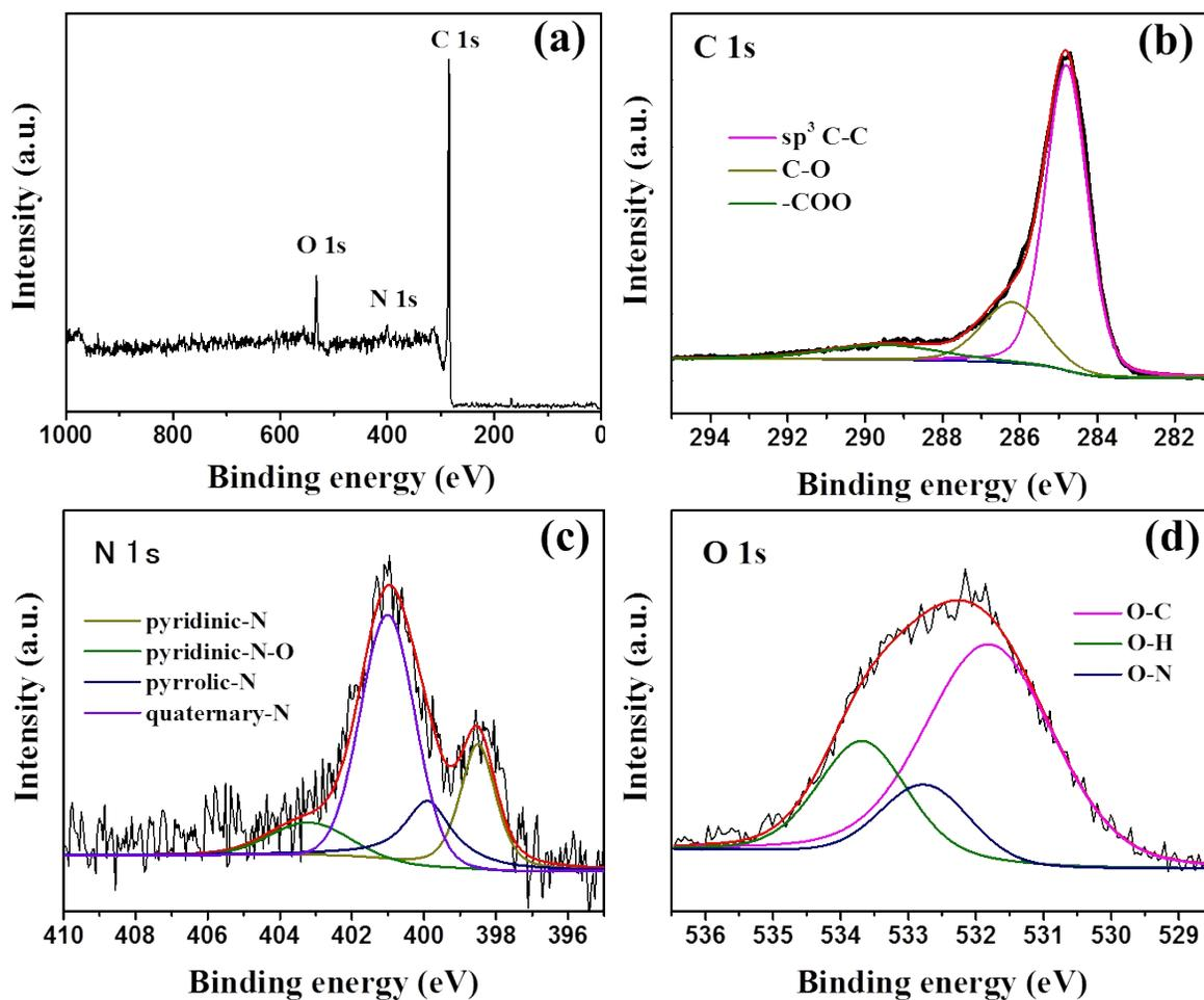
**Figure S2.** XPS spectra of the NHCS sample: (a) survey spectrum; (b) C 1s spectrum; (c) N 1s spectrum; (d) O 1s spectrum.
