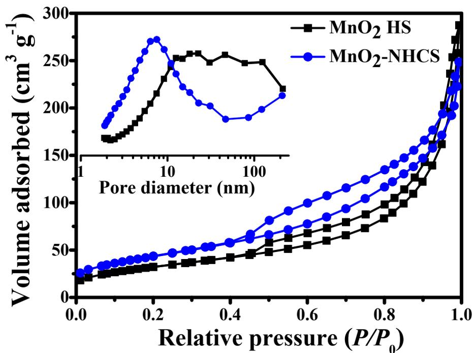
**Figure S5.** N<sub>2</sub> adsorption/desorption isotherms of MnO<sub>2</sub>-NHCS and MnO<sub>2</sub> HS, with the inset exhibiting the pore size distributions.
