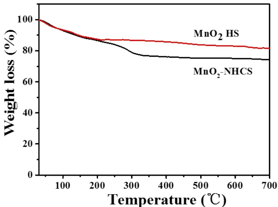
**Figure S4.** TGA curves of MnO<sub>2</sub>-NHCS and MnO<sub>2</sub> HS. This pyrolysis process was carried out in air at a heating rate of 10 °C min<sup>-1</sup>.
