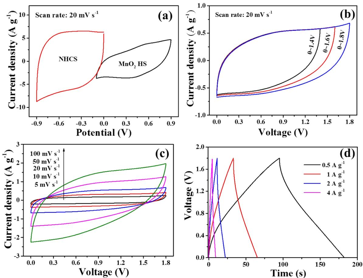
**Figure S8.** (a) CV curves of NHCS and MnO<sub>2</sub> HS measured in a three-electrode system at a scan rate of 20 mV s<sup>-1</sup>. Electrochemical performance of an asymmetric supercapacitor with MnO<sub>2</sub> HS as positive electrode and NHCS as negative electrode: (b) CV curves at different cell voltage, (c) CV curves at different scan rates with a cell voltage of 1.8 V, (d) GCD curves at various current densities. The electrolyte was 1 M Na<sub>2</sub>SO<sub>4</sub> aqueous solution.
