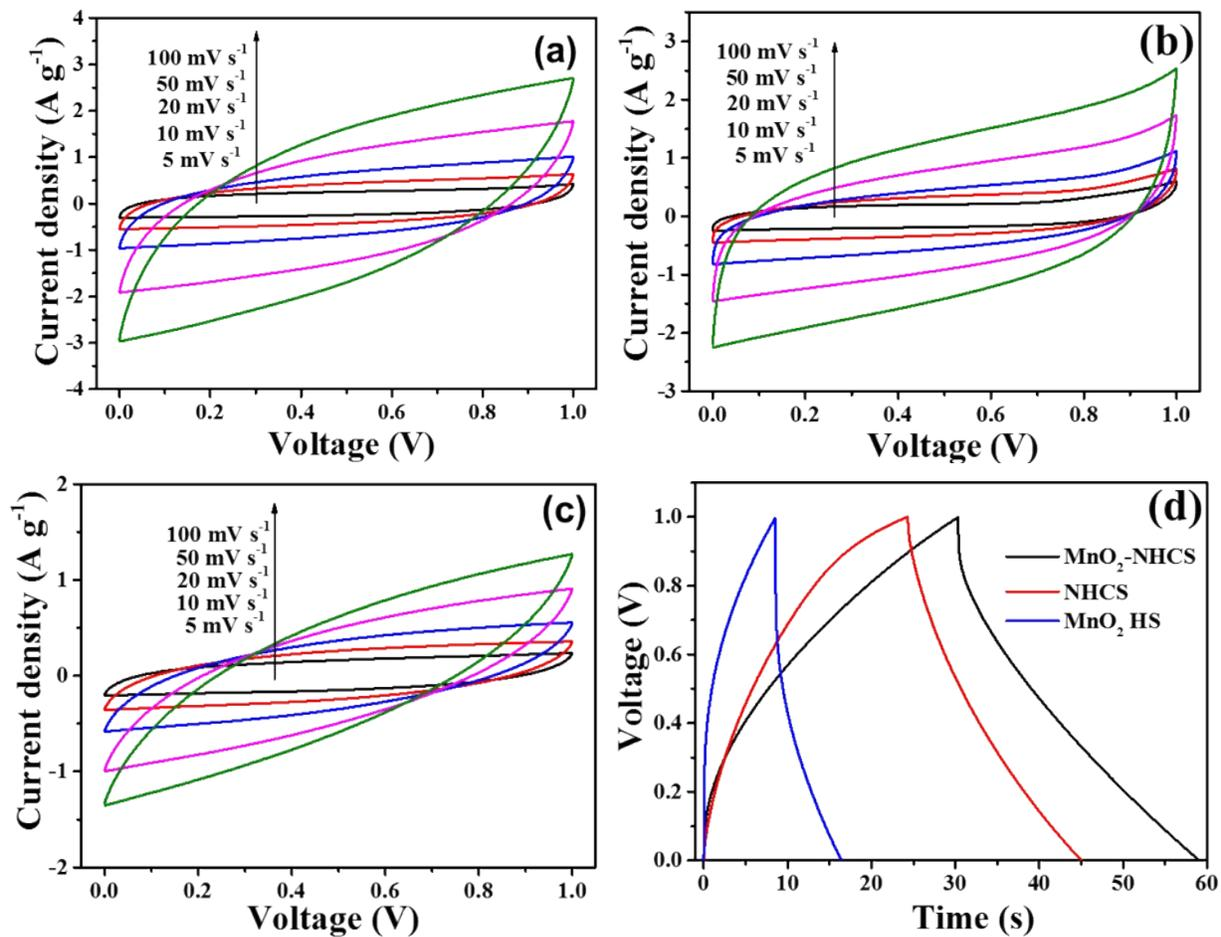
**Figure S9.** CV curves at different scan rates of the as-assembled symmetric supercapacitors (SC), (a) MnO<sub>2</sub>-NHCS//MnO<sub>2</sub>-NHCS, (b) NHCS//NHCS and (c) MnO<sub>2</sub> HS//MnO<sub>2</sub> HS. (d) GCD curves of MnO<sub>2</sub>-NHCS//MnO<sub>2</sub>-NHCS, NHCS//NHCS, and MnO<sub>2</sub> HS//MnO<sub>2</sub> HS at the current density of 1 A g<sup>-1</sup>.
