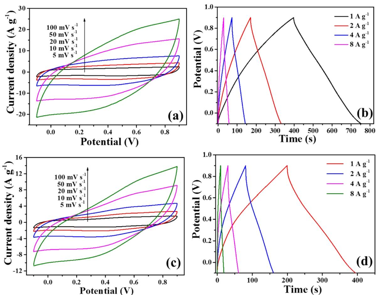
**Figure S7.** (a) CV curves at different scan rates and (b) GCD curves at various current densities of MnO<sub>2</sub>-NHCS composite. (c) CV curves at different scan rates and (d) GCD curves at various current densities of MnO<sub>2</sub> HS. These curves were measured in a three-electrode system in 1 M Na<sub>2</sub>SO<sub>4</sub> aqueous solution.
