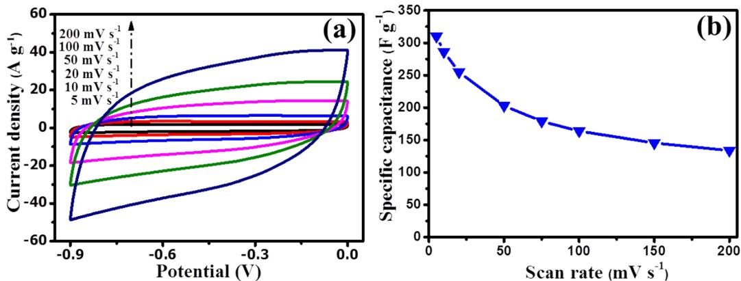
**Figure S6.** CV curves (a) and specific capacitances at different scan rates (b) of NHCS.
