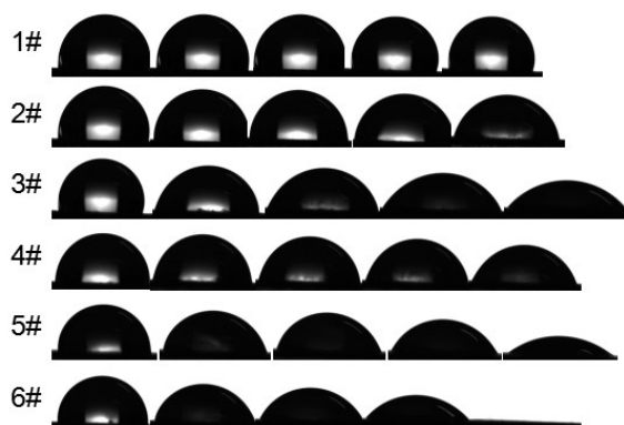
Fig. S4. The corresponding digital photos of the time-dependent water contact angle for DA-based TFC membrane top surface
