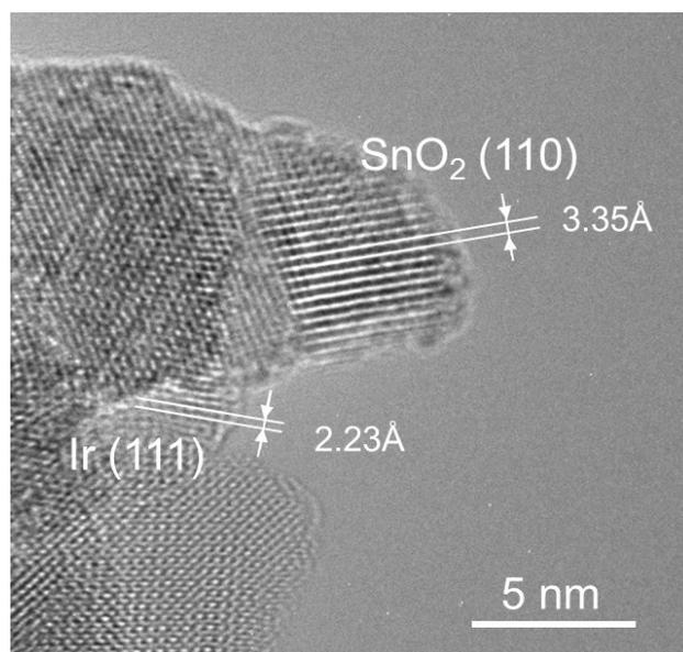
**Fig. S4** HRTEM image of Ir/SnO<sub>2</sub>:Sb-mod-V after the electrochemical oxidation (EC) protocol.
