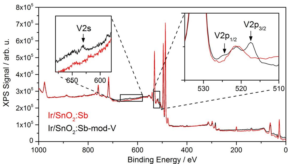
**Fig. S1** XPS survey spectra of Ir/SnO<sub>2</sub>:Sb-mod-V and Ir/SnO<sub>2</sub>:Sb demonstrating that V2p and V2s peaks were detected in Ir/SnO<sub>2</sub>:Sb-mod-V but not in Ir/SnO<sub>2</sub>:Sb.
