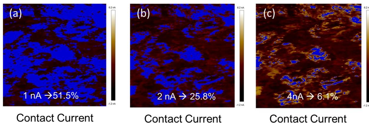
**Fig. S5** Contact current of Ir/SnO<sub>2</sub>:Sb-mod-V with different thresholds. The conductive area is marked in blue: (a) 1 nA; (b) 2 nA and (c) 4 nA.
