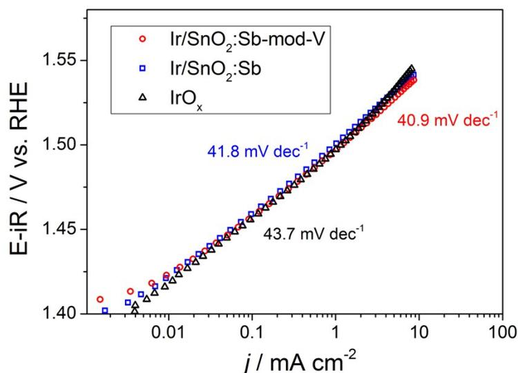
**Fig. S9** Tafel slope determination of Ir/SnO<sub>2</sub>:Sb-mod-V, Ir/SnO<sub>2</sub>:Sb and IrO<sub>x</sub>.
