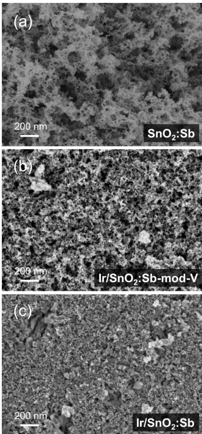
**Fig. S2** SEM images showing morphology of (a) SnO<sub>2</sub>:Sb aerogel, (b) Ir/SnO<sub>2</sub>:Sb-mod-V and (c) Ir/SnO<sub>2</sub>:Sb at high resolution.
