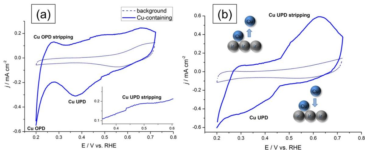
**Fig. S11** Cu-UPD measurements of (a) Ir/SnO<sub>2</sub>:Sb and (b) unsupported IrO<sub>x</sub>.
