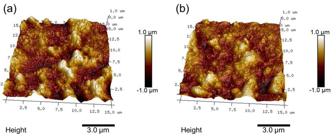
**Fig. S6** 3D topography (15 μm) of (a) Ir/SnO<sub>2</sub>:Sb-mod-V and (b) Ir/SnO<sub>2</sub>:Sb measured with AFM.
