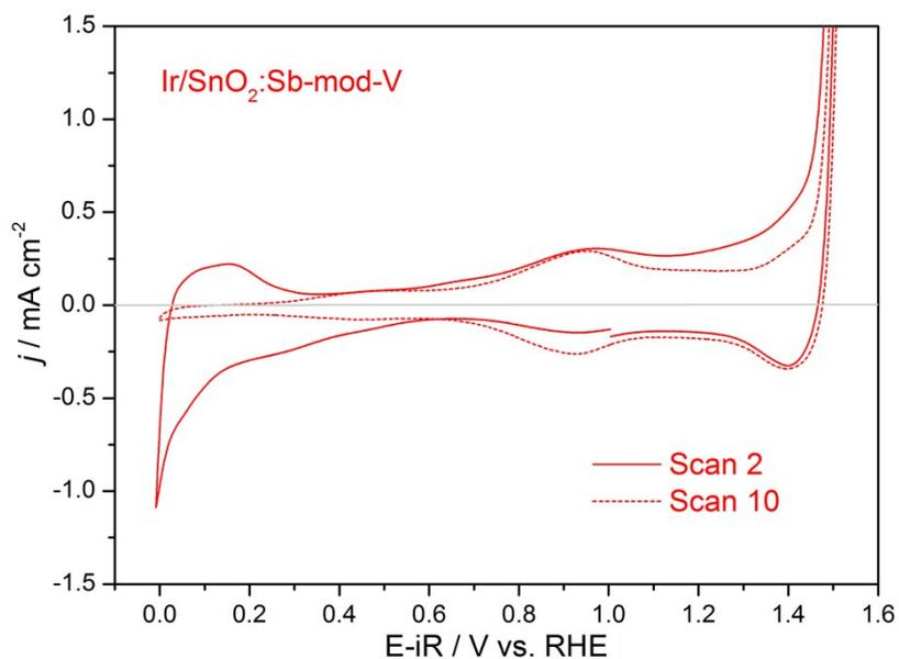
**Fig. S7** Fingerprint CV profiles (cycle 2 and cycle 10) of the Ir/SnO<sub>2</sub>:Sb-mod-V sample during the electrochemical oxidation (EC) protocol.
