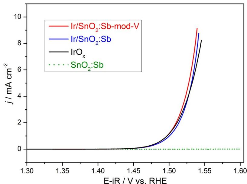
**Fig. S8** Geometric OER activity comparison among Ir/SnO<sub>2</sub>:Sb-mod-V, Ir/SnO<sub>2</sub>:Sb, unsupported IrO<sub>x</sub> and pure SnO<sub>2</sub>:Sb aerogel (N<sub>2</sub>-saturated 0.05 M H<sub>2</sub>SO<sub>4</sub>, 5 mV s<sup>-1</sup>, 1600 rpm, 25 °C). Ir loading on GC-RDE: 17 μg cm<sup>-2</sup> for Ir/SnO<sub>2</sub>:Sb-mod-V and Ir/SnO<sub>2</sub>:Sb, 60 μg for unsupported IrO<sub>x</sub>.
