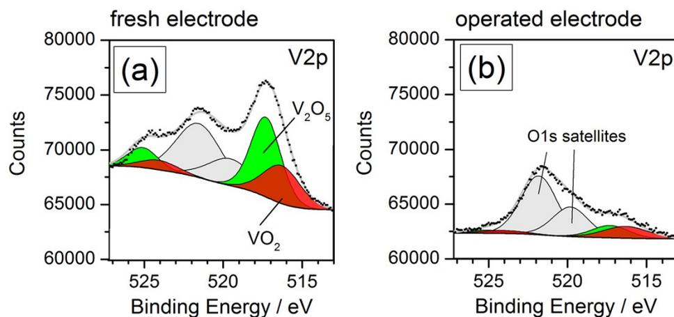
**Fig. S10** XPS analysis: detailed V2p spectra of Ir/SnO<sub>2</sub>:Sb-mod-V (a) before and (b) after electrochemical characterization. The deconvoluted peaks of O1s satellites (grey), VO<sub>2</sub> (red) and V<sub>2</sub>O<sub>5</sub> (green) are shown.
