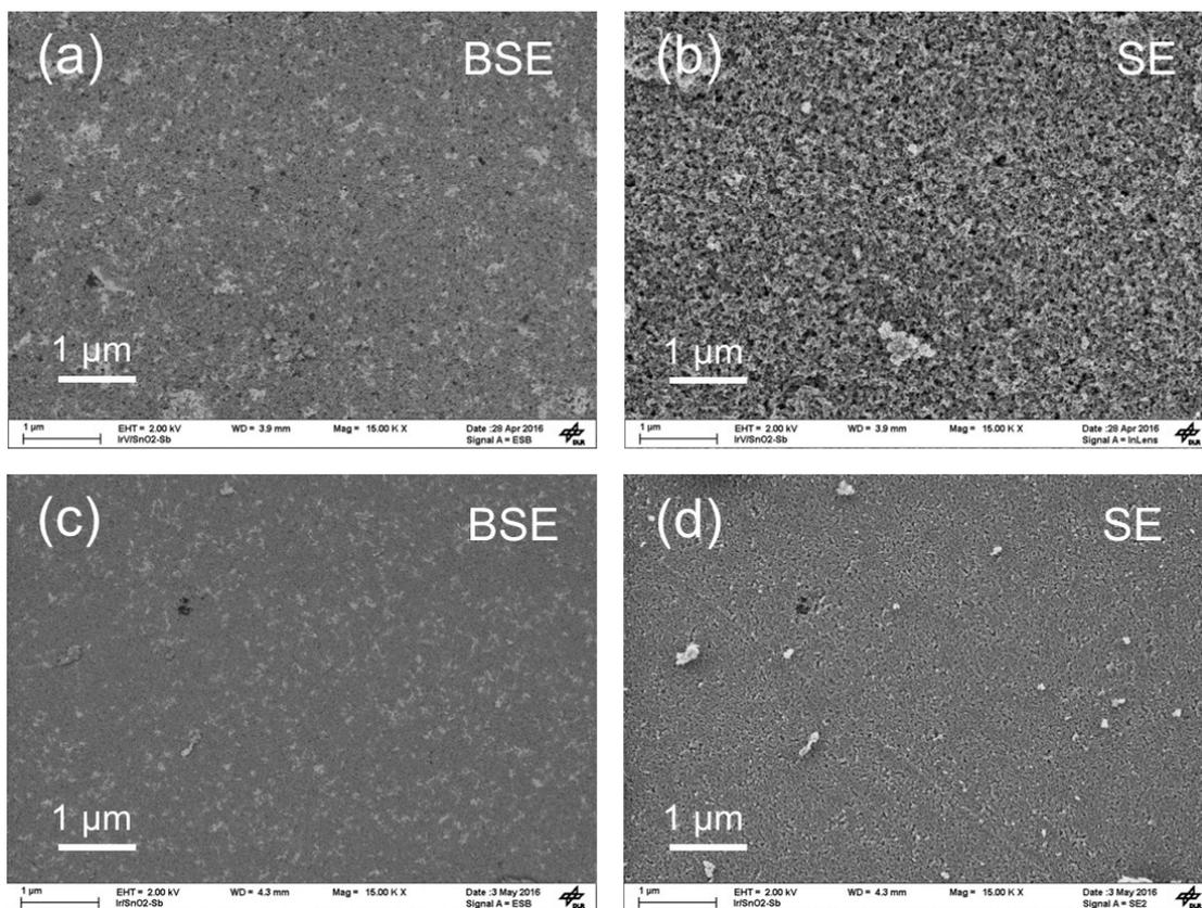
**Fig. S3** SEM images of (a, b) Ir/SnO<sub>2</sub>:Sb-mod-V and (c, d) Ir/SnO<sub>2</sub>:Sb: panel (a) and (c) were analyzed by back-scattered electrons for the elemental distribution; panel (b) and (d) were analyzed by secondary electrons for morphology observations.
