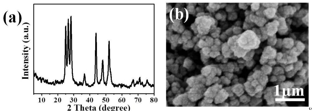
Fig. S1 (a) XRD pattern and (b) FESEM image of CdS-P
