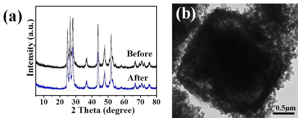
Fig. S5 (a) XRD patterns of CdS-YS before and after the photocatalytic reaction and (b) TEM image of CdS-YS after 4 cycles
