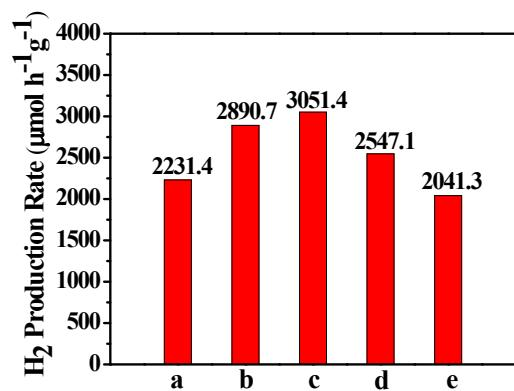
Fig. S3 Effect of sacrificial donor concentration on hydrogen evolution rate: (a)
