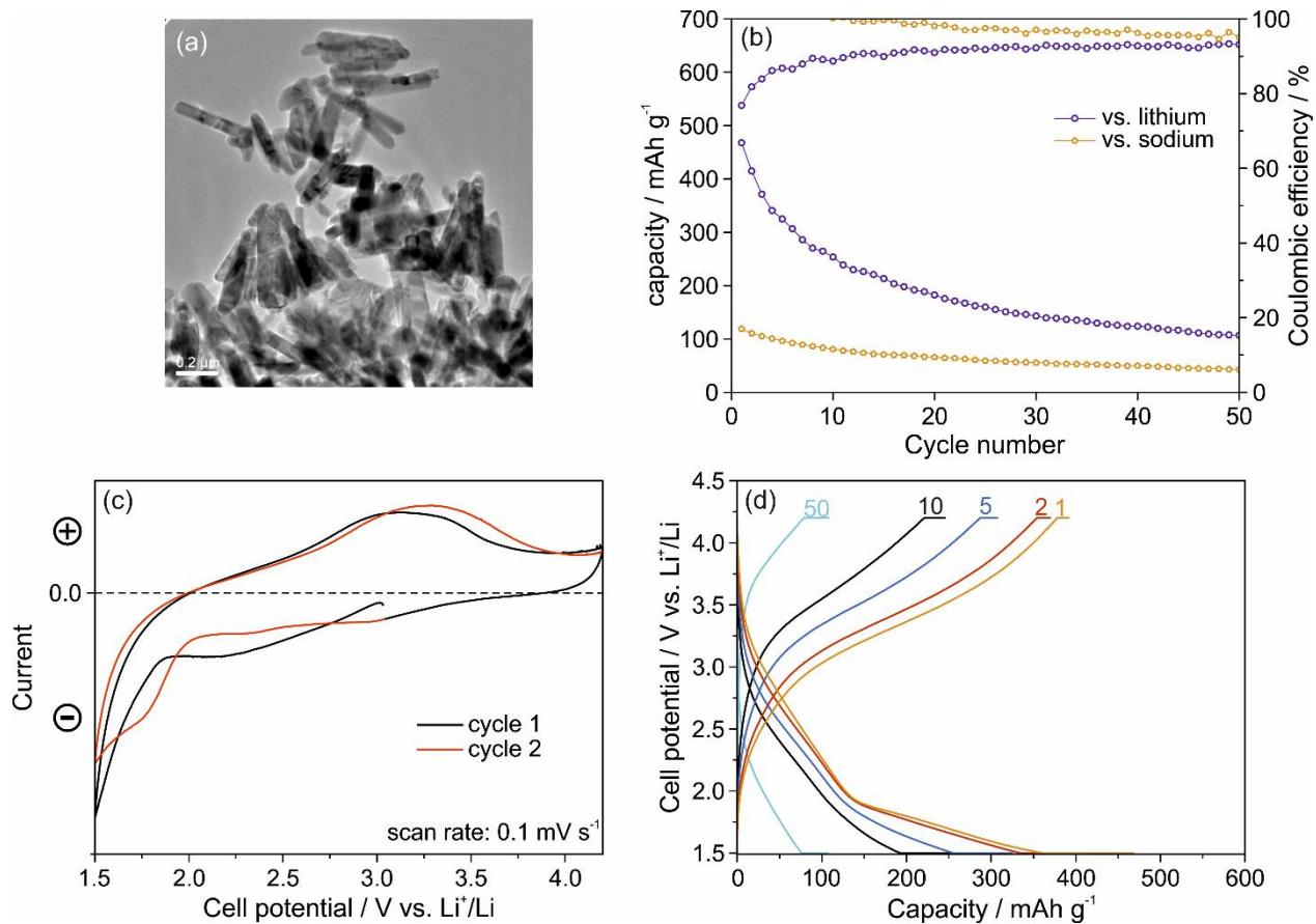
**Fig. S9** Electrochemical results obtained with  $\text{FeF}_2$  as active material. (a) TEM image of  $\text{FeF}_2$ ; (b) Galvanostatic cycling towards lithium (1.5-4.2 V) and sodium (1.2-4.0 V) with a current rate of 100 mAh/g; (c) Cycling voltammetry between 1.5 V and 4.2 V versus lithium. (d) Voltage - capacity plot towards lithium.
