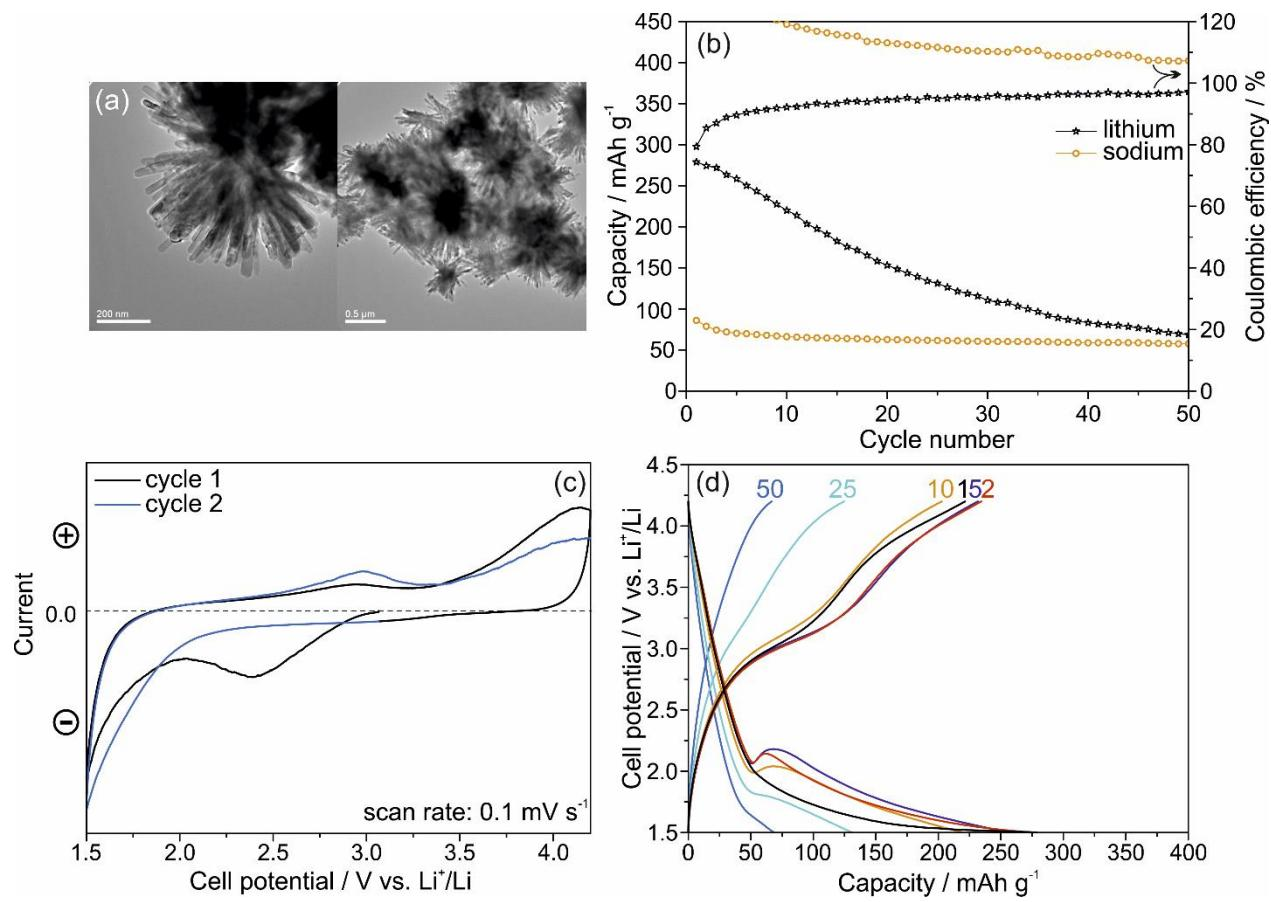
**Fig. S11** Electrochemical results obtained with  $\text{CoF}_2$  as active material. (a) TEM images of  $\text{CoF}_2$  (b) Galvanostatic cycling towards lithium (1.5-4.2 V) and sodium (1.2-4.0 V) with a current rate of 100  $\text{mAh/g}$  (c) Cyclic voltammetry between 1.5 V and 4.2 V. (d) Voltage - capacity plot towards lithium.
