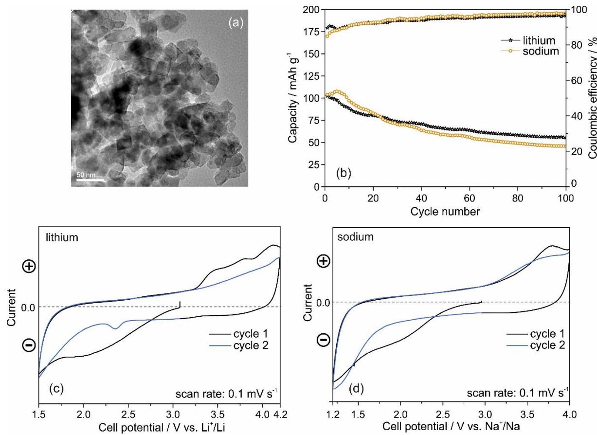
**Fig. S10** Electrochemical results and TEM image from  $\text{MnF}_2$ . (a) TEM image of  $\text{MnF}_2$ . (b) Galvanostatic measurements measured against lithium (1.5–4.2 V) and sodium (1.2–4.0 V) with a current rate of 100 mA/g. (c) Cycling voltammetry towards lithium between 1.5 V and 4.2 V. (d) Cyclic voltammetry towards sodium between 1.2 V and 4.0 V.
