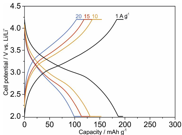
**Fig. S16** Voltage-capacity plot of galvanostatic measurements in the voltage window 2.0 – 4.2 V towards lithium. Different current speeds ( $1, 10, 15, 20 \text{ A g}^{-1}$ ) were applied. The 5<sup>th</sup> cycle is presented for each measurement.
