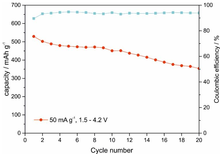
**Fig. S13** Galvanostatic cycling of  $\text{FeF}_3$  within 1.5-4.2 V with a current density of  $50 \text{ mA/g}$ . In this half-cell a different cathode composition was used but with the same method of preparation. The cathode material has a ratio of 40%  $\text{FeF}_3$ , 50 % CB, 10 % pVdF. The observed coulombic efficiency is lower as well as the cycling retention compared to the intercalation reaction only between 2-4.2 V.
