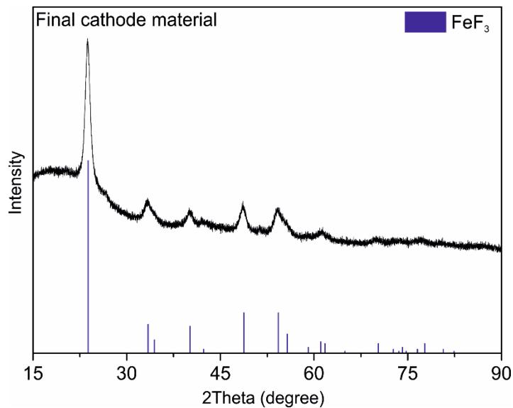
**Fig. S12** Powder XRD pattern of the cathode material ( $\text{FeF}_3/\text{CB}/\text{GO}$ ) after wet ball milling. No sign of reduction of  $\text{FeF}_3$  (PDF 033-0647) is observable.
