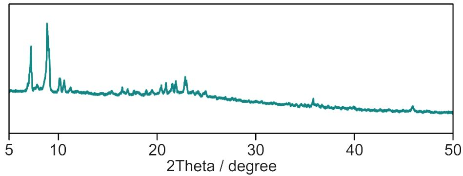
**Fig. S1** Powder XRD pattern of “Co(TFA)<sub>2</sub>”.
