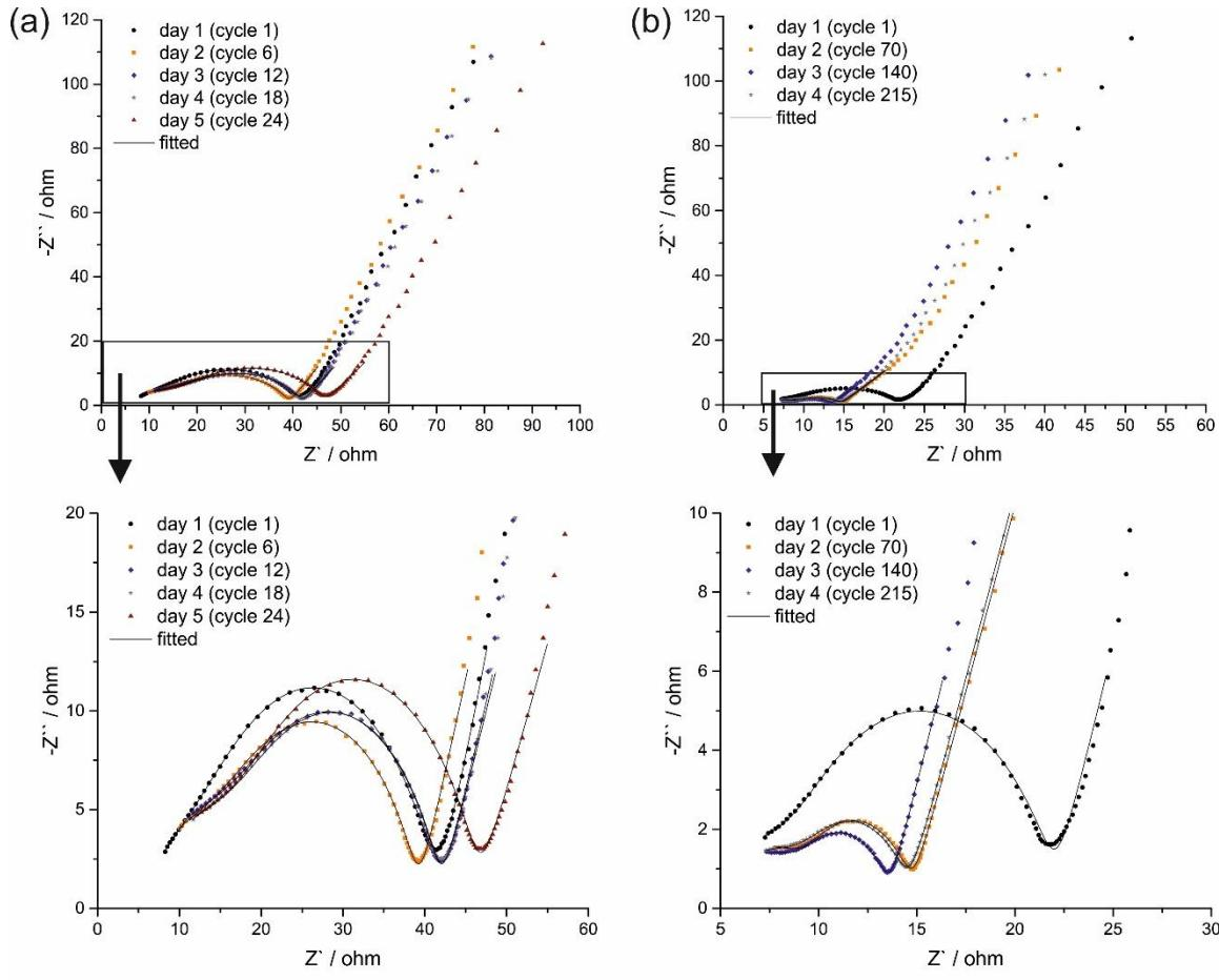
**Fig. S14** EIS measurements during the galvanostatic cycling of two Li-ion half-cells at current densities of (a)  $0.1 \text{ A g}^{-1}$  and (b)  $1 \text{ A g}^{-1}$ . Every day an EIS measurement was performed. (c) Equivalent electrical circuit.
