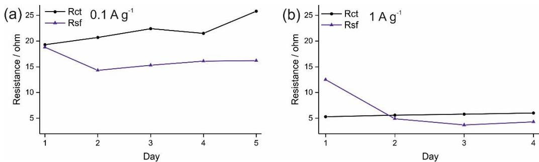
**Figure S15.** Evolution of the  $R_{ct}$  and  $R_{sf}$  values over several days of cycling at (a)  $0.1 \text{ A g}^{-1}$  and (b)  $1 \text{ A g}^{-1}$  in the voltage range of 2-4.2 V.
