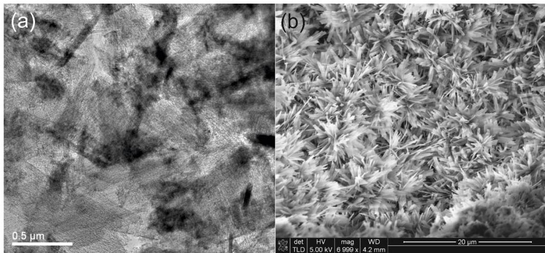
**Fig. S8** Low resolution images (a) TEM image of  $\text{FeF}_3$ ; (b) SEM image of  $\text{FeF}_3$
