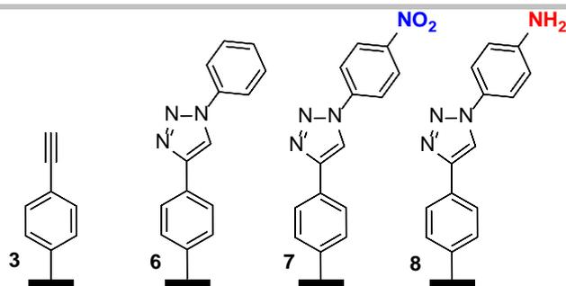
**Figure 9.** Representative chemical structures of functionalized fibers, after electrochemical grafting (3) and click reaction to give phenyl (6), nitro (7), and aniline (8) terminated samples.
