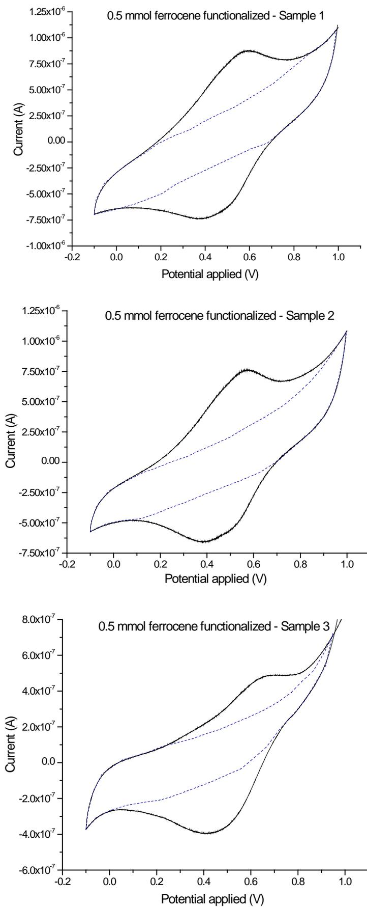
Figure 5. 0.5 mM ferrocene redox curve scanned at  $0.01 \text{ V s}^{-1}$  in  $0.1 \text{ M TBAPF}_6$  in MeCN.
