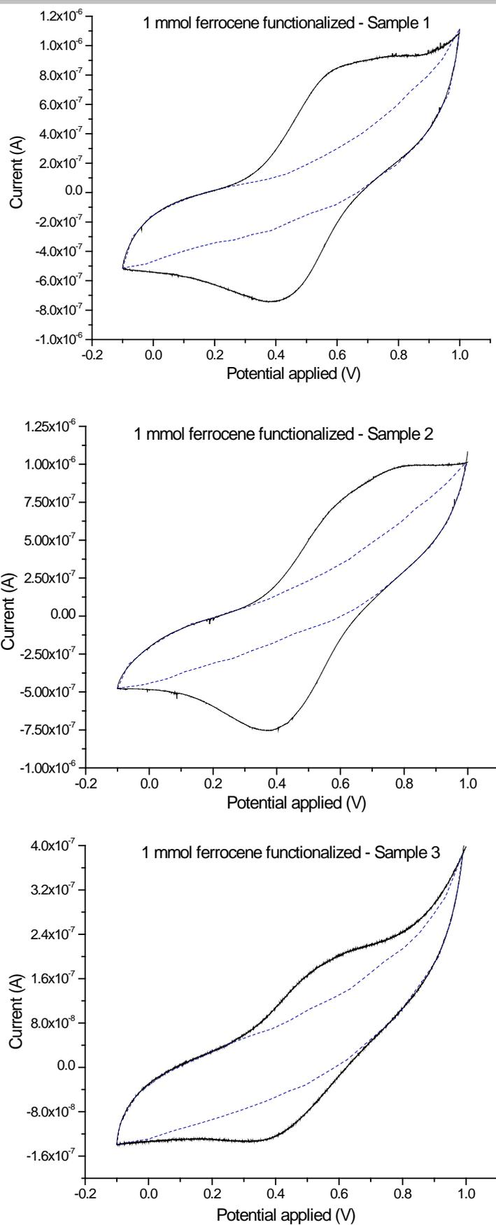
**Figure 4.** 1 mM ferrocene redox curve scanned at 0.01 V s<sup>-1</sup> in 0.1 M TBAPF<sub>6</sub> in MeCN.
