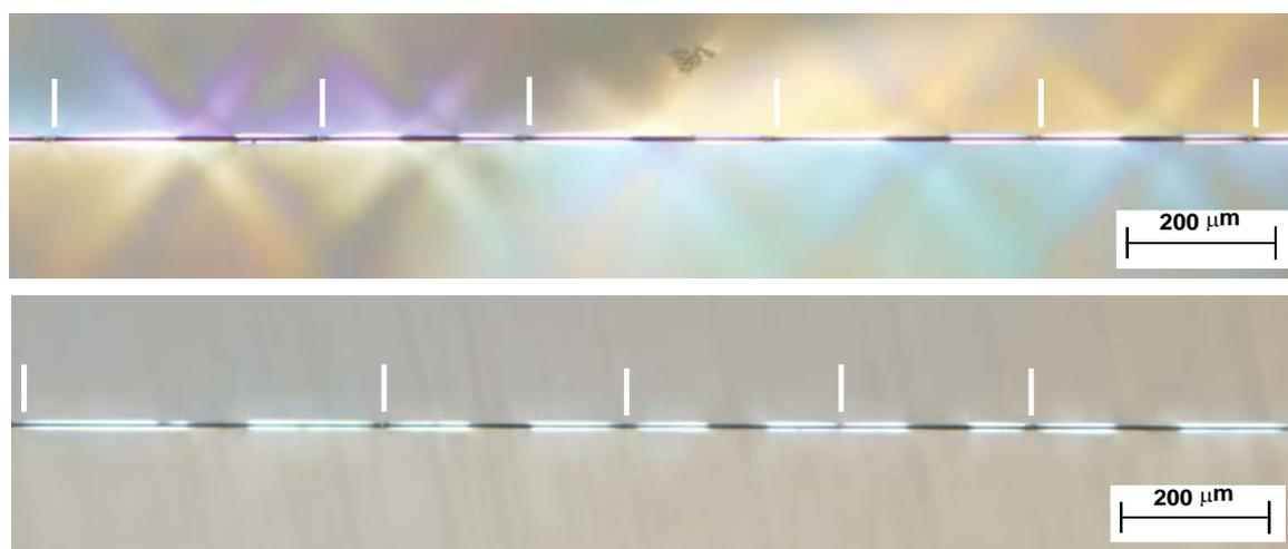
Figure 16. Representative optical microscope images of SFFT samples **8a** (top) and **11** fiber fragments denoted using vertical white lines. Average fragment size calculated for samples are: (**8a**) 397 μm, (**11**) 380 μm.
