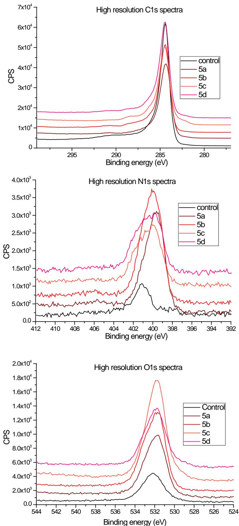
**Figure 2.** High resolution C1s, N1s, and O1s XPS spectra for treated samples
