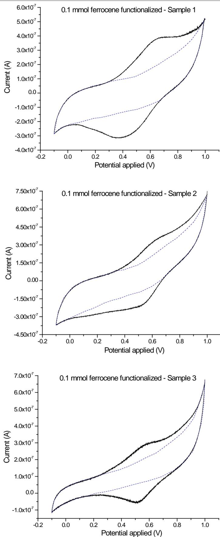
Figure 6. 0.1 mM ferrocene redox curve scanned at  $0.01 \text{ V s}^{-1}$  in 0.1 M TBAPF<sub>6</sub> in MeCN.
