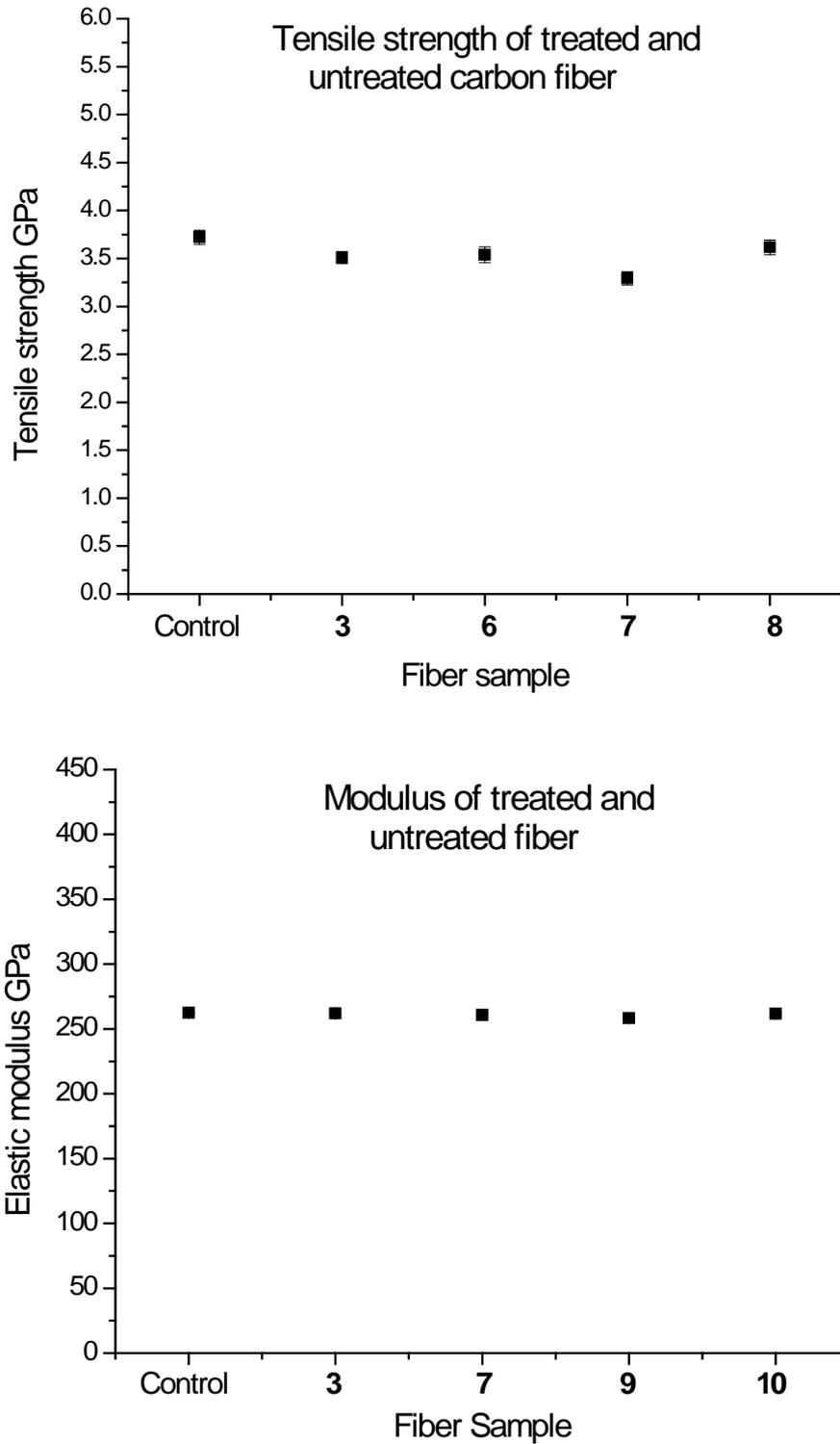
**Figure 12.** Tensile strength and modulus measured using a Favimat tensile tester (75 filaments per sample). Standard error presented (may be too small to see).
