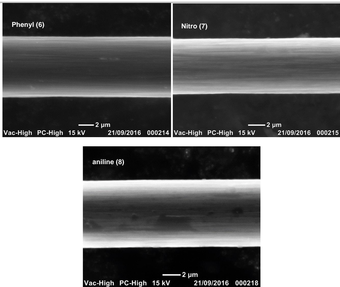
**Figure 11.** Electron micrographs of control and treated fibers 3, 6, 7 and 8.
