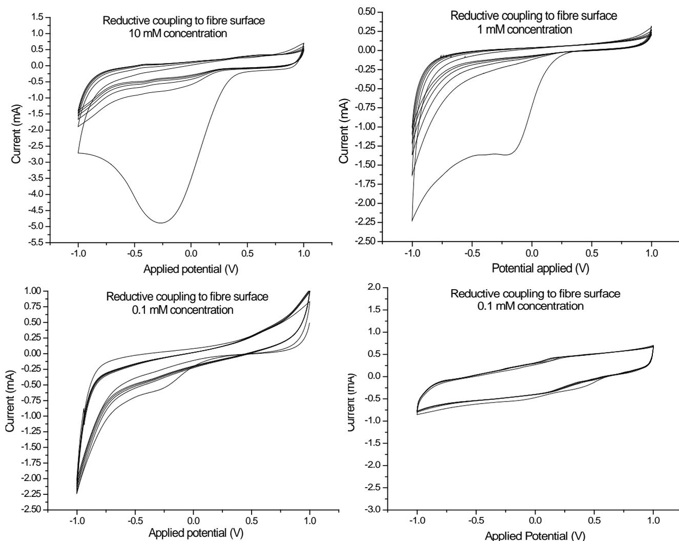
Figure 1. Reductive coupling of diazoalkyne 2 to carbon fiber probe at a 10, 1, 0.5 and 0.1 mM concentration in 0.1 M TBAPF<sub>6</sub> in MeCN.
