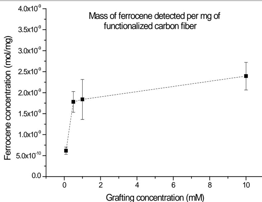
Figure 8. Average number of moles of surface bound ferrocene per mg of CF.
