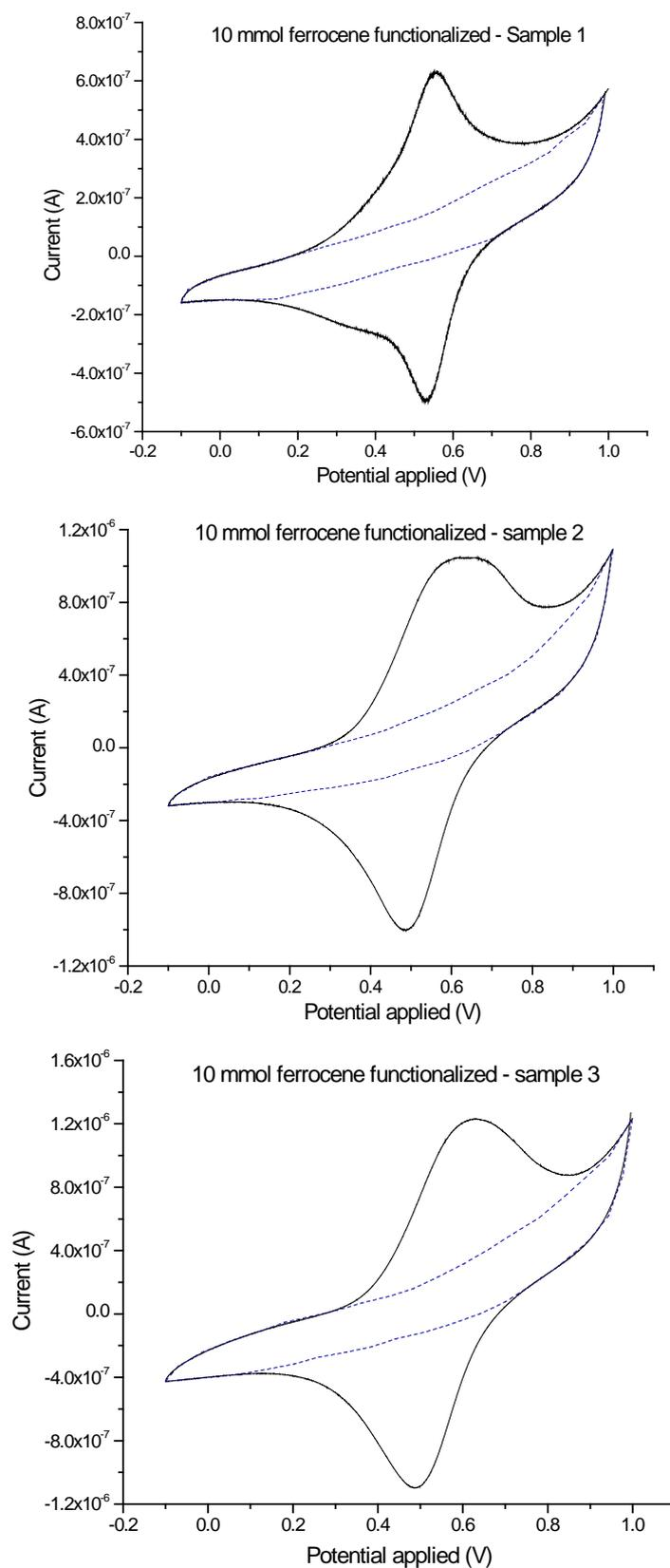
Figure 3. 10 mM ferrocene redox curve scanned at 0.01 V s<sup>-1</sup> in 0.1 M TBA PF<sub>6</sub> in MeCN.
