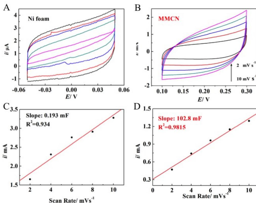
**Figure S9.** CV curves measured at different scan rates from 2 mV/s to 10 mV/s of (A) Ni foam, (B) MMCN, current densities recorded at 0.2 V plotted vs. scan rates of (C) Ni foam and (D) MMCN.
