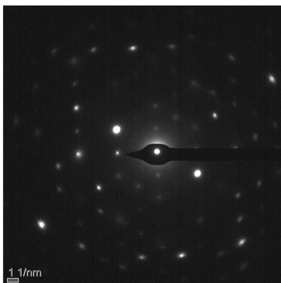
**Figure S5.** SAED pattern of electrodeposited MnO<sub>2</sub> shell-NSs.
