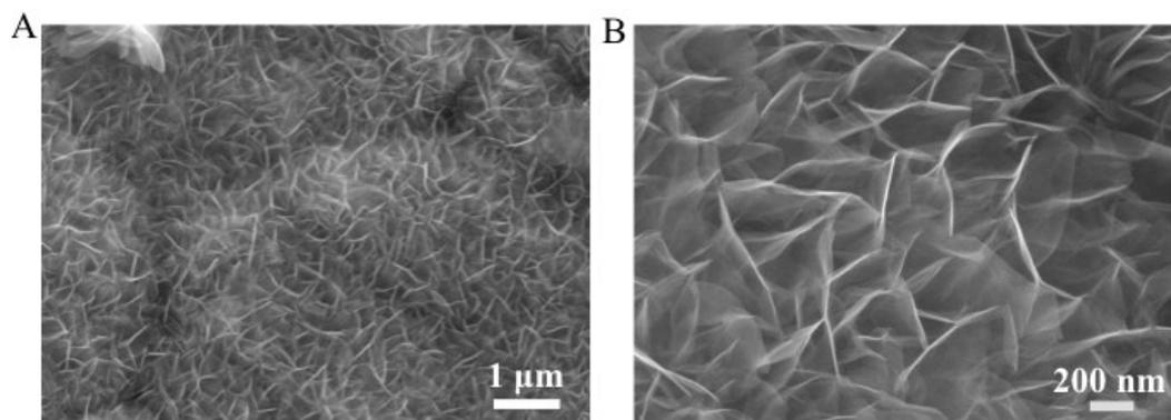
**Figure S8.** SEM images of MnO<sub>2</sub>/Ni foam electrode at different magnifications.
