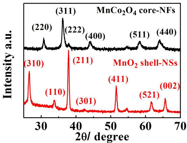
**Figure S4.** XRD patterns of MnO<sub>2</sub> Shell-NSs electrodeposited on ITO glass (red) and MnCo<sub>2</sub>O<sub>4</sub> core-NFs (black) .
