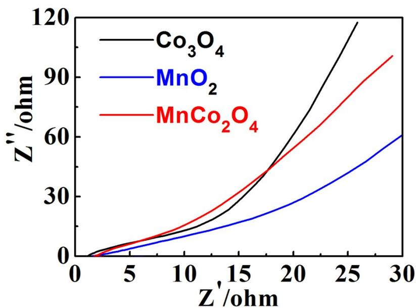
**Figure S13.** Nyquist plots  $\text{Co}_3\text{O}_4/\text{Ni}$  foam,  $\text{MnCo}_2\text{O}_4/\text{Ni}$  foam and MMCN electrodes.
