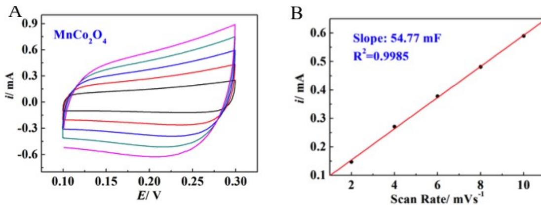
**Figure S10.** CV curves of MnCo<sub>2</sub>O<sub>4</sub>/Ni foam electrode measured at different scan rates from 2 mV/s to 10 mV/s and (B) current densities at 0.2 V plotted vs. scan rates.
