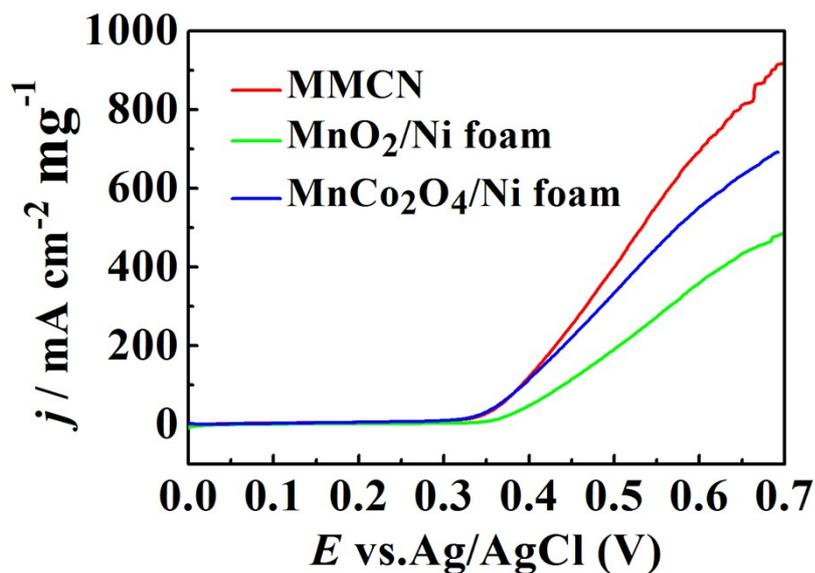
**Figure S12.** Absolute UOR polarization curves of MMCN,  $\text{MnCo}_2\text{O}_4/\text{Ni}$  foam and  $\text{MnO}_2/\text{Ni}$  foam electrodes in 0.5 urea/1 M KOH at a scan rate of  $5 \text{ mV s}^{-1}$ . The current is normalized by catalyst mass loading and subtracted off the current from OER.
