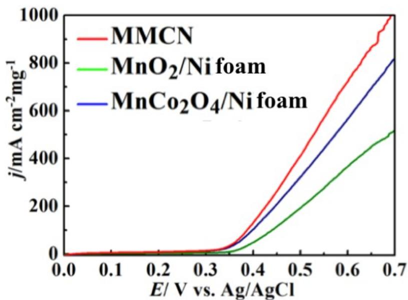
**Figure S7.** UOR polarization curves of MMCN, MnCo<sub>2</sub>O<sub>4</sub>/Ni foam and MnO<sub>2</sub>/Ni foam electrodes in 0.5 urea/1 M KOH at a scan rate of 5 mV s<sup>-1</sup>.
