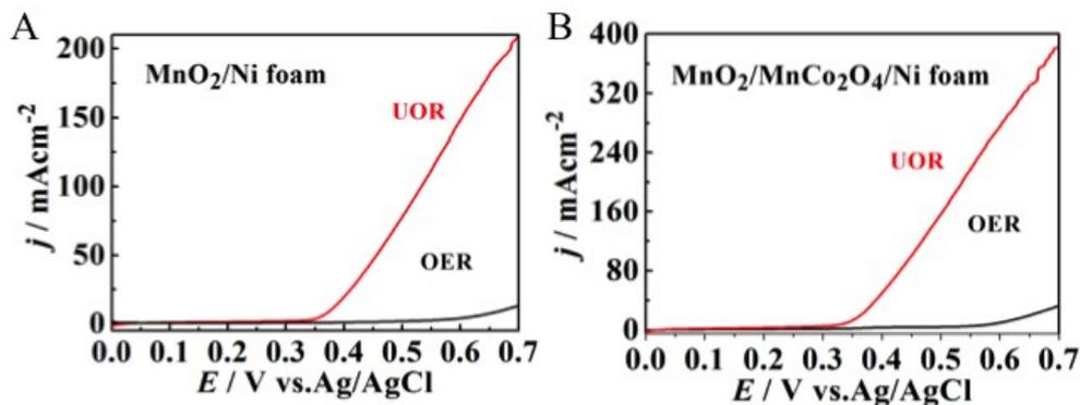
**Figure S14.** Comparison of UOR and OER polarization curves of (A)  $\text{MnO}_2/\text{Ni}$  foam and (B)  $\text{MnCo}_2\text{O}_4$  electrodes.
