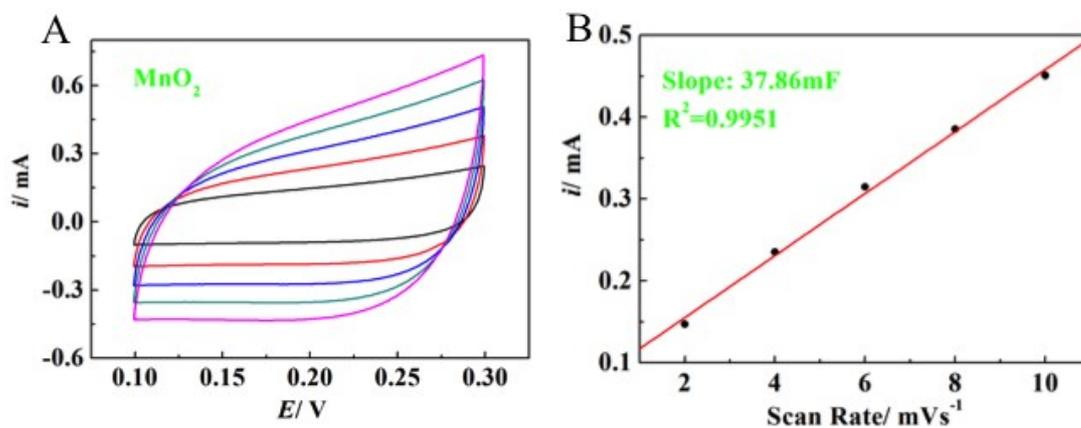
**Figure S11.** CV curves of MnO<sub>2</sub>/Ni foam electrode measured at different scan rates from 2 mV/s to 10 mV/s and (B) current densities at 0.2 V plotted vs. scan rates.
