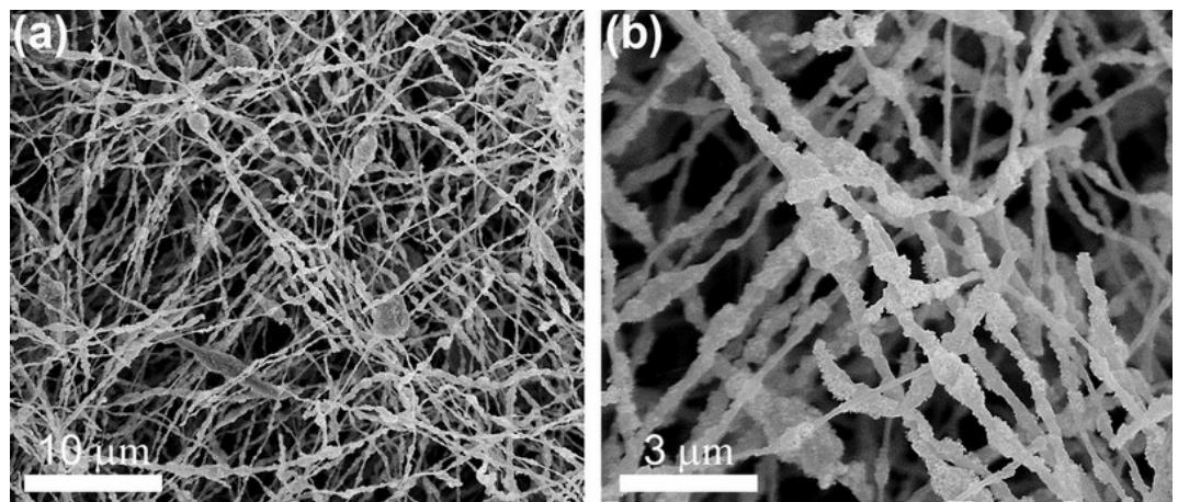
**Fig. S1** SEM images of SiO<sub>2</sub>/G/NPCFs with SiO<sub>2</sub> concentration of 30 mg mL<sup>-1</sup>.
