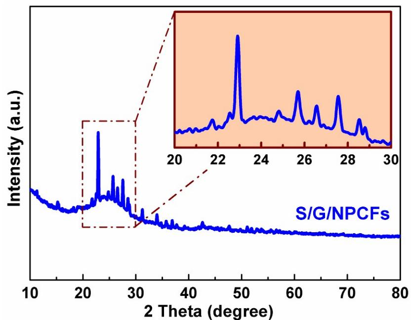
**Fig. S2** XRD diffraction pattern of S/G/NPCFs (inset: partial enlarge pattern of S/G/NPCFs).
