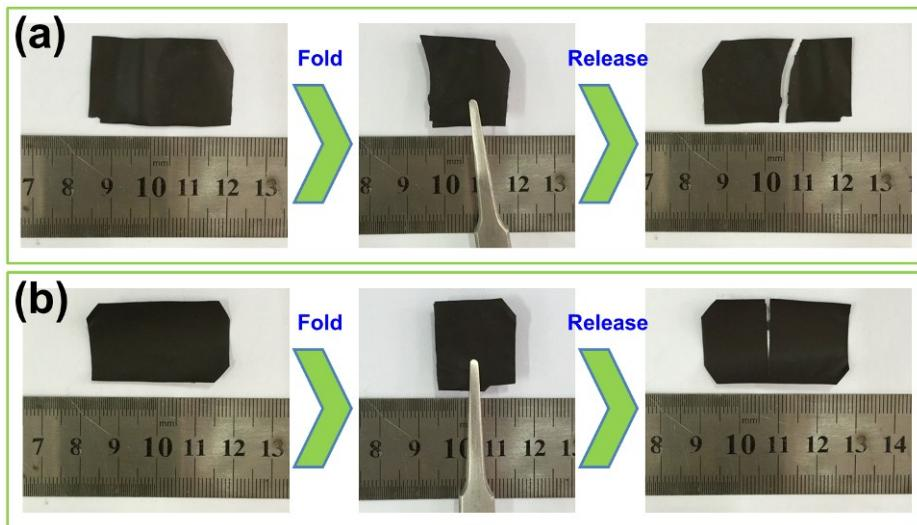
**Fig. S6** Mechanical properties of sulfur composite film without adding  $\text{SiO}_2$ . a) Photographs of S/NCFs composite film and b) S/G/NCFs composite film.
