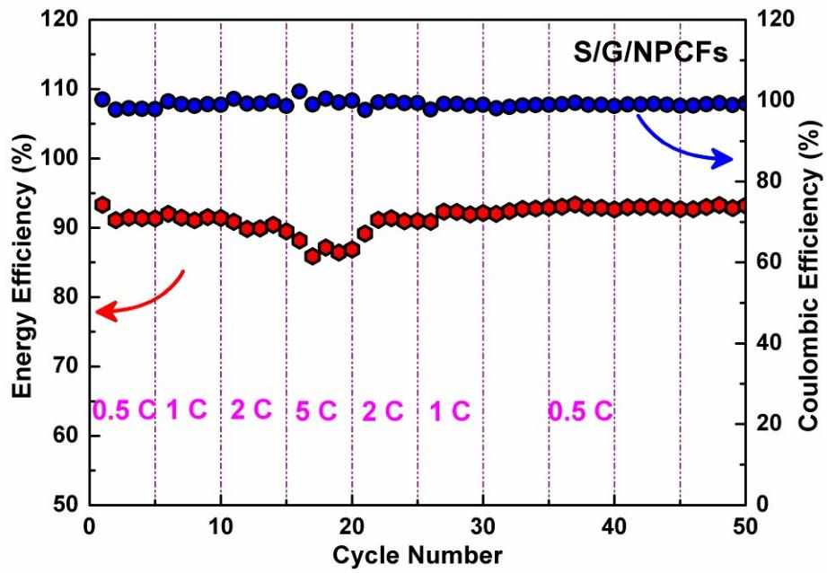
**Fig. S12** Energy efficiency and Coulombic efficiency of S/G/NPCFs electrode at different current densities.
