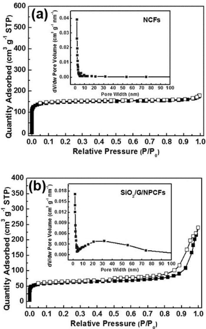
**Fig. S5** a) Nitrogen adsorption-desorption isotherms of NCFs and b) SiO<sub>2</sub>/G/NPCFs (insets are the corresponding pore size distribution curves).
