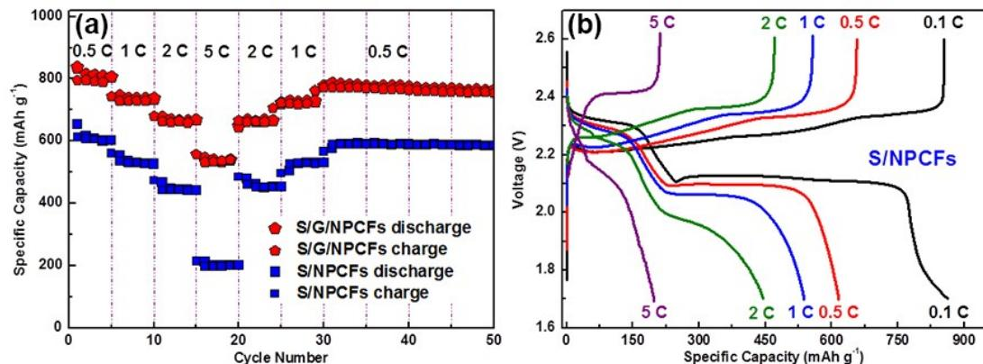
**Fig. S13** a) Rate capabilities of S/NPCFs and S/G/NPCFs electrode; b) Typical discharge-charge curves of S/NPCFs electrodes recorded at current rates of 0.1 C, 0.5 C, 1 C, 2 C, and 5 C.
