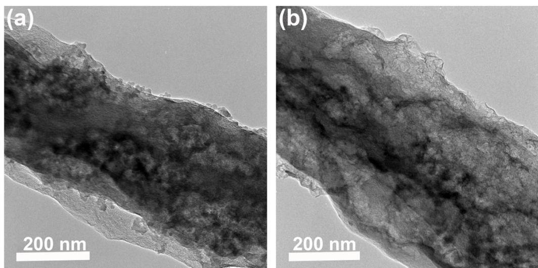
**Fig. S8** TEM images of a)  $\text{SiO}_2/\text{G}/\text{NPCFs}$ , b)  $\text{G}/\text{NPCFs}$ ;
