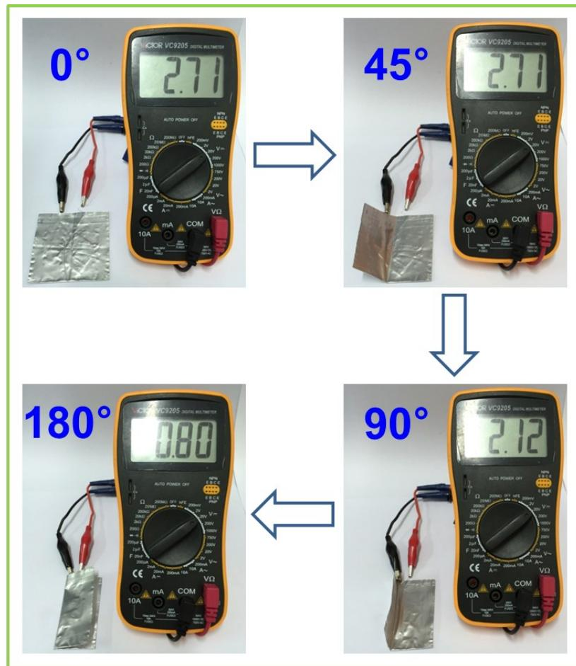
**Fig. S14** The open-circuit voltage of a flexible battery using S/G/NCFs electrode as cathode at different bending angles.
