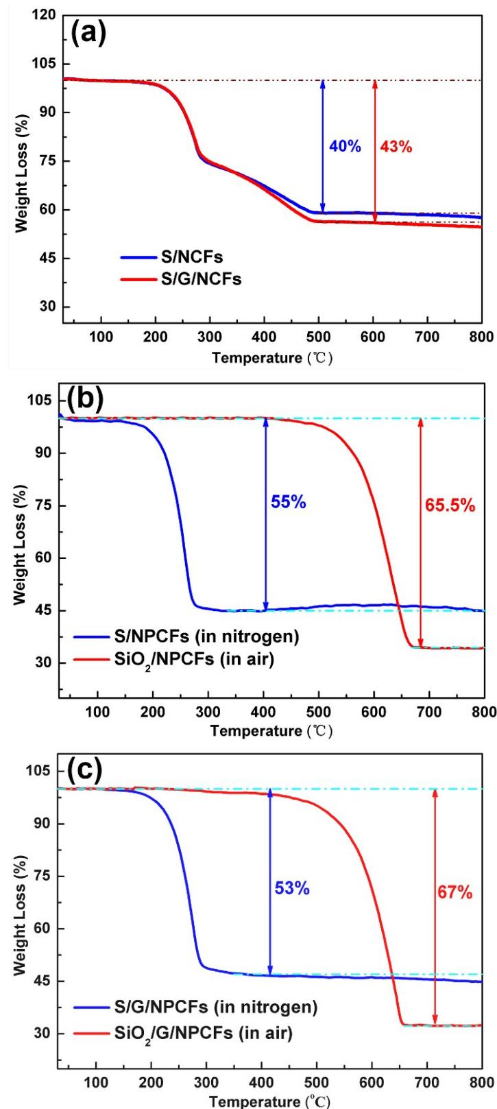
**Fig. S7** a) TG curves of S/NCFs (in nitrogen) and S/G/NCFs (in nitrogen); b) TG curves of SiO<sub>2</sub>/NPCFs (in air) and S/NPCFs (in nitrogen); c) TG curves of SiO<sub>2</sub>/G/NPCFs (in air) and S/G/NPCFs (in nitrogen).
