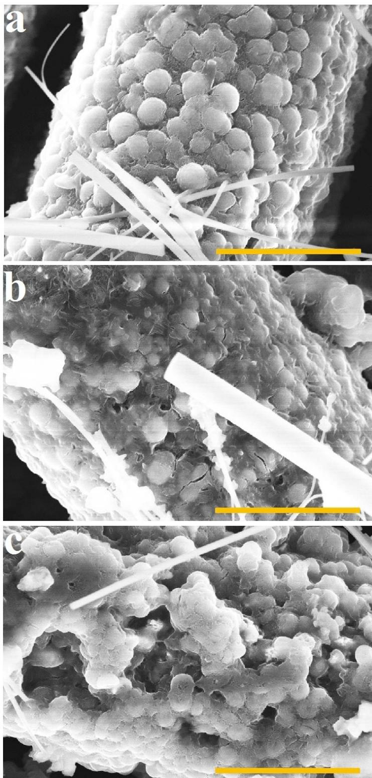
**Figure S3.** SEM images of Mo<sub>2</sub>C@CC electrodes after discharged to 2.2 V under different current density. a, 200 mA g<sup>-1</sup>; b, 500 mA g<sup>-1</sup>; and c, 1000 mA g<sup>-1</sup>, respectively. All bar is 5.0 μm
