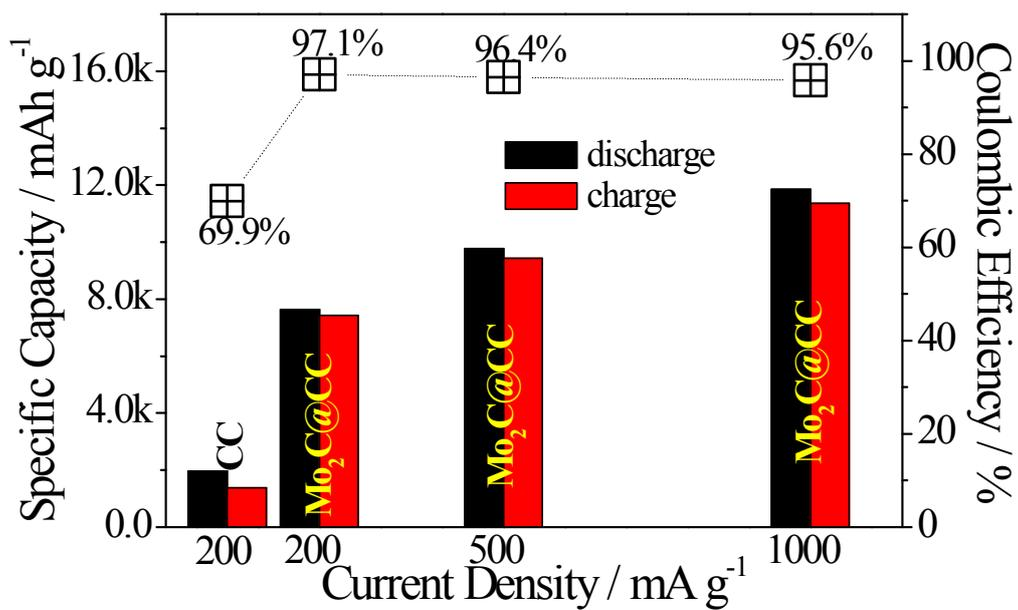
**Figure S4.** Discharge/charge specific capacity and corresponding coulombic efficiency at different current densities.
