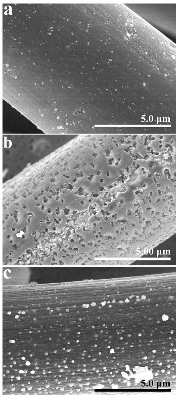
**Figure S2.** SEM images of Mo<sub>2</sub>C@CC electrodes impregnated in different concentration (NH<sub>4</sub>)<sub>6</sub>Mo<sub>7</sub>O<sub>24</sub>·4H<sub>2</sub>O solution: 0.005 M (a), 0.015 M (b), 0.05 M (c).
