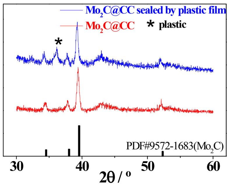
**Figure S7.** XRD patterns of Mo<sub>2</sub>C@CC with and without sealed by plastic film.
