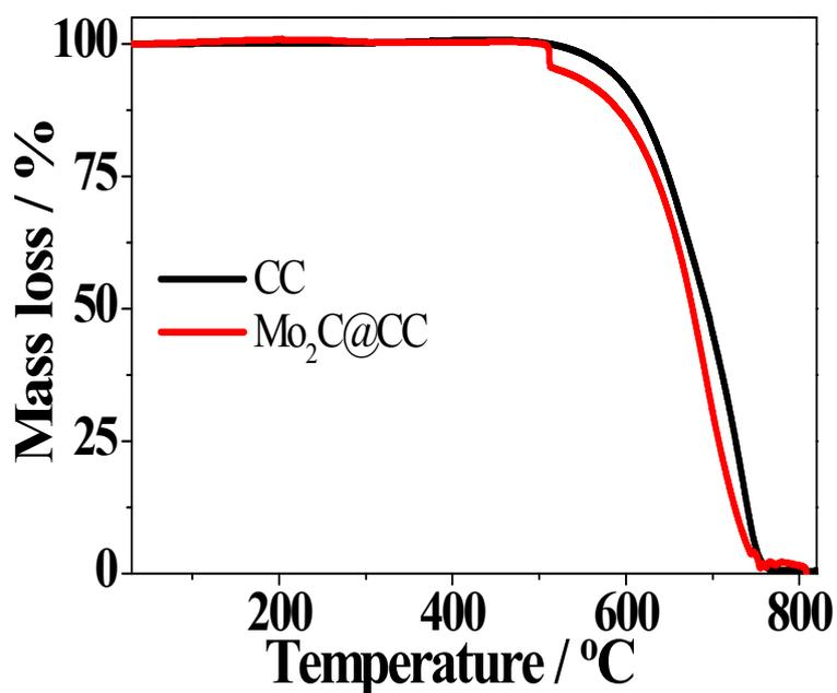
**Figure S1.** TG profiles of pure CC and Mo<sub>2</sub>C@CC electrodes measured at a heating rate of 10 °C min<sup>-1</sup> under air flow, respectively.
