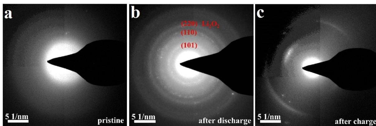
**Figure S9.** SAED patterns of pristine  $Mo_2C@CC$  electrode (a),  $Mo_2C@CC$  electrode after discharged at 2.2 V for 5 h (b), and  $Mo_2C@CC$  electrode after recharged at 4.0 V for 5 h (c), respectively.
