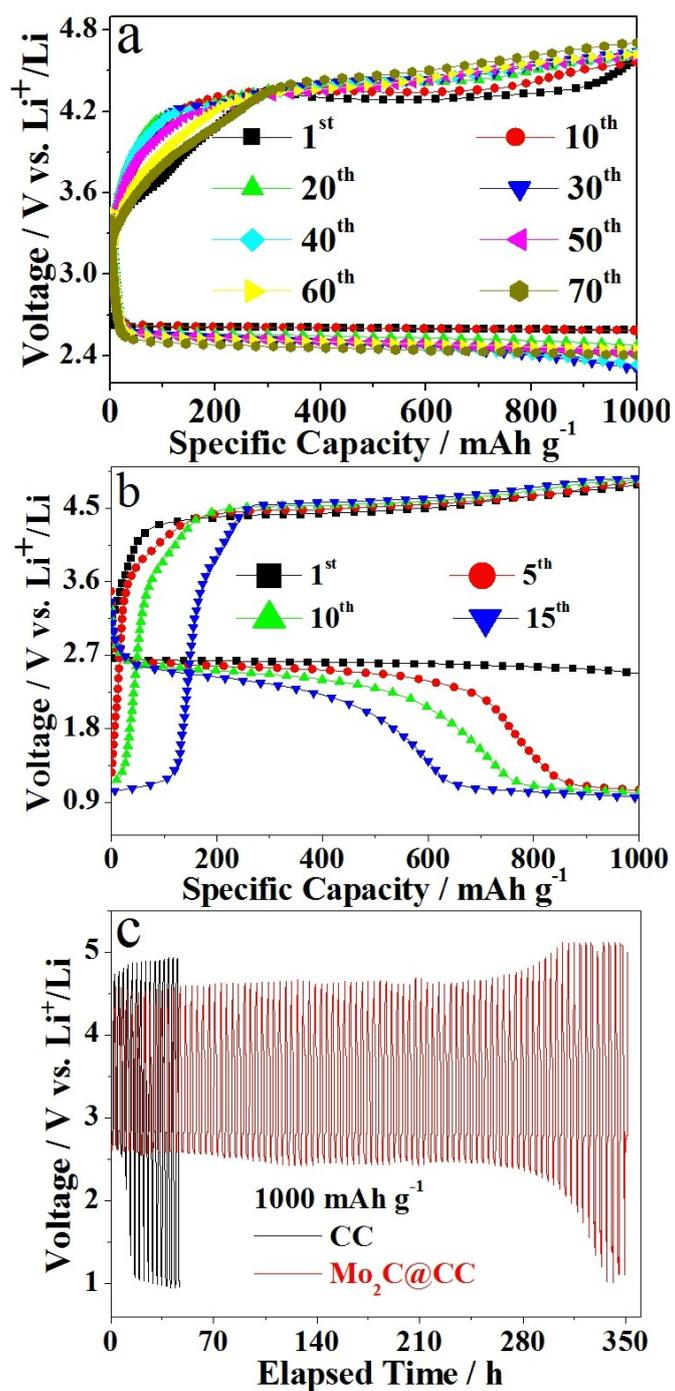
**Figure S5.** Cycling performances of CC (a and c) and Mo<sub>2</sub>C@CC (b and c) electrode based LOBs at a current density of 1000 mA g<sup>-1</sup> with a cut-off capacity of 1000 mAh g<sup>-1</sup>, respectively.
