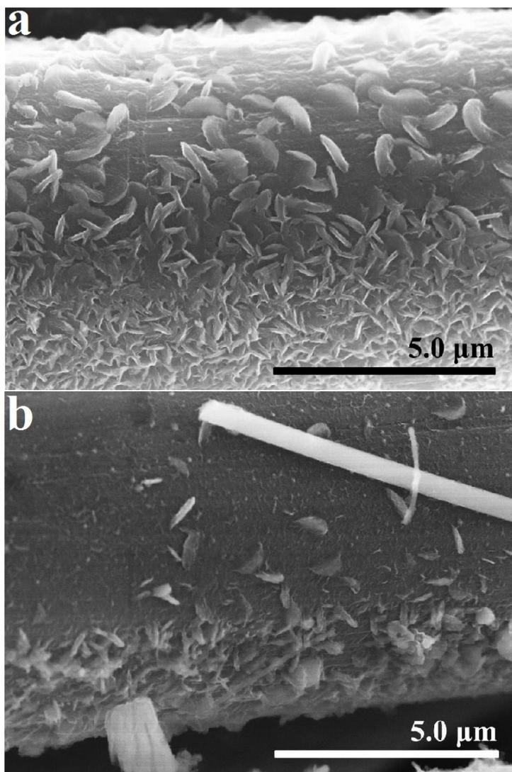
**Figure S8.** SEM images of CC electrode after discharged at 2.2 V (a) and charged at 4.0 V (b).
