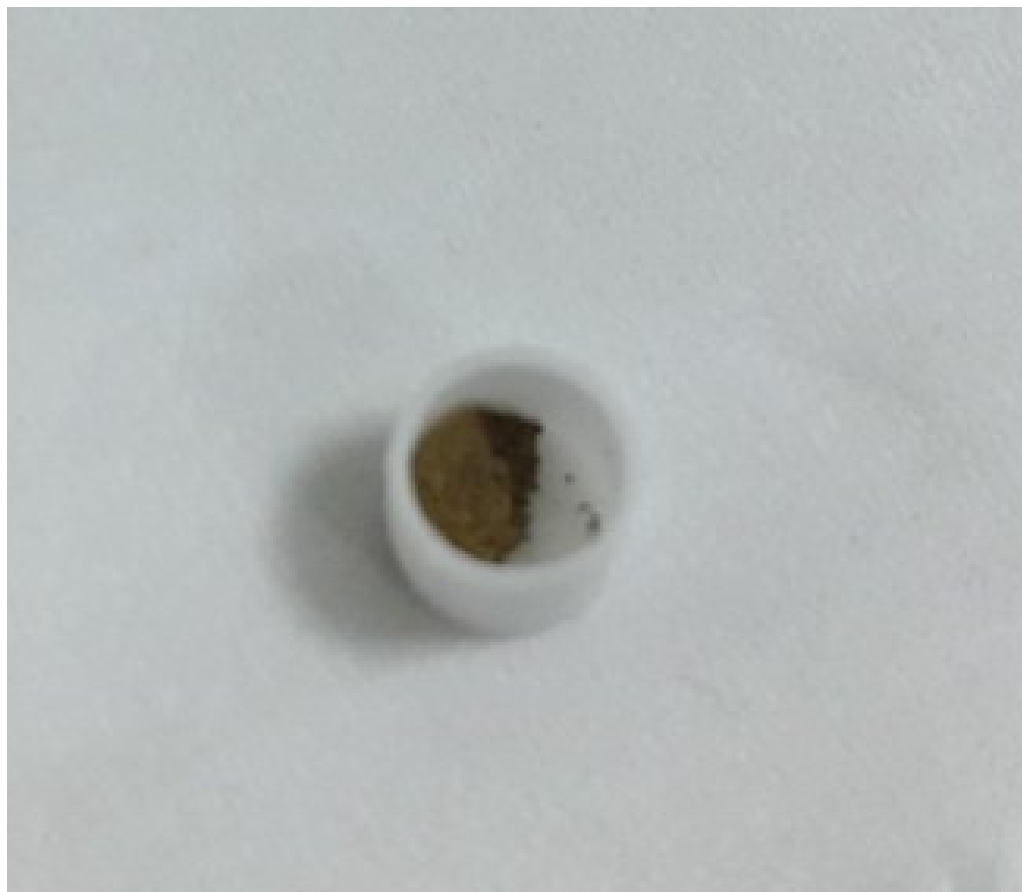
Fig. S1 Si/SiO x @C sample after TGA in air changed from a black color to brownish.
