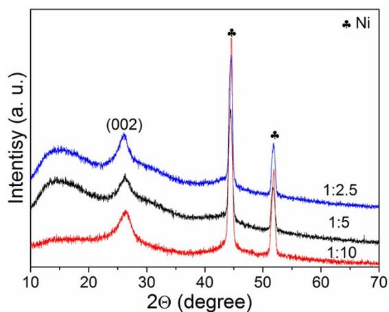
**Fig. S4** Powder XRD patterns of the obtained Ni@NCNTs-CS by using different mass ratios between nickelocene and melamine: 1:2.5, 1:5 and 1:10.
