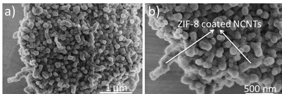
**Fig. S8** SEM images of the obtained NCNTs-CS-ZIF-8 composite.
