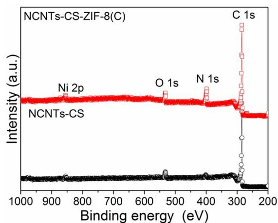
**Fig. S10** XPS spectrum of a) NCNTs-CS and b) NCNTs-CS-ZIF-8(C).
