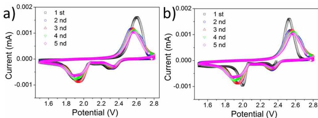
**Fig. S16** CVs of a) S/NCNTs-CS and b) S/NCNTs-CS-ZIF-8(C) in the voltage range of 1.5-2.8 V versus  $\text{Li}^+/\text{Li}$ .
