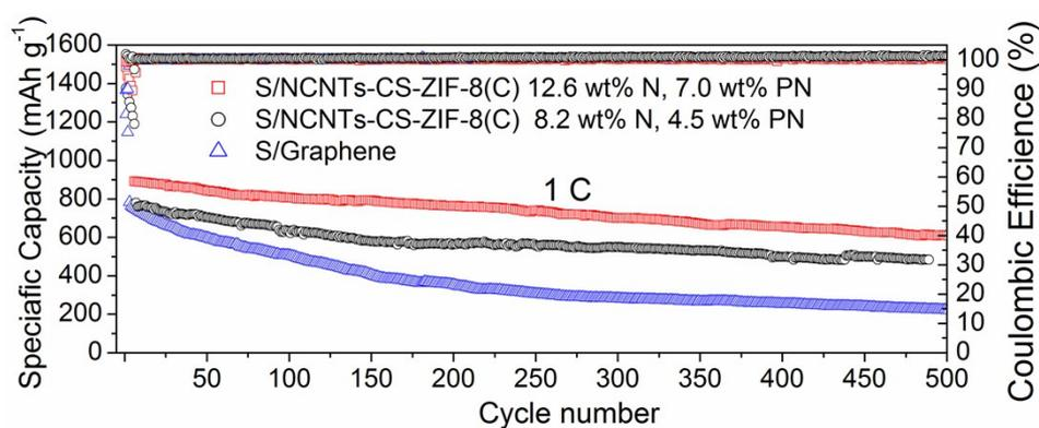
**Fig. S18** The long-term cycling performance and Coulombic efficiencies of S/Graphene and S/NCNTs-CS-ZIF-8(C) with different nitrogen content at 1 C.
