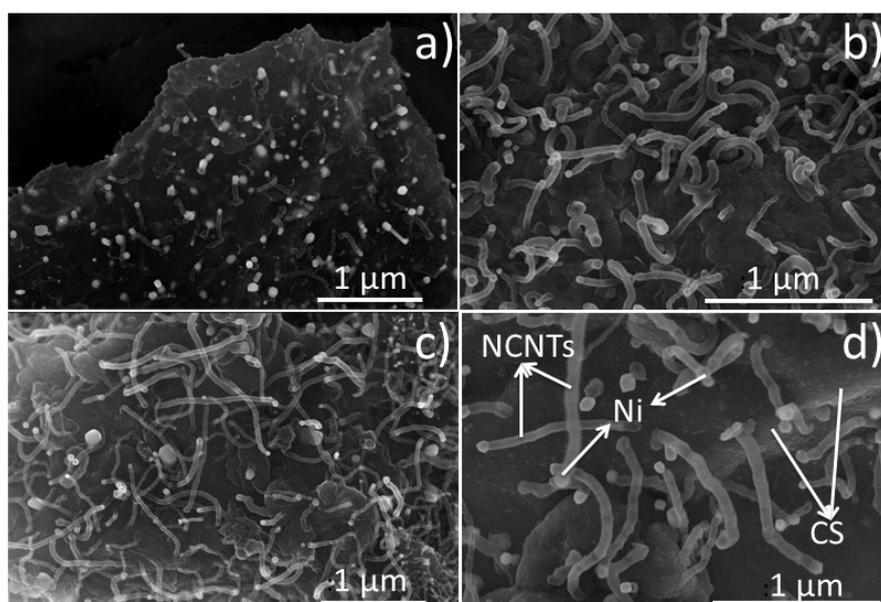
**Fig. S2** SEM images of the obtained Ni@NCNTs-CS by using different mass ratios between nickelocene and melamine: a) 1:2.5, b) 1:5 and c) 1:10. d) SEM images of the obtained NCNTs-CS at Ar- $\text{H}_2$  atmosphere using 1:10 ratios between nickelocene and melamine.
