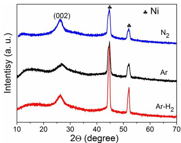
**Fig. S3** Powder XRD patterns of as-prepared Ni@NCNTs-CS at N<sub>2</sub>, Ar and Ar-H<sub>2</sub> atmosphere.
