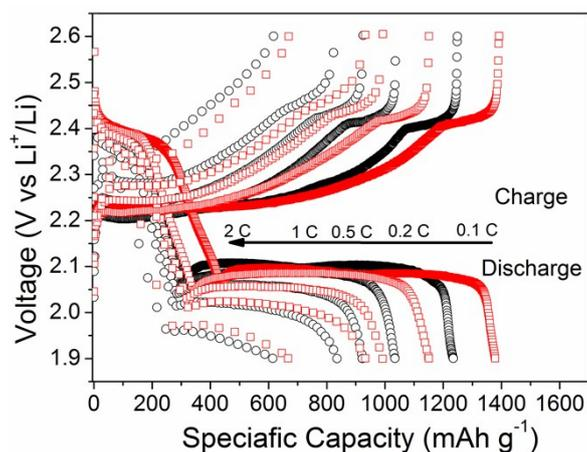
**Fig. S17** The discharge-charge curves of the batteries with the S/NCNTs-CS and S/NCNTs-CS-ZIF-8(C) cathodes at different C rates.
