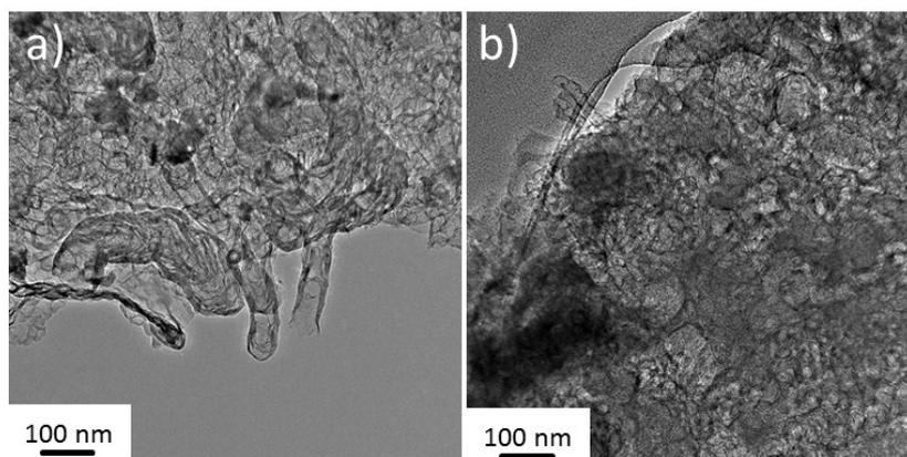
**Fig. S14** TEM images of a) S/NCNTs-CS and b) S/NCNTs-CS-ZIF-8(C).
