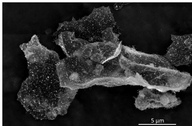
**Fig. S6** SEM images of the obtained Ni@NCNTs-CS at Ar atmosphere using 1:5 ratios between nickelocene and melamine.
