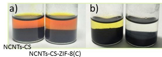
**Fig. S12** Sealed vials of a lithium polysulfides solution ( $\text{Li}_2\text{S}_6$  dissolved in DOL/DME solvents) containing NCNTs-CS and NCNTs-CS-ZIF-8(C) powder: (a) after 0 h, (b) after 0.5 h.
