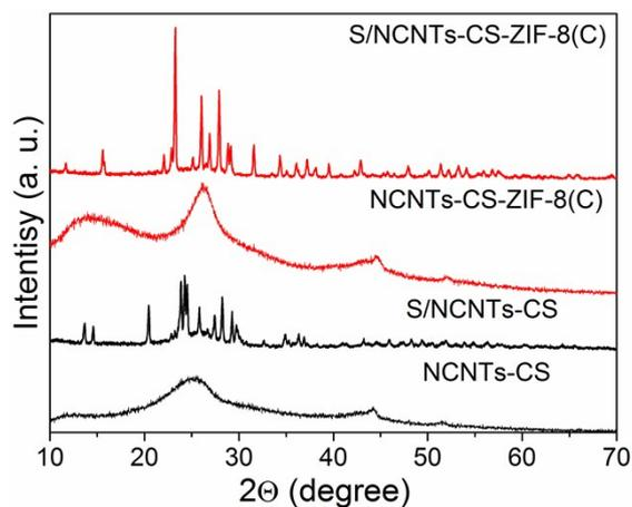
**Fig. S9** Powder XRD patterns of as-prepared NCNTs-CS, ZIF-8, NCNTs-CS-ZIF-8 and NCNTs-CS-ZIF-8(C).
