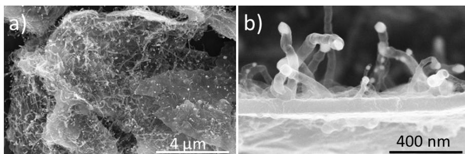
**Fig. S5** SEM images of the obtained Ni@NCNTs-CS at N<sub>2</sub> atmosphere using 1:10 ratios between nickelocene and melamine.
