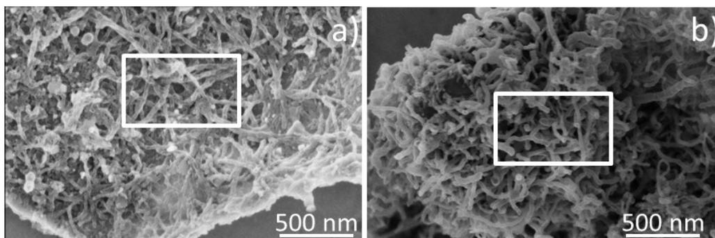
**Fig. S13** SEM images of a) S/NCNTs-CS and b) S/NCNTs-CS-ZIF-8(C).
