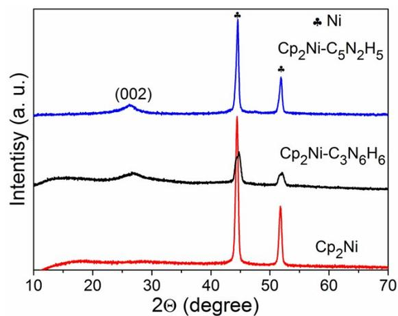
**Fig. S1** Powder XRD patterns of the calcined products by using nickelocene, nickelocene ( $\text{Cp}_2\text{Ni}$ ) and 2-methylimidazole ( $\text{C}_5\text{N}_2\text{H}_5$ ), nickelocene and melamine ( $\text{C}_3\text{N}_6\text{H}_6$ ).
