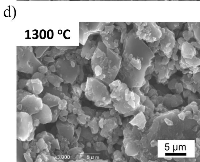
**Figure S3:** Electrode morphology observed by SEM of a) Argan-800, b) Argan-1000, c) Argan-1200, and d) Argan-1300.
