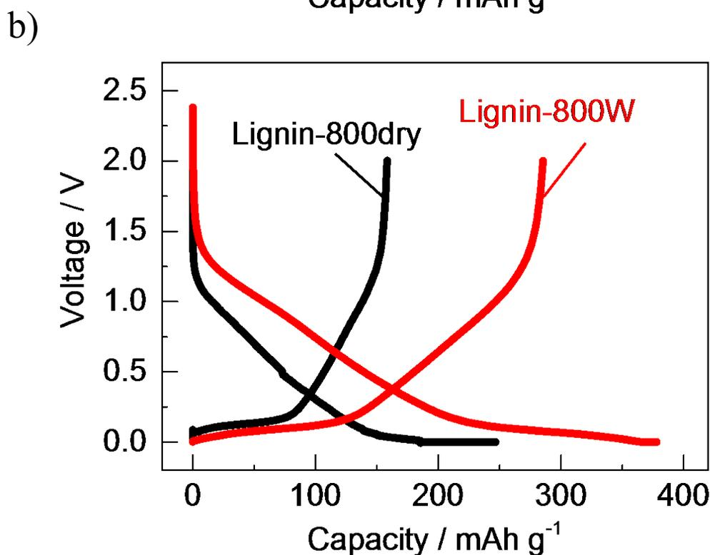
**Figure S14:** First charge/discharge profiles of a) Cellulose-800, Cellulose-800dry, and Cellulose-800W, b) Lignin-800, and Lignin-800W electrodes cycled between 2 and 0 V at a rate of 25 mA g<sup>-1</sup> in 1.0 mol dm<sup>-3</sup> NaPF<sub>6</sub> EC:DEC.
