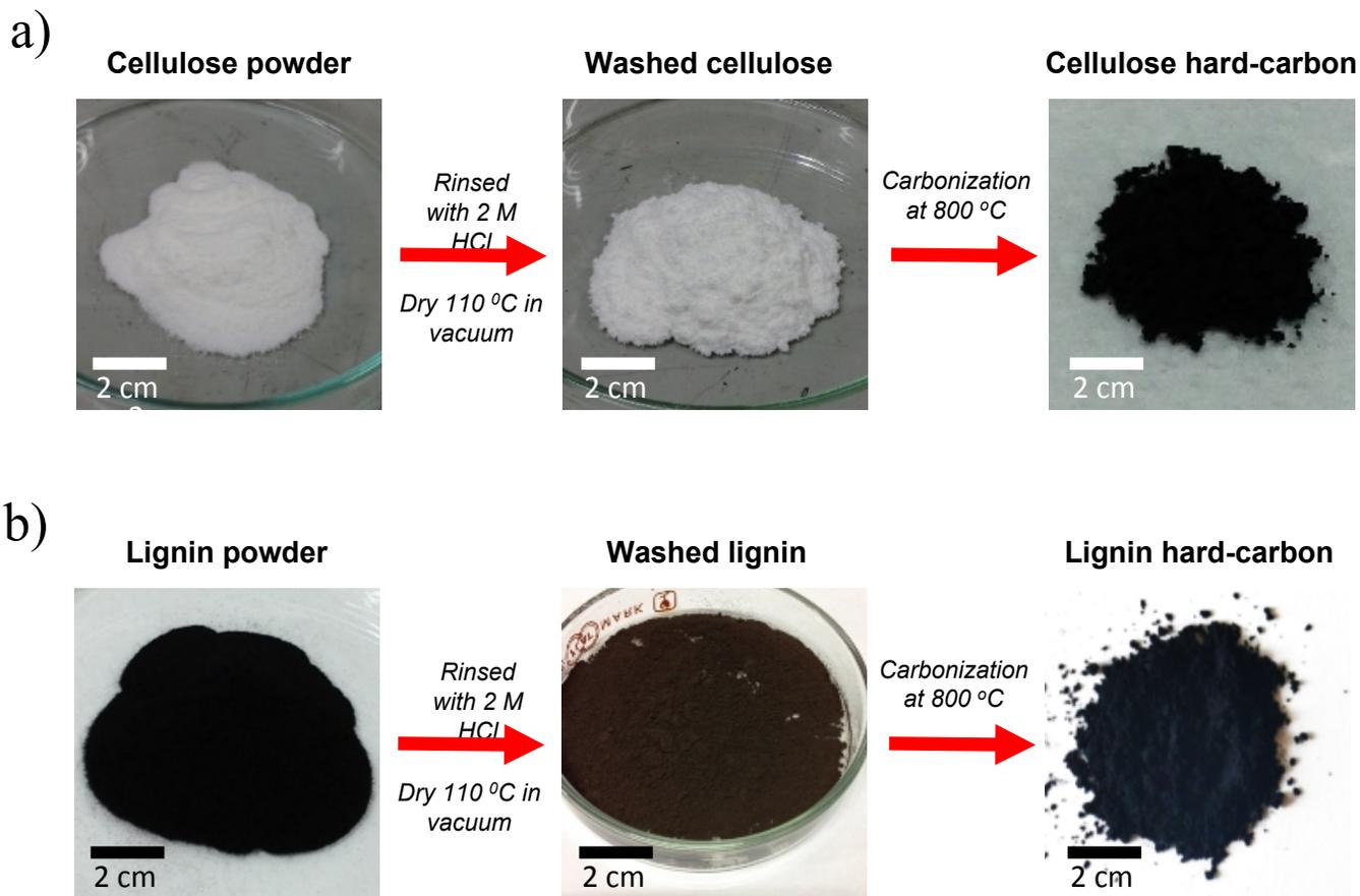
**Figure S1:** Cellulose and lignin materials synthesis processes with and without HCl treatment at 800 °C.
