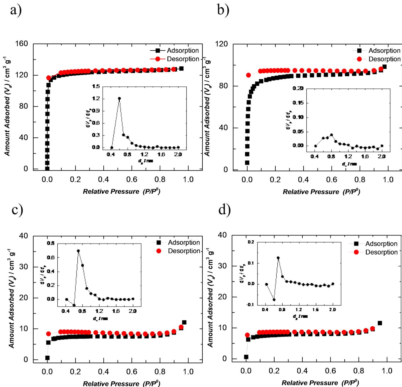
**Figure S8:**  $N_2$  adsorption-desorption isothermal curve of HCl-treated materials a) argan-800W, b) argan-1000W, c) argan-1200W, and d) argan-1300W. The insert is corresponding pore size distribution.
