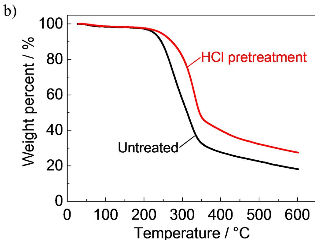
**Figure S5:** a) XRF spectra of untreated Argan-1000 (black curve), Argan-1200 (red curve) and Argan-1300 (blue curve). b) TGA analysis of untreated (black curve) and HCl washed (red curve) Argan raw materials before carbonization.
