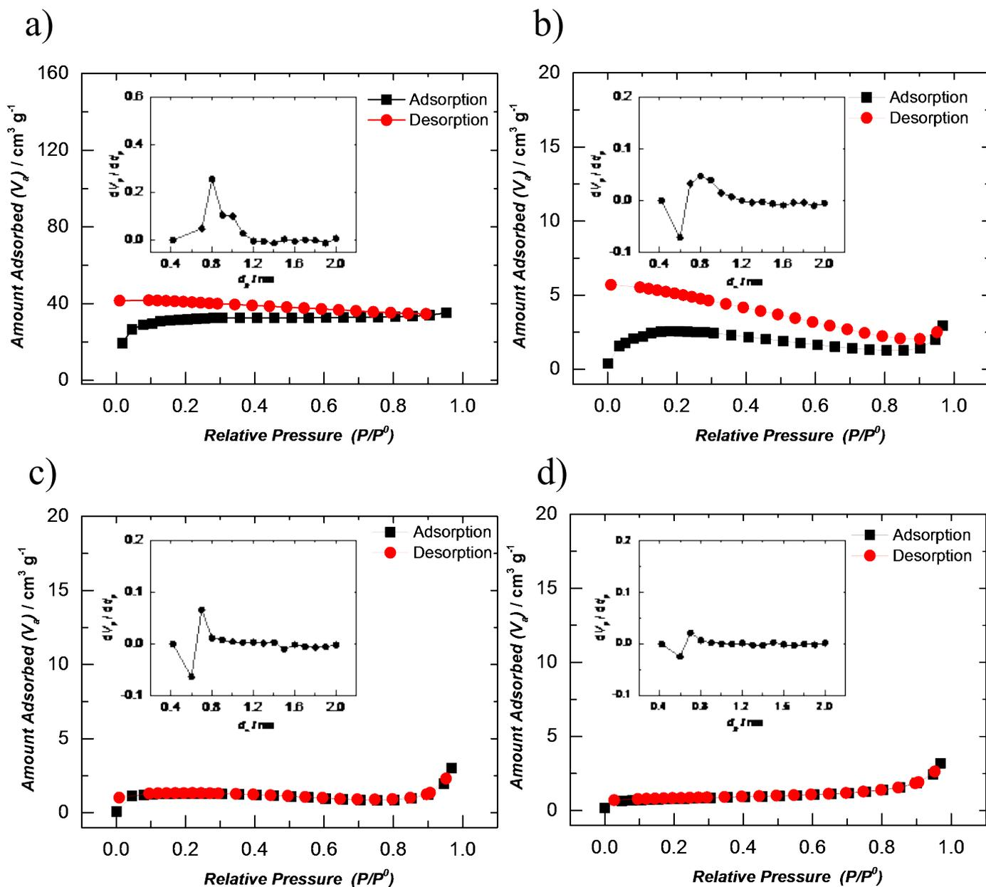
**Figure S4:**  $N_2$  adsorption-desorption isothermal curve of a) Argan-800, b) Argan-1000, c) Argan-1200, and d) Argan-1300. The insert is corresponding pore size distribution.
