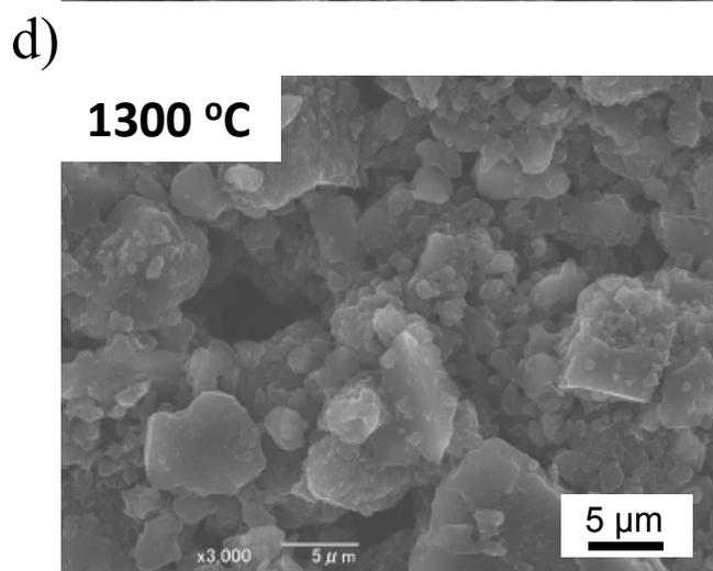
**Figure S7:** Electrode morphology observed by SEM of HCl-treated materials a) Argan-800W, b) Argan-1000W, c) Argan-1200W, and d) Argan-1300W.
