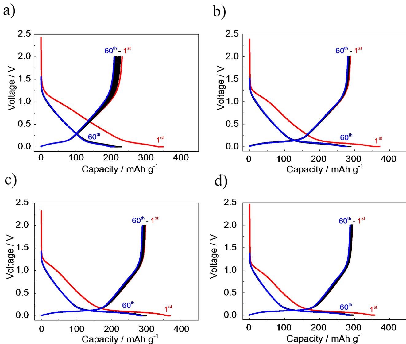
**Figure S12:** Charge/discharge curves of a) Argan-800, b) Argan-1000, c) Argan-1200, and d) Argan-1300 electrodes with PANA binder cycled between 2.0 and 0.0 V at a rate of 25 mA g<sup>-1</sup> in 1.0 mol dm<sup>-3</sup> NaPF<sub>6</sub> EC:DEC solution.
