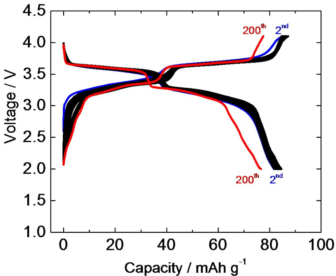
**Figure S16:** Galvanostatic charge/discharge curves of Na/Na<sub>2/3</sub>Ni<sub>1/3</sub>Mn<sub>2/3</sub>O<sub>2</sub> in Na cell at 25 mA g<sup>-1</sup> in 1.0 mol dm<sup>-3</sup> NaPF<sub>6</sub>/EC/DEC.
