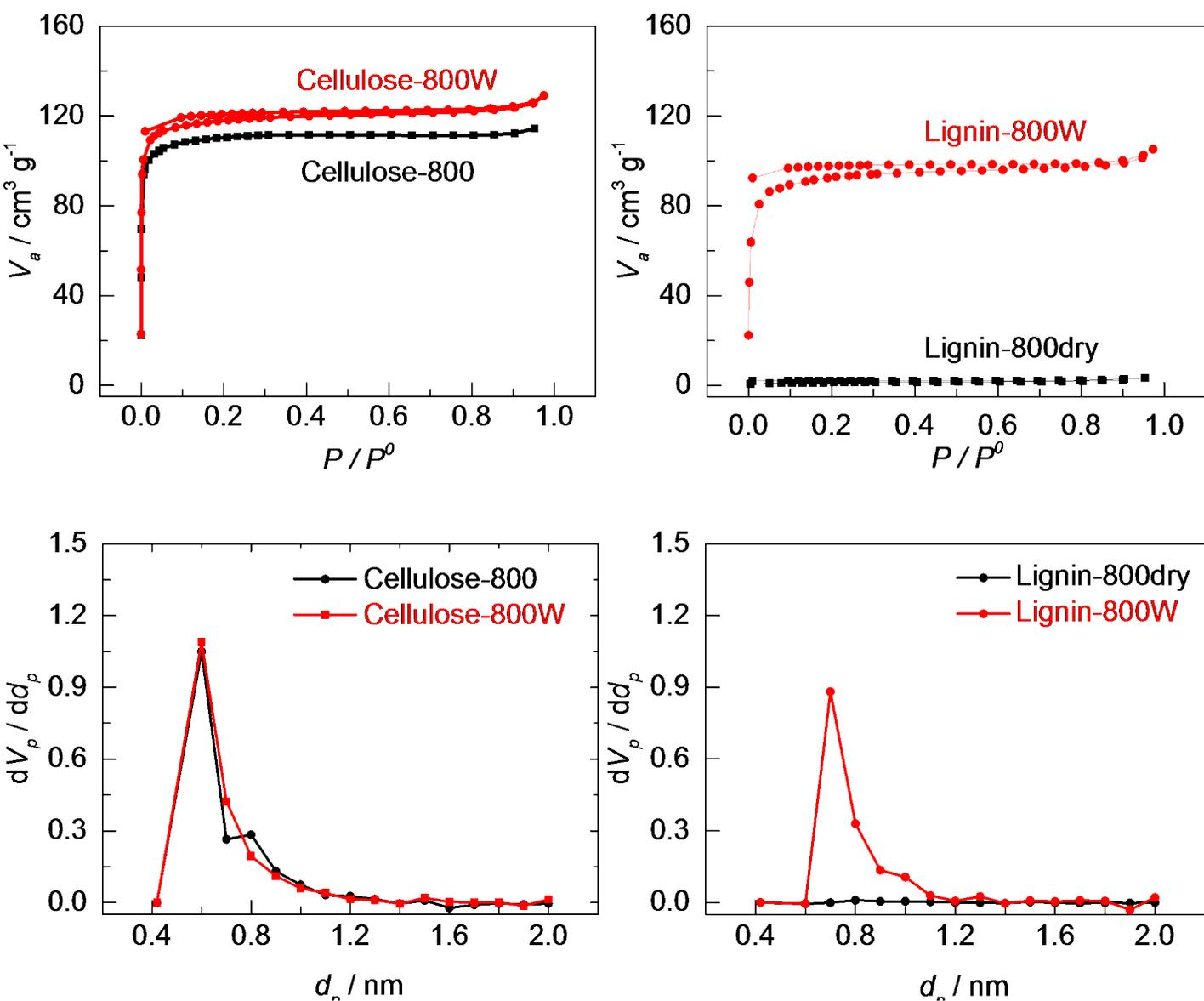
**Figure S11:**  $N_2$  adsorption–desorption isothermal curve (top) and corresponding pore size distribution (down) of cellulose and lignin materials.
