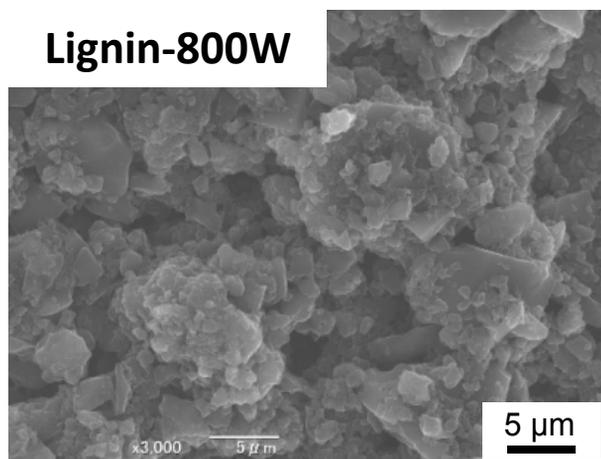
**Figure S10:** Electrode morphology observed by SEM of carbonized cellulose and lignin materials at 800 °C: a) cellulose-800, b) cellulose-800W, c) lignin-800, and d) lignin-800W.
