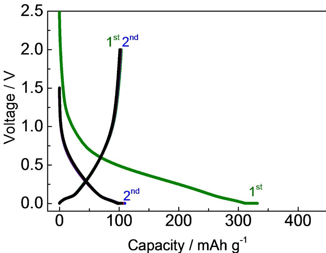
**Figure S13:** Charge/discharge profiles of Argan-1300W electrode pretreated by HCl without drying in vacuum at 110 °C, cycled between 2 and 0 V in PANa binder at a rate of 25 mA g<sup>-1</sup> in 1.0 mol dm<sup>-3</sup> NaPF<sub>6</sub>/EC/DEC.
