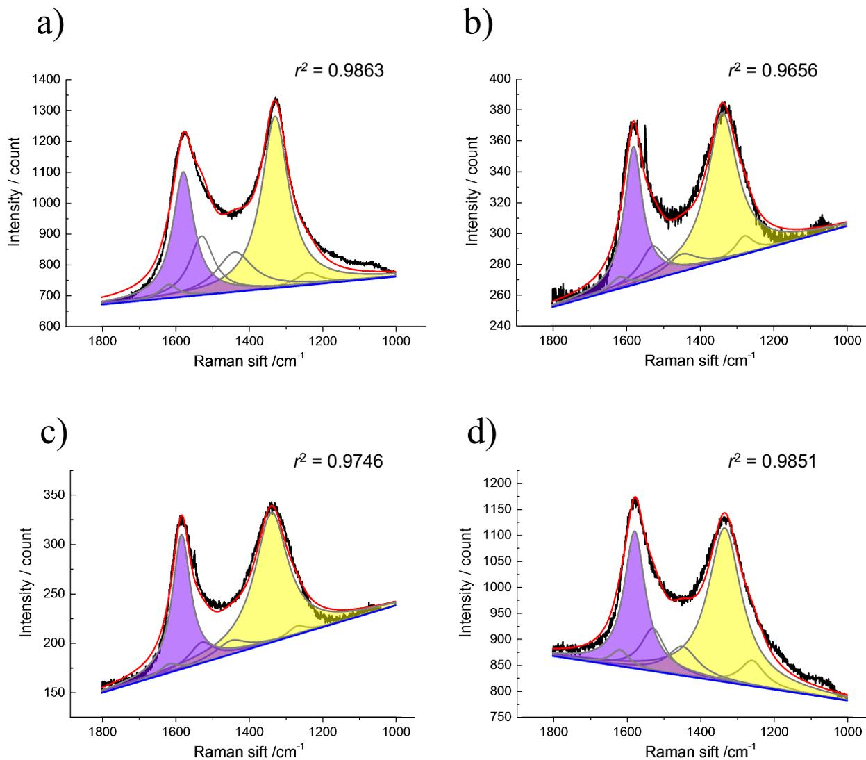
**Figure S6:** Fitted Raman spectra profiles of HCl washed argan materials a) Argan-800W, b) Argan-1000W, c) Argan-1200W, and d) Argan-1300W. The fitting was done with Fityk 0.9.0 software using Lorentzian function.
