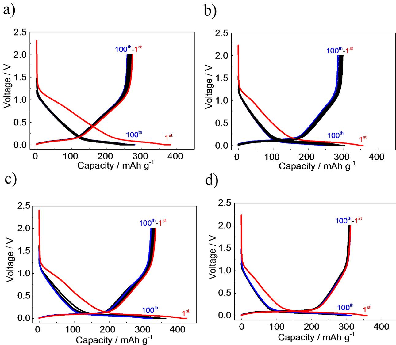
**Figure S15:** Charge/discharge curves of a) Argan-800W, b) Argan-1000W, c) Argan-1200W, and d) Argan-1300W electrodes with PANA binder cycled between 2.0 and 0.0 V at a rate of 25 mA g<sup>-1</sup> in 1.0 mol dm<sup>-3</sup> NaPF<sub>6</sub> EC:DEC solution.
