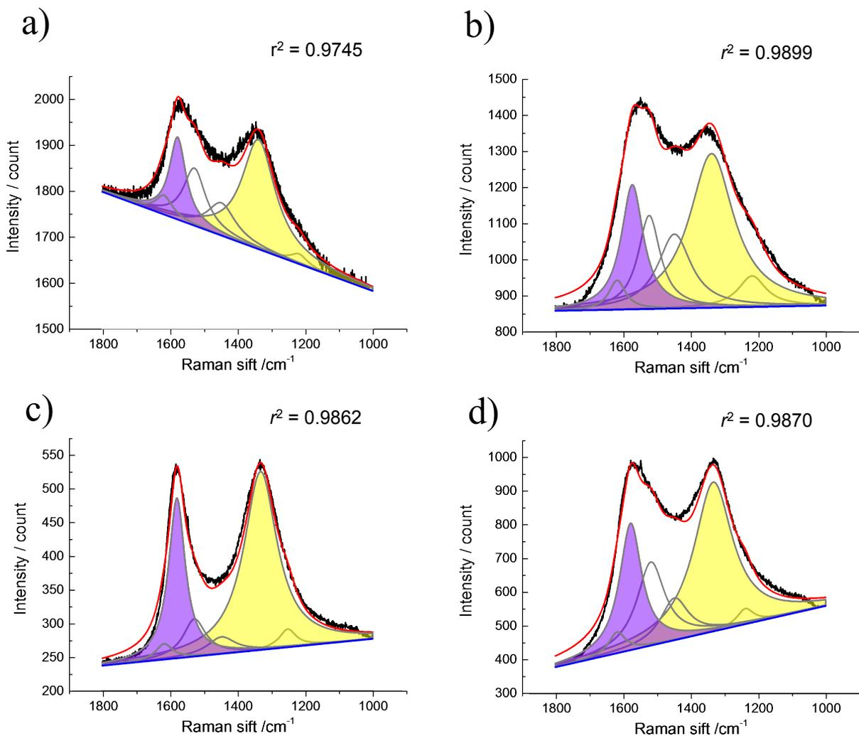
**Figure S2:** Fitted Raman spectra profiles of a) Argan-800, b) Argan-1000, c) Argan-1200, and d) argan-1300. The fitting was done with Fityk 0.9.0 software program using Lorentzian function.
