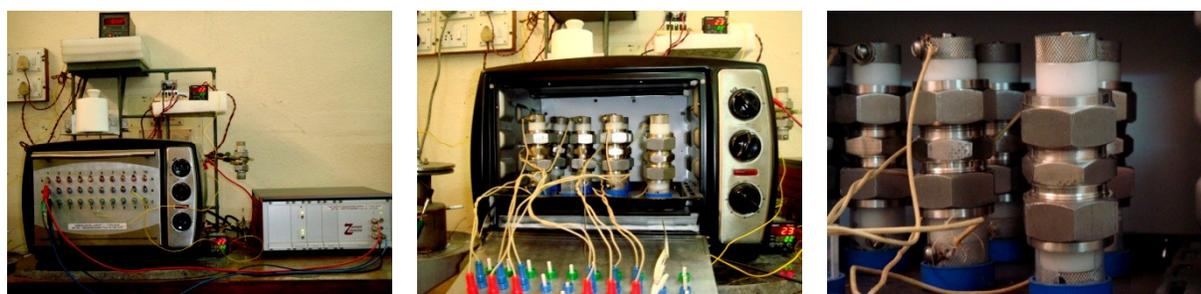
**Figure SI-2(b).** Typical photographs depicting the experimental set-up used for electrochemical evaluation during an ongoing investigation. The system is interfaced with a thermostated oven equipped with parallel test channels independently connected to spring loaded Swagelok cells to test the samples at identical conditions.
