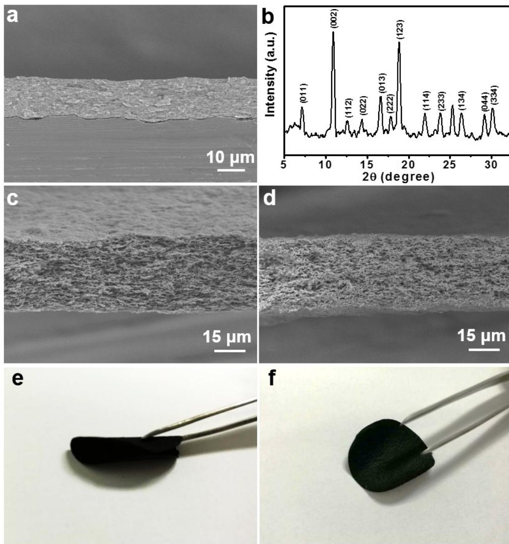
**Figure S1.** (a), (c) and (d) SEM of ZHN/CNT, CNCF-5/1 and CNCF-15/1, respectively; (b) XRD pattern of ZIF-8/CNT; (e) and (f) digital photograph of bended and released CNCF-10/1.
