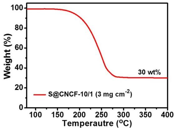
**Figure S6.** (a) The TGA curve of S@CNCF-10/1 electrode with a sulfur loading of  $3 \text{ mg cm}^{-2}$  in  $\text{N}_2$  with a heating rate of  $5 \text{ }^{\circ}\text{C min}^{-1}$ , indicating sulfur content of  $\sim 70 \text{ wt\%}$ .
