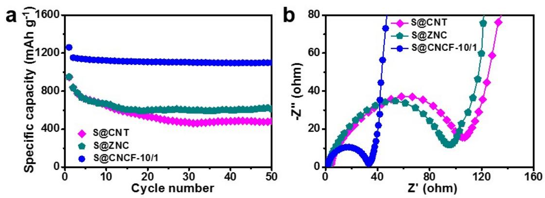
**Figure S8.** (a) cycling performance of S@CNT, S@ZNC and S@CNCF-10/1; (b) EIS spectra of the samples.
