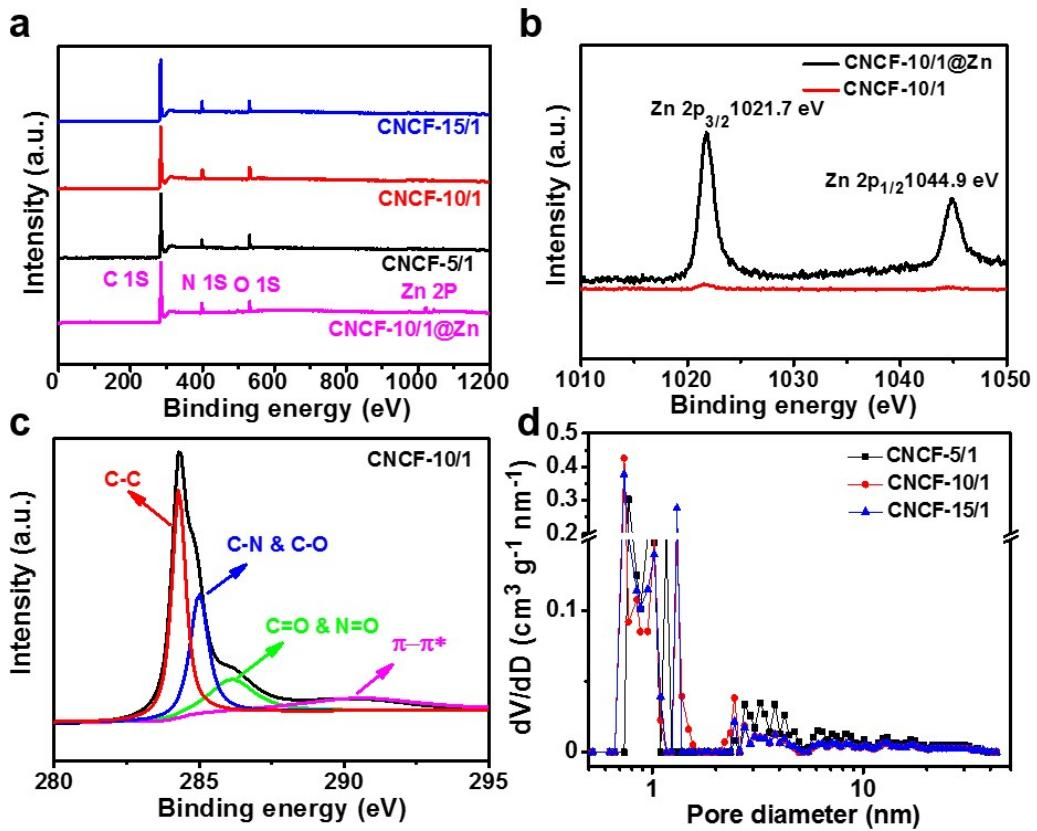
**Figure S4.** (a) Overview XPS spectra of CNCF-5/1, 10/1, 15/1 and CNCF-10/1@Zn; (b) comparison of Zn 2p spectra between CNCF-10/1@Zn and CNCF-10/1; (c) C 1s spectra of CNCF-10/1; (d) DFT pore-size distribution of CNCF-5/1, 10/1 and 15/1.
