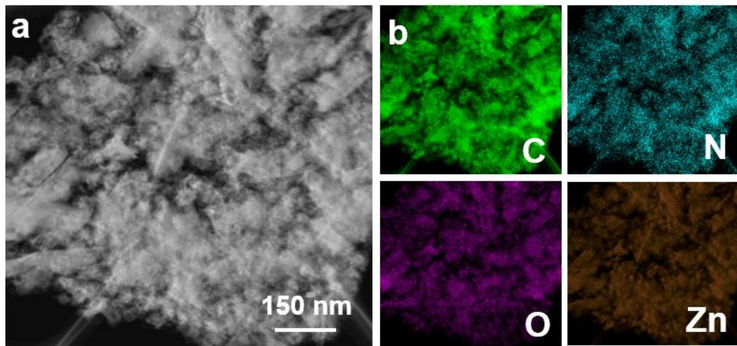
**Figure S3.** (a) TEM and (b) mapping results of CNCF-10/1@Zn.
