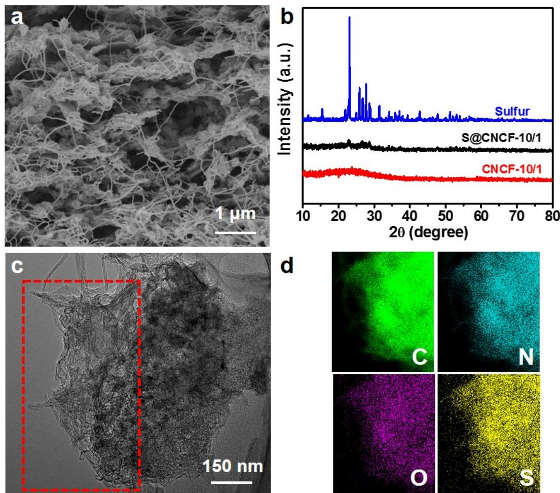
**Figure S7.** (a) SEM image of S@CNCF-10/1 electrode; (b) XRD pattern of CNCF-10/1 and S@CNCF-10/1; (c) and (d) TEM image and mapping results of S@CNCF-10/1.
