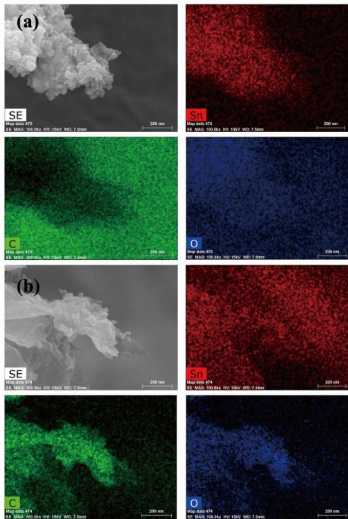
**Figure S4.** EDS mappings of SnO<sub>2</sub>/G-S (a) and SnO<sub>2</sub>/G-O (b) composites.
