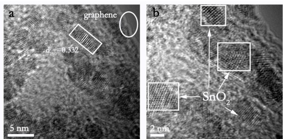
**Figure S5.** HRTEM images prepared  $\text{SnO}_2/\text{G-S}$  through one-step synergistic effect of  $\text{SnO}_2$  nanoparticles' formation and GO's reduction.
