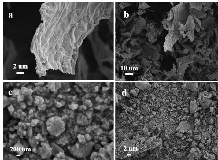
**Figure S3.** SEM images of prepared pristine graphene (a, b) and SnO<sub>2</sub>(c, d)
