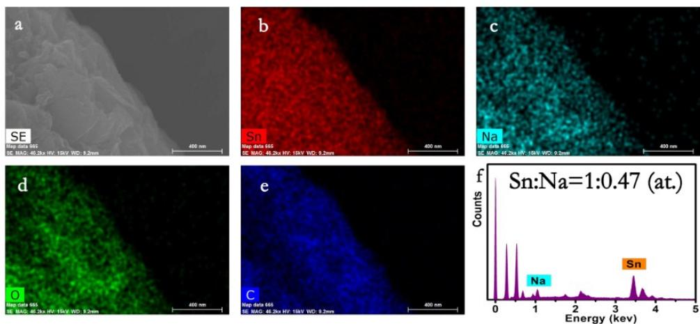
**Figure S12.** EDS mappings (a, b, c, d, e) and EDS spectra (f) of  $\text{SnO}_2/\text{G-S}$  electrode after desodiation to 3V in Na-ion batteries.
