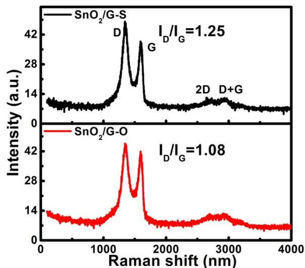
**Figure S7.** Raman spectra of SnO<sub>2</sub>/G-S and SnO<sub>2</sub>/G-O, ratio of  $I_D/I_G$  is generally used for degree of defect in the graphene roughly.
