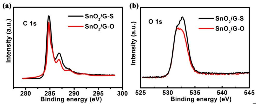
**Figure S6.** high-resolution C 1s (a) and O 1s (b) XPS spectrum of the SnO<sub>2</sub>/G-S and SnO<sub>2</sub>/G-O composites.
