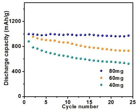
**Figure S15.** Comparison of cycling stability and reversible capacity of  $\text{SnO}_2/\text{G}$  materials with different loading of  $\text{SnO}_2$  active materials.
