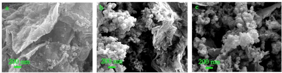
**Figure S14.** SEM images of  $\text{SnO}_2/\text{G-S-80}$ (a),  $\text{SnO}_2/\text{G-S-60}$ (b) and  $\text{SnO}_2/\text{G-S-40}$ (c) materials
