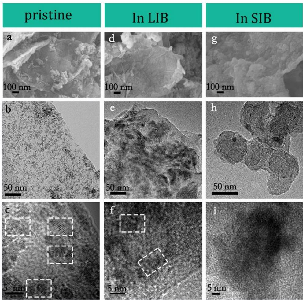
**Figure S13.** Morphology of pristine  $\text{SnO}_2/\text{G-S}$  through one-step synergetic effect of  $\text{SnO}_2$  nanoparticles' formation and GO's reduction.(a, b, c) after 10 cycles in Li-ion batteries.(b, e, f) after 10 cycles in Na-ion batteries.(g, h, i) SEM images.(a, d, g) TEM images.(b, e, h, c, f, i).
