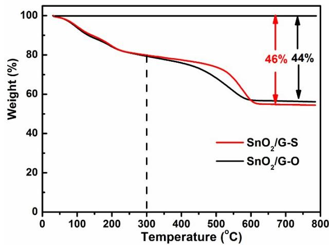
**Figure S2.** Thermogravimetric analysis curves of prepared  $\text{SnO}_2/\text{G-S}$  through one-step synergistic effect and  $\text{SnO}_2/\text{G-O}$  through two-step method in order of  $\text{SnO}_2$  nanoparticles' formation and GO's reduction.
