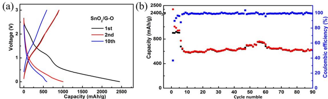
**Figure S9.** The electrochemical performance of prepared SnO<sub>2</sub>/G-O electrode through two-step method in order of SnO<sub>2</sub> nanoparticles' formation and GO's reduction in Na-ion batteries.
