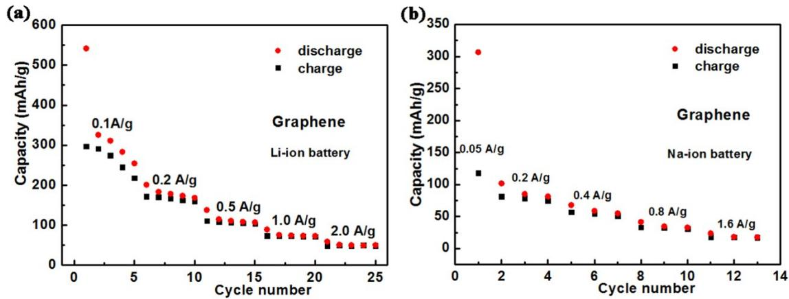
**Figure S8.** The electrochemical performance of prepared pristine graphene as working electrode in Li-ion batteries (a) and Na-ion batteries (b), respectively.
