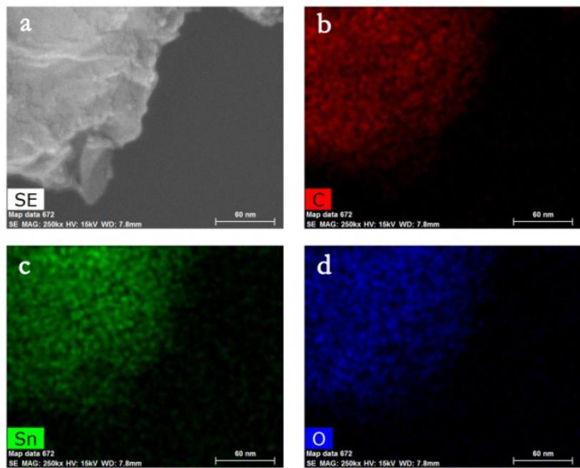
**Figure S10.** EDS mappings (a, b, c, d) of  $\text{SnO}_2/\text{G-S}$  electrode after 10 cycles in Li-ion batteries.
