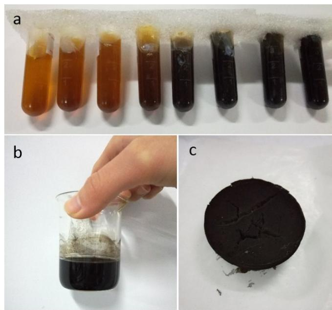
**Figure S1.** (a), The process that graphene oxide was reduced by  $\text{Na}_2\text{S}_2\text{O}_3$ , in order from left to right, pristine GO, adding  $\text{Na}_2\text{S}_2\text{O}_3$ , 5, 10, 15, 30, 60, and 120 min. (b), dispersion of graphene after 24 h, no layer. (c), graphene after freeze-drying.
