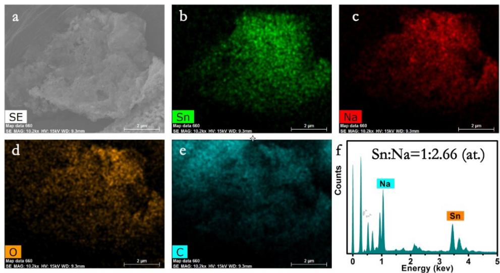
**Figure S11.** EDS mappings (a, b, c, d, e) and EDS spectra (f) of  $\text{SnO}_2/\text{G-S}$  electrode after sodiation to 0.01V in Na-ion batteries.
