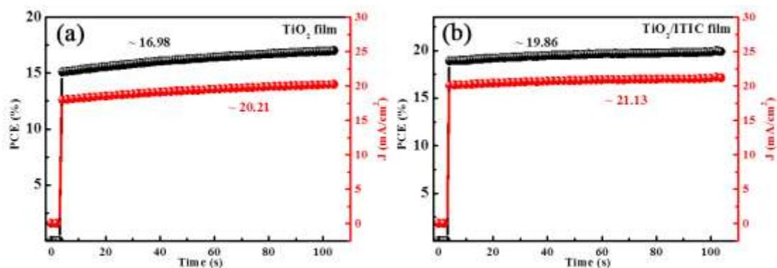
**Figure S8.** PCE measured as a function of time for the cells biased at 0.84 V for (a) TiO<sub>2</sub> ETL and 0.94 V for (b) ITIC modified TiO<sub>2</sub> ETL.
