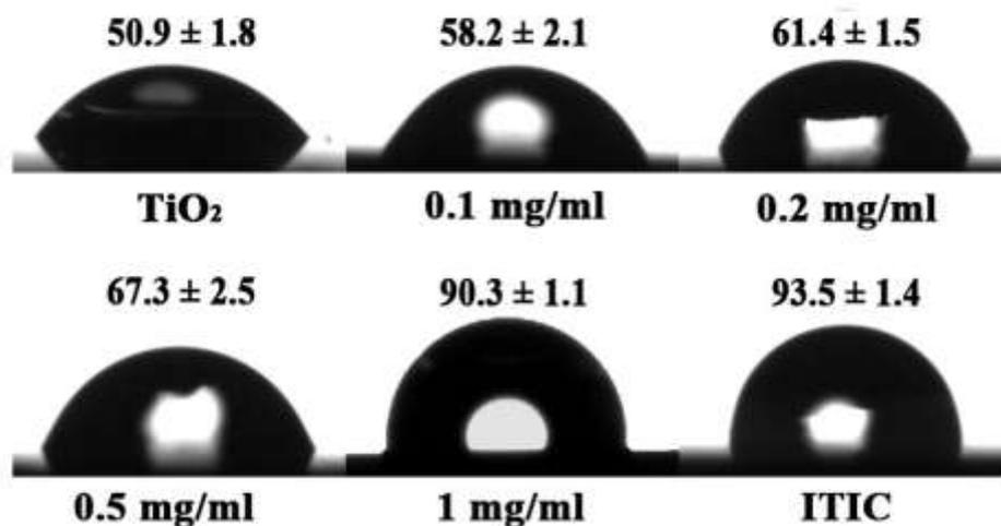
**Figure S2.** Photographs of water droplet on: pristine TiO<sub>2</sub> film, different concentrate ITIC modified TiO<sub>2</sub> film and pristine ITIC film.
