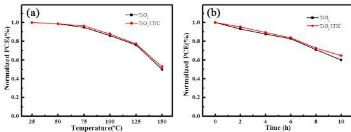
**Figure S9.** Normalized PCEs of PSCs with or without ITIC modified TiO<sub>2</sub> ETL: (a) after annealing different temperature for 10 min and (b) after annealing at 80 °C for different times.
