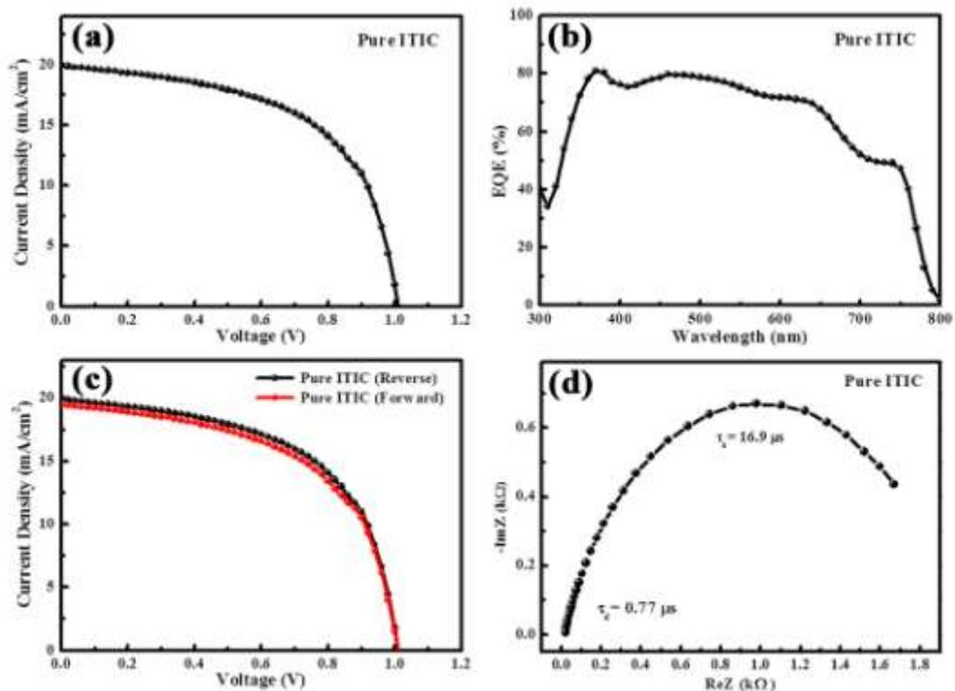
**Figure S3.** Properties of the perovskite solar cells based on ITIC ETL: (a) for J-V characteristics, (b) for EQE curve, (c) for J-V characteristics with different sweep directions (scan rate 200mV/s), (d) for IS result.
