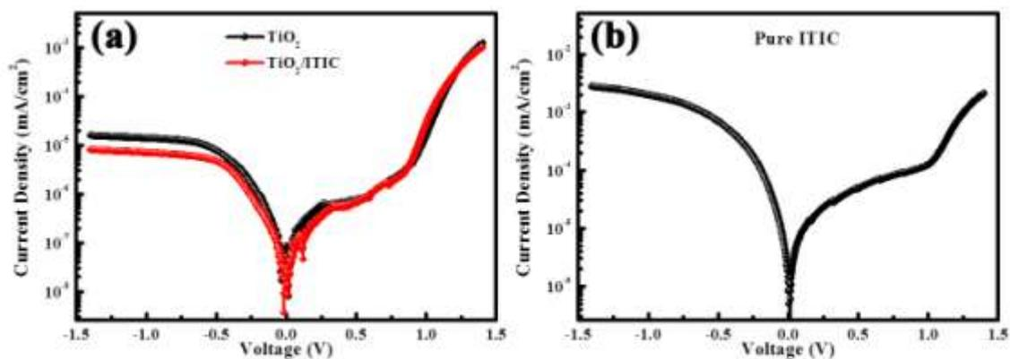
**Figure S6.** J-V characteristics of the fabricated perovskite photovoltaic solar cells with different ETL in dark condition: (a) for  $\text{TiO}_2$  ETL and  $\text{TiO}_2/\text{ITIC}$  ETL, (b) for ITIC ETL.
