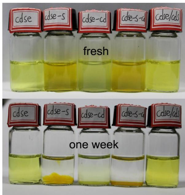
**Figure S3** Images of CdSe QDs solution, CdSe QDs with one monolayer of S added, CdSe QDs with one monolayer of Cd added, CdSe QDs with one monolayer of S added and an additional layer of Cd added, and as prepared CdSe/CdS QDs.
