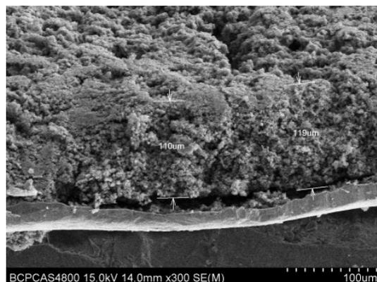
**Figure S2.** The morphologies of the CS@CTAB/ABS composite electrode (S content: 76 wt% in electrode, S mass loading:  $6.7 \text{ mg cm}^{-2}$ ).
