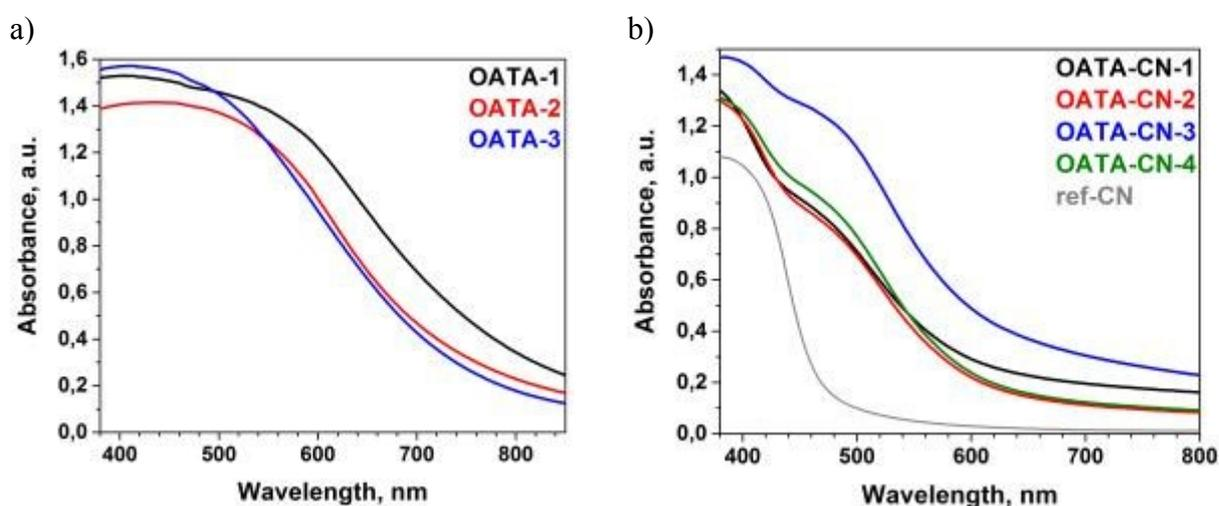
Figure S9. UV-Vis absorption spectra of OATA-N (a) and OATA-CN-N materials compared to ref-CN (b).
