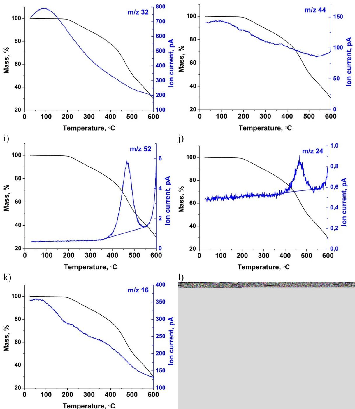
Figure S3. TGA and MS ion current curves for the selected mass numbers measured for OATA-1 sample. Analysis was performed using He as a carrier gas. Carrier gas contains  $\leq 2.0$  ppm water,  $\leq 2.0$  ppm oxygen,  $\leq 0.2$  ppm hydrocarbons,  $\leq 5.0$  ppm nitrogen.
