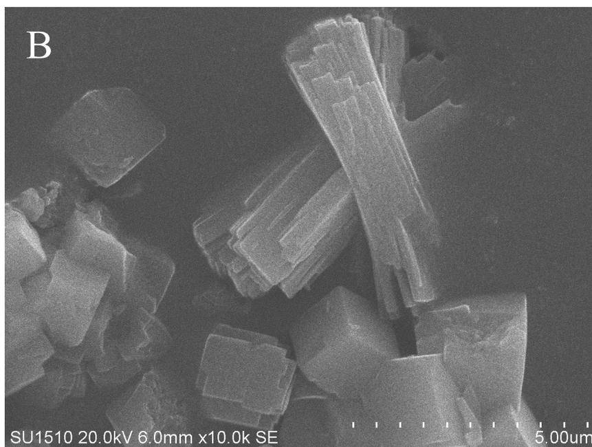
**Fig. S6** (A) XRD pattern (impurity of MOR labelled with an asterisk) and (B) SEM image of CHA-ST without addition of CHA seeds at 150 °C for 7 days.
