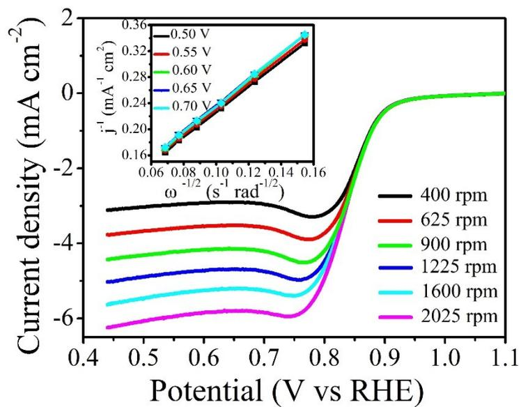
**Fig. S6.** Polarization curves of Ni@Pd<sub>3</sub>/C NPs at various rotating speeds in 0.1 M HClO<sub>4</sub> solution and the corresponding Koutecky-Levich plots at various potentials (Inset image).
