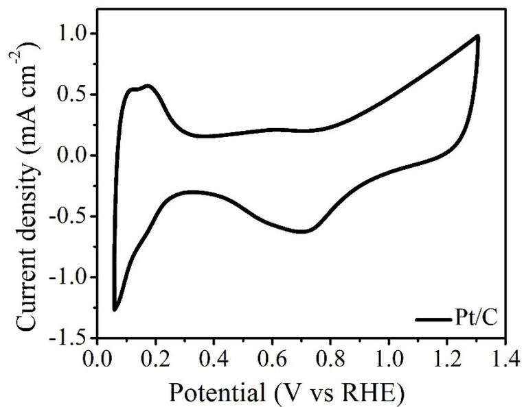
**Fig. S4.** CV curves of the commercial Pt/C (wt.20%) tested in a  $N_2$ -saturated 0.1 M  $HClO_4$  solution at a sweep rate of  $20\ mV\ s^{-1}$ .
