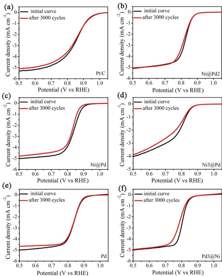
**Fig. S10.** LSV curves of the catalysts before and after 3000 cycles in 0.1 M  $\text{HClO}_4$  solution: (a) Pt/C (wt.20%), (b) Ni@Pd2, (c) Ni@Pd, (d) Ni3@Pd, (e) Pd, and (f) Pd3@Ni.
