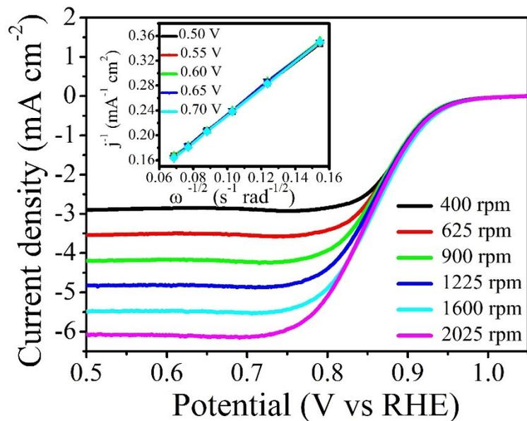
**Fig. S7.** Polarization curves of Ni@Pd<sub>3</sub>/C NPs at various rotating speeds in 0.1 M KOH solution and the corresponding Koutecky-Levich plots at various potentials (Inset image).
