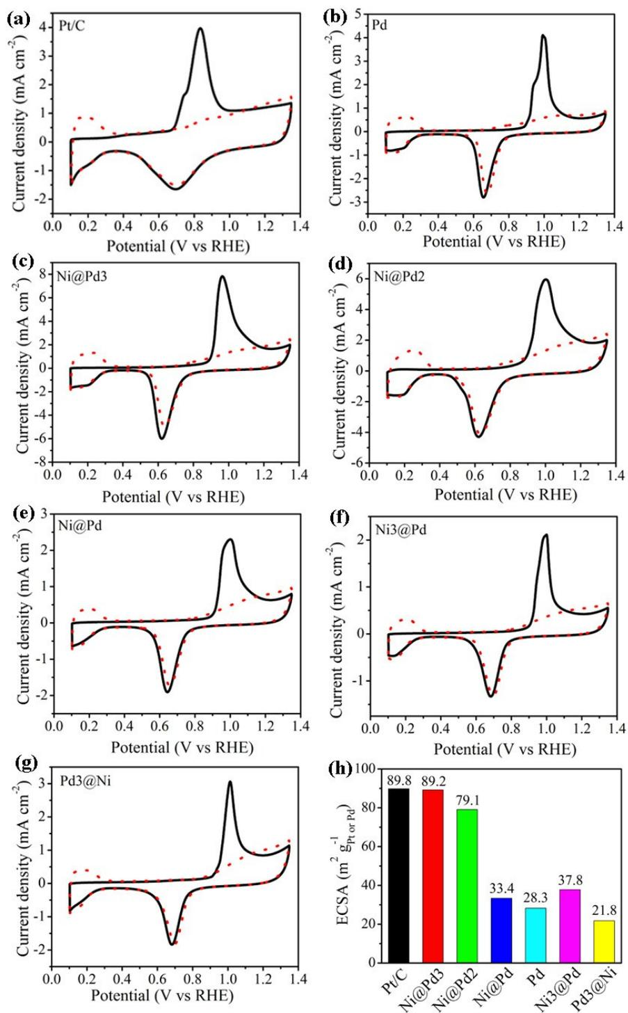
**Fig. S13.** (a-g) CO-stripping voltammograms of Pt/C and the as-prepared catalysts in 0.1 M HClO<sub>4</sub> solutions at a scan rate of 20 mV s<sup>-1</sup> with the first cycle (black solid line) and the second cycle (red dot line), and (h) ECSA for Pt/C and the as-prepared catalysts.
