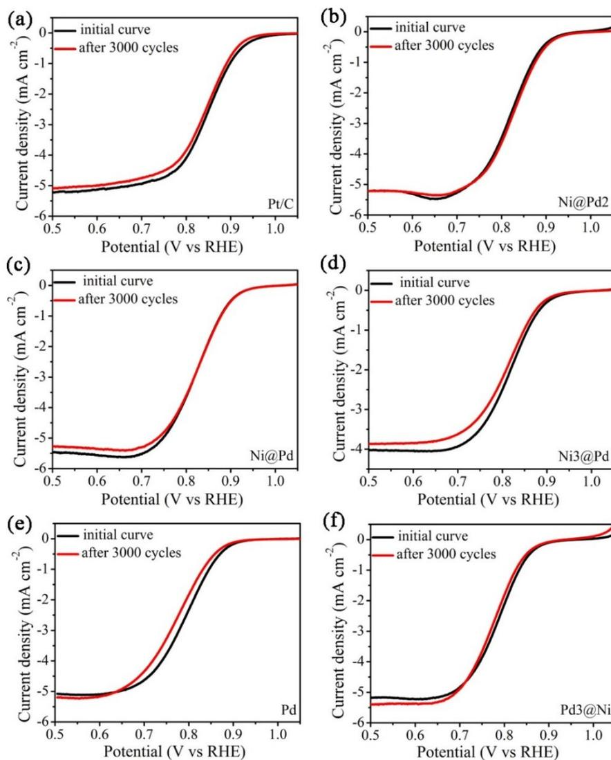
**Fig. S11.** LSV curves of the catalysts before and after 3000 cycles in 0.1 M KOH solution: (a) Pt/C (wt.20%), (b) Ni@Pd<sub>2</sub>, (c) Ni@Pd, (d) Ni<sub>3</sub>@Pd, (e) Pd, and (f) Pd<sub>3</sub>@Ni.
