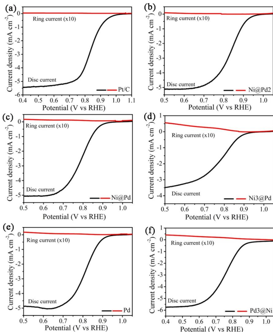
**Fig. S9.** LSV polarization curves of the catalysts at a rotating speed of 1600 rpm in the RRDE tests to calculate the electron transfer number and H<sub>2</sub>O<sub>2</sub>% in 0.1 M KOH solution: (a) Pt/C (wt.20%), (b) Ni@Pd<sub>2</sub>, (c) Ni@Pd, (d) Ni<sub>3</sub>@Pd, (e) Pd, and (f) Pd<sub>3</sub>@Ni.
