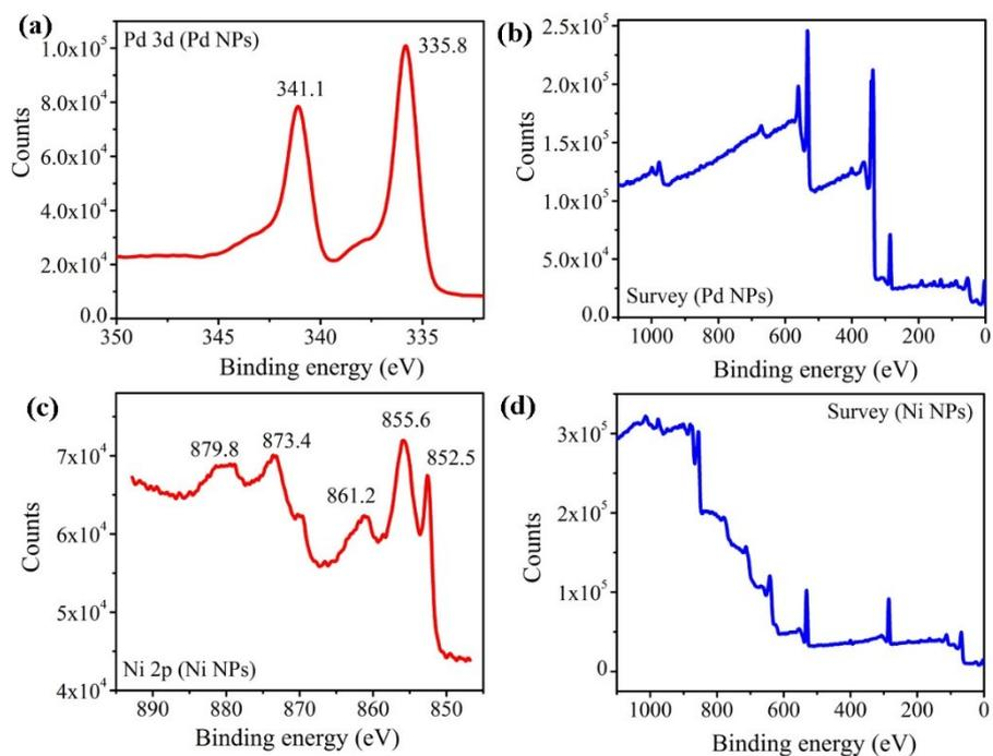
**Fig. S3.** (a-b) Pd 3d and survey signal of the Pd NPs in the XPS spectra; and (c-d) Ni 2p and survey signal of the Ni NPs in the XPS spectra.
