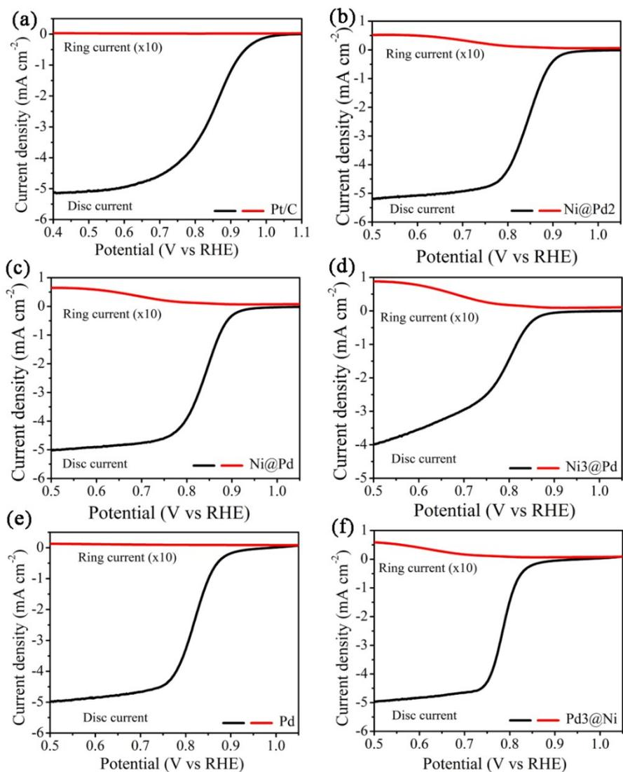
**Fig. S8.** LSV polarization curves of the catalysts at a rotating speed of 1600 rpm in the RRDE tests to calculate the electron transfer number and H<sub>2</sub>O<sub>2</sub>% in 0.1 M HClO<sub>4</sub> solution: (a) Pt/C (wt.20%), (b) Ni@Pd<sub>2</sub>, (c) Ni@Pd, (d) Ni<sub>3</sub>@Pd, (e) Pd, and (f) Pd<sub>3</sub>@Ni.
