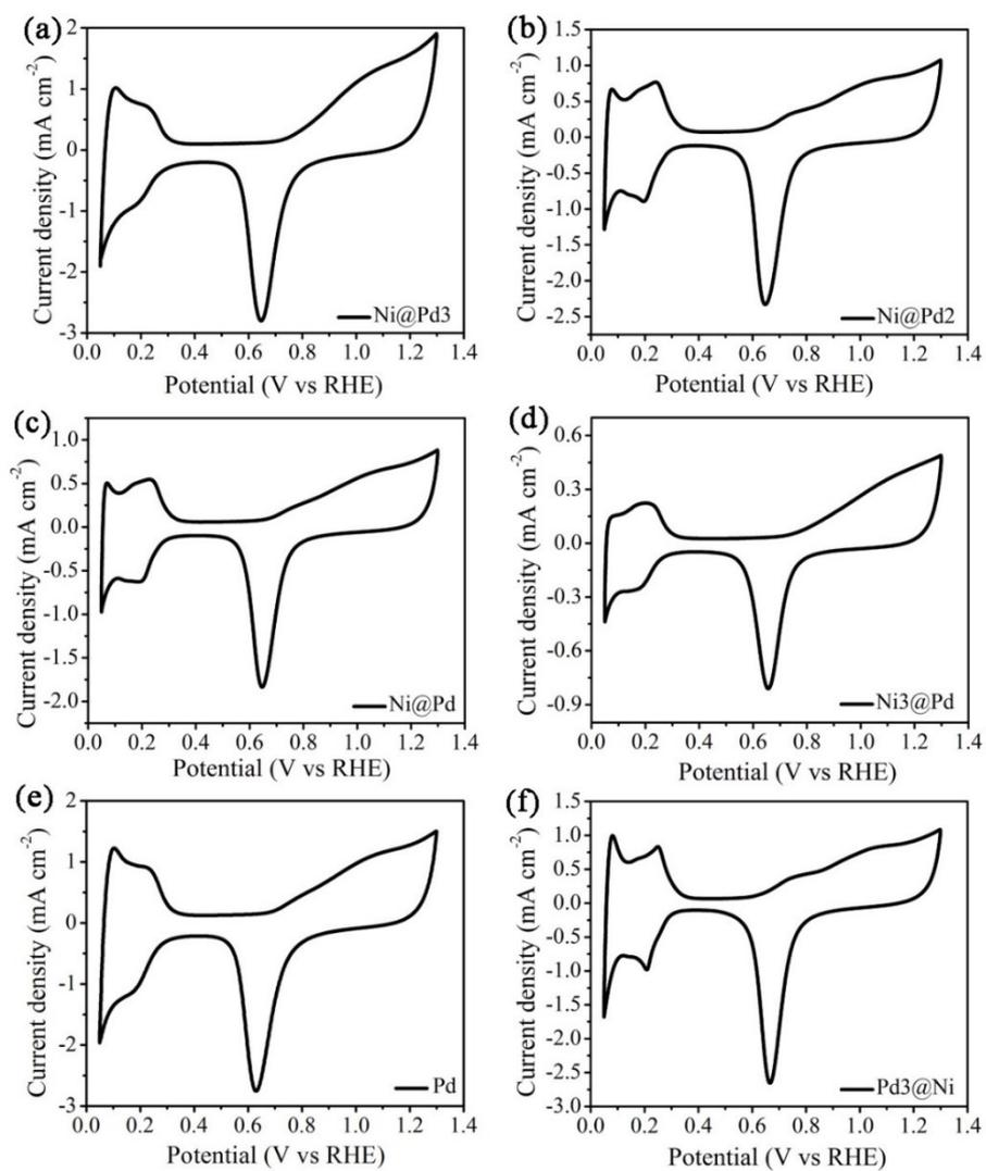
**Fig. S5.** CV curves of the as-prepared catalysts in a N<sub>2</sub>-saturated 0.1 M KOH solution at a sweep rate of 20 mV s<sup>-1</sup>.
