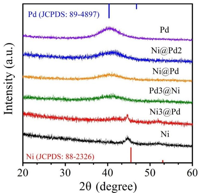
**Fig. S2.** XRD of the products with different molar ratios of precursors (Pd:Ni), including pure Pd, Pd:Ni=2:1 in OAM; Pd:Ni=1:1 in OAM; Pd:Ni=1:3 in OAM; Pd:Ni=3:1 in OAM+ODE; and (f) pure Ni.
