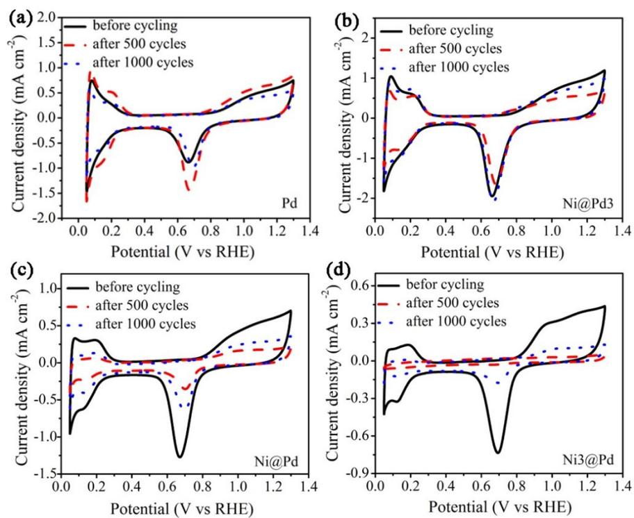
**Fig. S12.** Initial and post-potential cycling CV curves for Pd, Ni@Pd3, Ni@Pd and Ni3@Pd catalysts in N<sub>2</sub>-saturated 0.1 M HClO<sub>4</sub> solution at the sweep rate of 20 mV s<sup>-1</sup> at room temperature.
