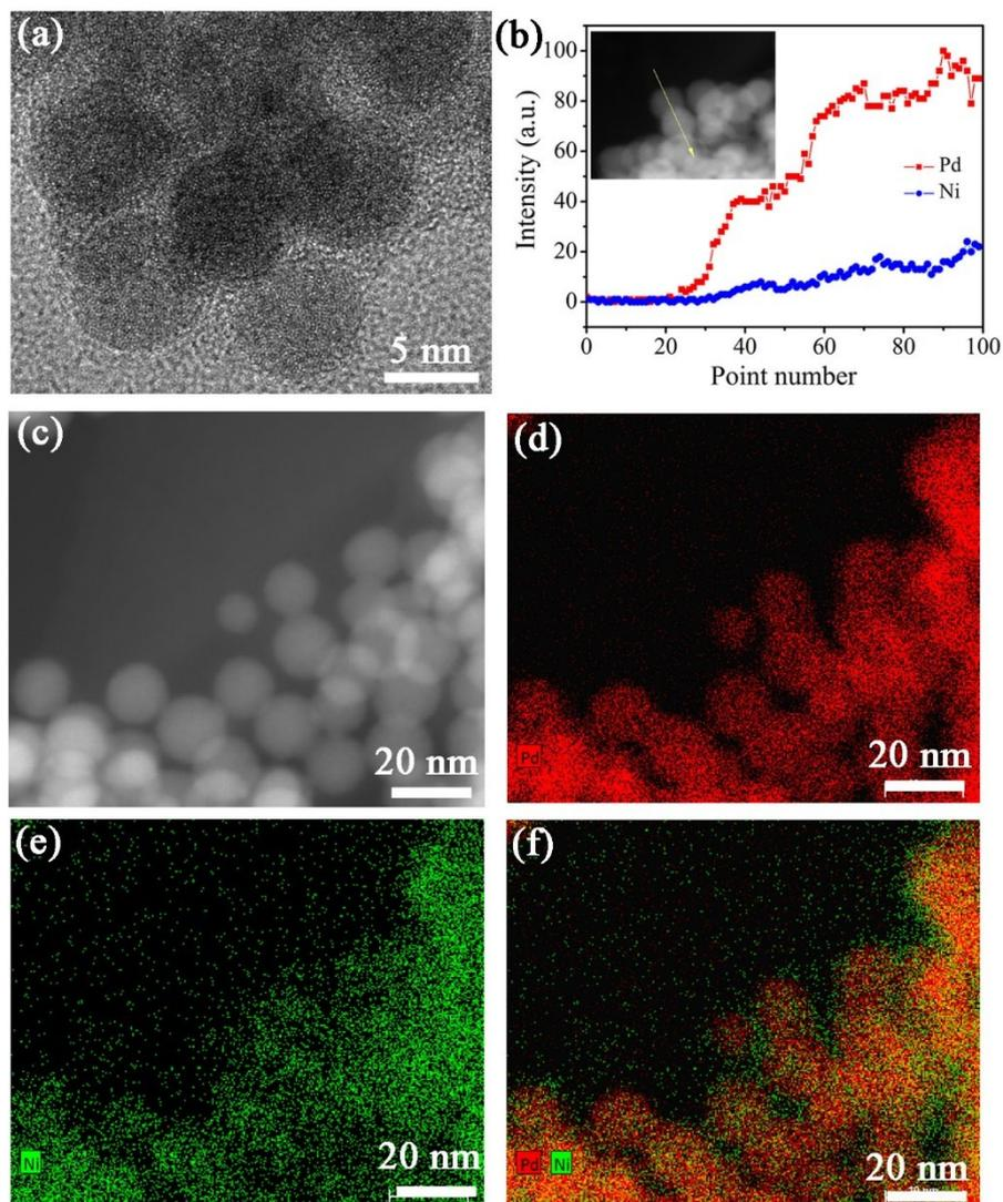
**Fig. S1.** (a) HRTEM image; (b) STEM-EDX line scan; and (c-f) HAADF-STEM image with the corresponding high resolution elemental mapping of the Pd<sub>3</sub>@Ni NPs. Green denotes Ni and red highlights the Pd distribution within NPs.
