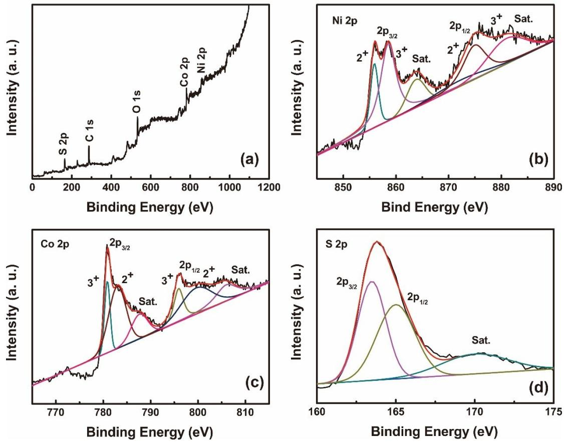
**Figure S4.** (a) XPS full survey spectra and high-resolution XPS spectra of (b) Ni 2p, (c) Co 2p, and (d) S 2p of as-obtained  $\text{NiCo}_2\text{S}_4$  nanosheet sample.
