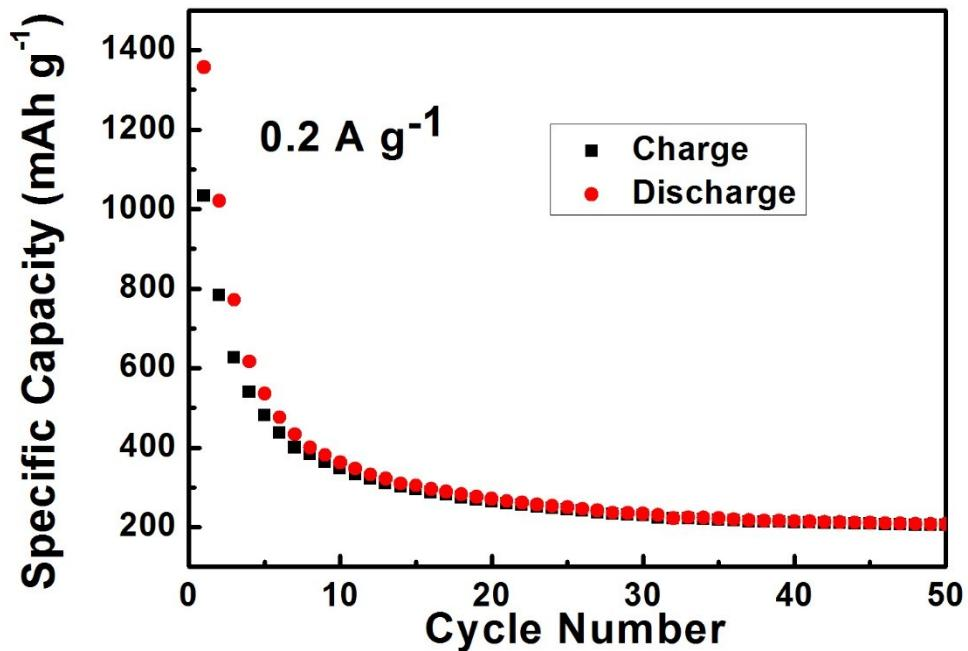
**Figure S6.** Cycling performance of  $\text{NiCo}_2\text{S}_4$ -P electrode at a current density of  $0.2 \text{ A g}^{-1}$
