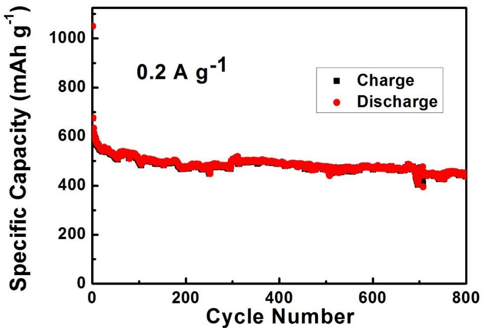
**Figure S5.** Cycling performance of  $\text{NiCo}_2\text{O}_4$ -G electrode at a current density of  $0.2 \text{ A g}^{-1}$
