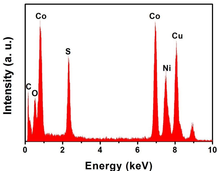
**Figure S1.** EDX spectrum of incompletely vulcanized  $\text{NiCo}_2\text{O}_4/\text{NiCo}_2\text{S}_4$  composite after a 1 h sulfidation reaction of the  $\text{NiCo}_2\text{O}_4$  precursor under  $\text{H}_2\text{S}/\text{Ar}$  atmosphere.
