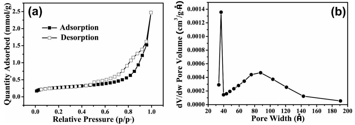
**Figure S3.** (a) Nitrogen adsorption–desorption isotherms and (b) pore size distribution of the mesoporous  $\text{NiCo}_2\text{S}_4$  nanosheets.
