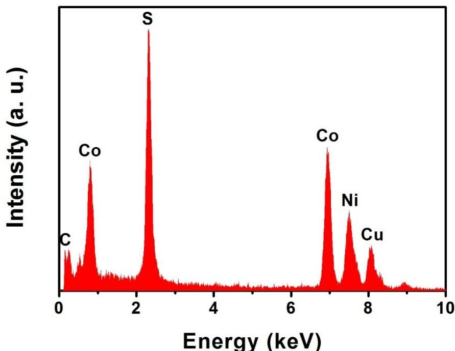
**Figure S2.** EDX spectrum of pure  $\text{NiCo}_2\text{S}_4$  nanosheets after a 3 h sulfidation reaction.
