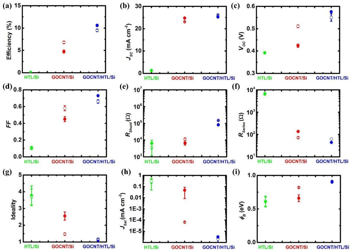
Fig. S3: The details of light and dark curves of spiro-OMeTAD/Si, GOCNT/Si and GOCNT/spiro-OMeTAD/Si devices, (a) Efficiency, (b)  $J_{sc}$ , (c)  $V_{oc}$ , (d) FF, (e)  $R_{shunt}$ , (f)  $R_{series}$ , (g) ideality, (h)  $J_{sat}$  and (i)  $\phi_B$  before (hollow points) and after (solid points)  $AuCl_3$  doping. In the devices in this figure, the T of GOCNT films is 77 % before  $AuCl_3$  and the thickness of spiro-OMeTAD layers is 90 nm. HTL stands for spiro-OMeTAD.
