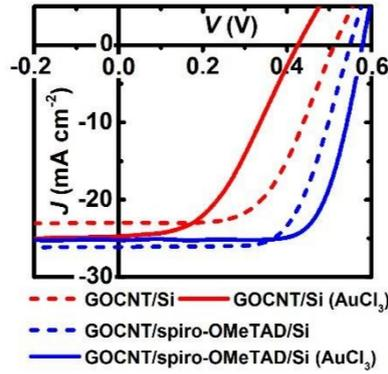
Fig. S4: J-V curves of GOCNT/Si and GOCNT/spiro-OMeTAD/Si before and after  $\text{AuCl}_3$  doping under light condition. Short dash and solid curves show the performance of the devices before and after  $\text{AuCl}_3$  doping respectively.
