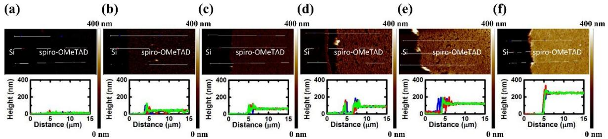
Fig. S5: AFM height images of spiro-OMeTAD films deposited on Si with different volumes of stock solution (a) 2.5  $\mu\text{L}$ , (b) 10  $\mu\text{L}$ , (c) 20  $\mu\text{L}$ , (d) 30  $\mu\text{L}$ , (e) 40  $\mu\text{L}$  and (f) 80  $\mu\text{L}$ .
