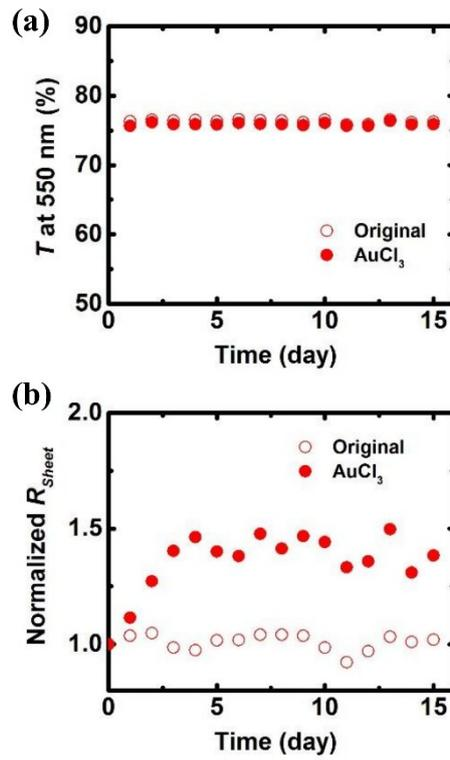
Fig. S8: Degradation of the performance (a)  $T$  and (b)  $R_{Sheet}$  of the GOCNT films. The hollow and solid data points are used to characterize the properties of the devices or films with and without AuCl<sub>3</sub> doping.
