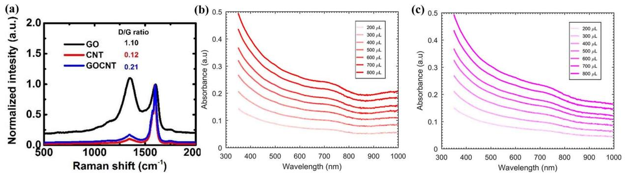
Fig. S2: (a) The Raman spectrum of pure GO, CNT and GOCNT films. (b,c) UV-Vis spectra of (b) GOCNT films and (c) GOCNT/AuCl<sub>3</sub> films created with varying volume of GOCNT suspension.
