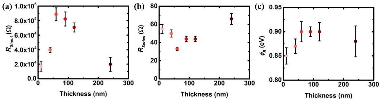
Fig. S6: The performance of  $\text{AuCl}_3$  doped GOCNT/spiro-OMeTAD/Si as a function of the thickness of the spiro-OMeTAD layer applied on the Si surface (a)  $R_{Shunt}$ , (b)  $R_{Series}$  and (c)  $\phi_B$ . The devices in this figure are made of GOCNT films with  $T$  of 77 % (measured before  $\text{AuCl}_3$ ) with spiro-OMeTAD layers of thicknesses ranging from 10 to 240 nm.
