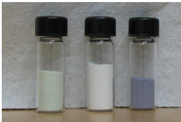
Figure S1. From left to right: \text{CuO}/\text{La}_2\text{O}_3/\text{TiO}_2 , \text{Ag}_2\text{O}/\text{La}_2\text{O}_3/\text{TiO}_2 and \text{Au}/\text{La}_2\text{O}_3/\text{TiO}_2 after calcination at 500^\circ\text{C} for two hrs.
