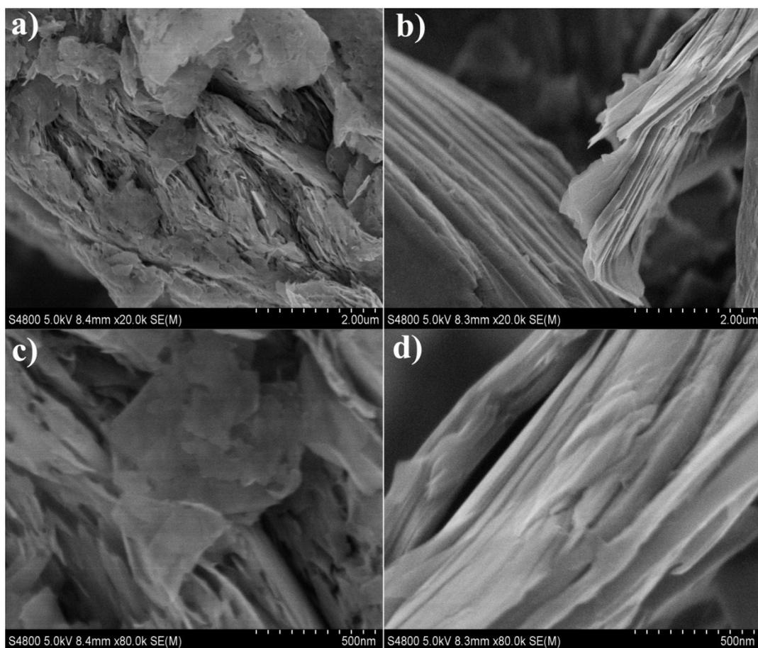
**Figure S4.** SEM images of S/G-DBD composite with 3 h synthesis time and different sulfur mass percentage of 60 % (a, c), 80% (b, d) in the precursor mixture.
