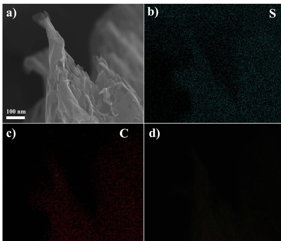
Figure S2. SEM image of S/G-DBD (a) and its corresponding element mappings of S (b), C (c), and hybrid element mapping (d).
