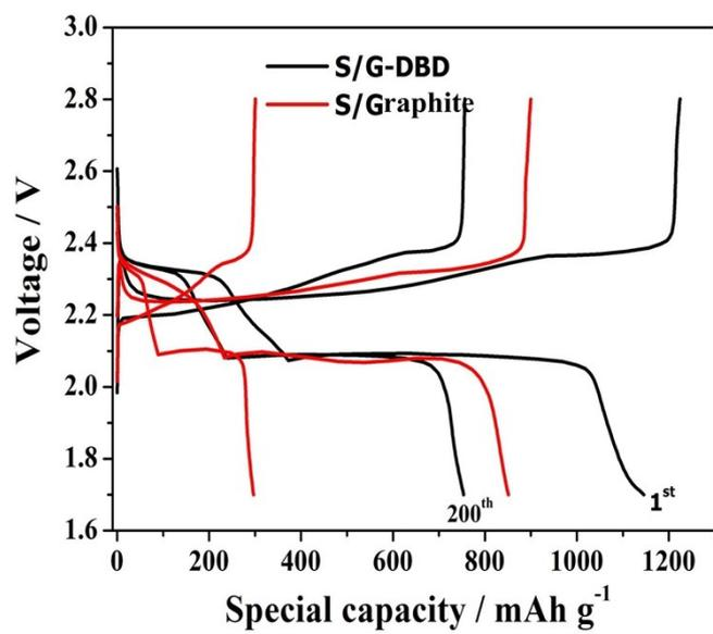
**Figure S6.** charge-discharge profiles of S/G-DBD and S/Graphite at 0.2 C.
