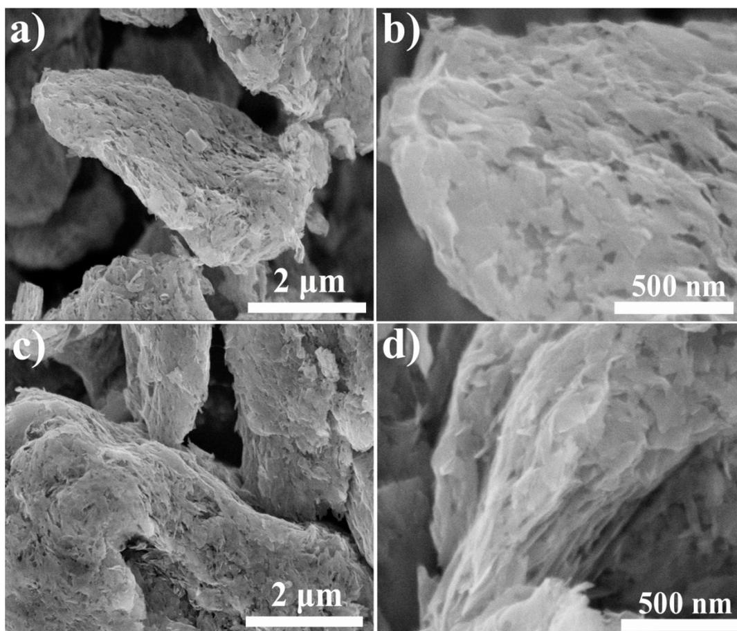
**Figure S3.** SEM images of (a, b) S/G-DBD2 and (c, d) S/G-DBD5 synthesized at the controlled time of 2 h and 5 h with sulfur mass percentage of 70 % in the precursor mixture.
