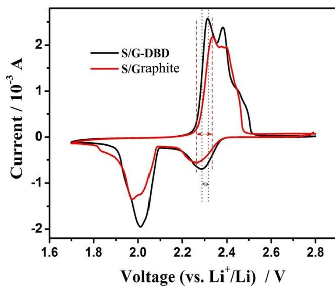
**Figure S5.** Cyclic voltammogram of S/G-DBD and S/Graphite with a scan rate of 0.1 mV s<sup>-1</sup> between 1.7 V and 2.8 V.
