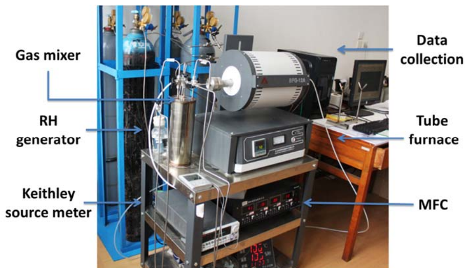
Figure S7. A photograph of the homemade setup for the humidity measurement (MFC: mass flow controller).
