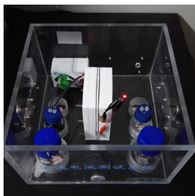
Fig. S8 Photograph of the S-KB@rGO suspension flow battery system.
