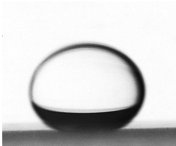
Figure S12. Image of a water droplet on the coated glass slide under oil, which still exhibits superhydrophobicity.
