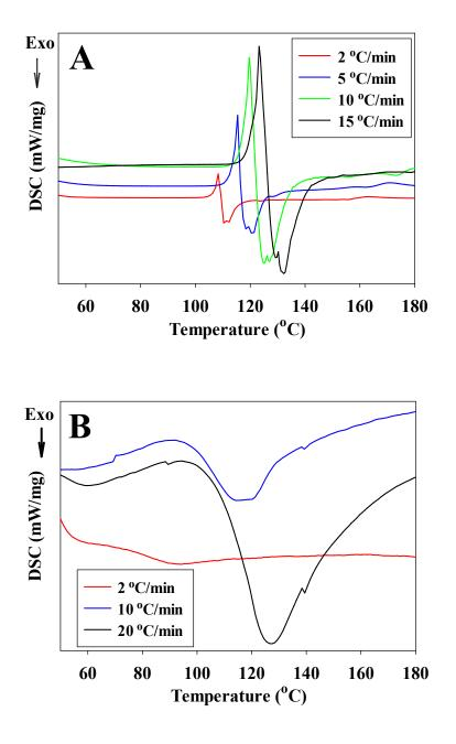
Fig. S1 DSC profiles for neat AB (A) and AB/CEMC (B) at various heating rate.
