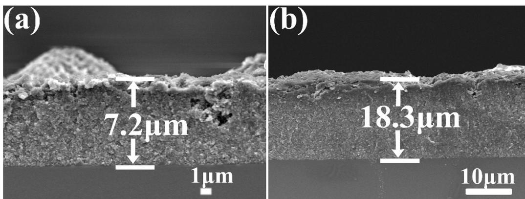
Figure S1. Coating thickness for (a) SiO<sub>2</sub>/PU (b) SiO<sub>2</sub>/epoxy resin on glass substrate.
