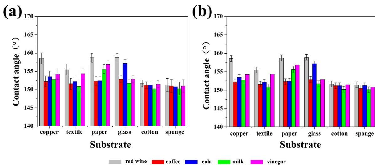
Figure S2. (a) Contact angles of different droplets on different substrates that were coated with (a) SiO<sub>2</sub>/PU and (b) SiO<sub>2</sub>/epoxy resin, respectively.
