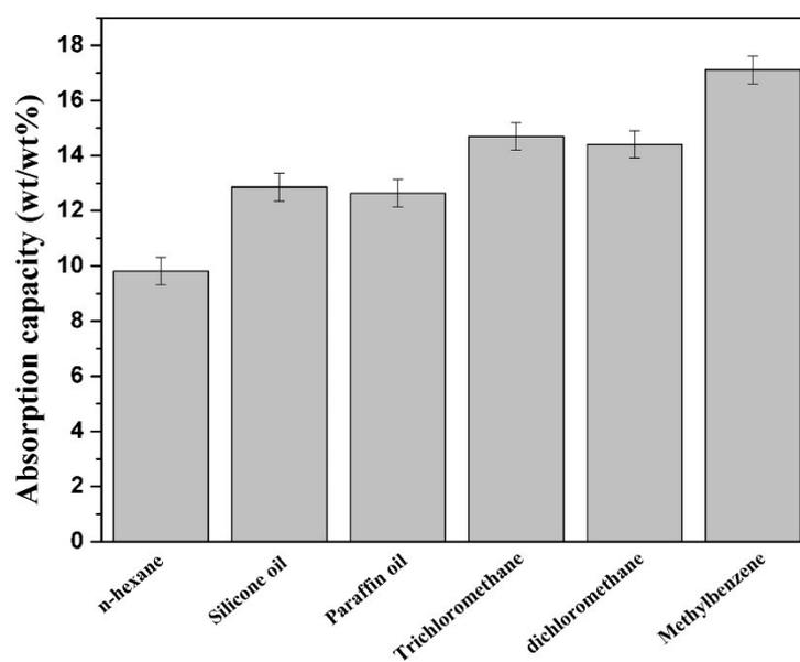
Figure S7. Absorption capacity of the superhydrophobic SiO<sub>2</sub>/PU sponge for different oils and organic solvents. The absorption capacity shows the weight of each solvent that can be collected in the sponge per gram of sponge.
