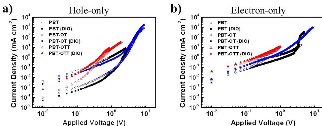
**Figure S5.** Dark current density versus effective voltage characteristics of a) hole-only devices and b) electron only devices, with photoactive layers of polymers: PC<sub>71</sub>BM (1:1.5, w/w) blends without DIO and with DIO additive. In the case of electron-only devices the  $V_{bi} = 1.5$  V is used.
