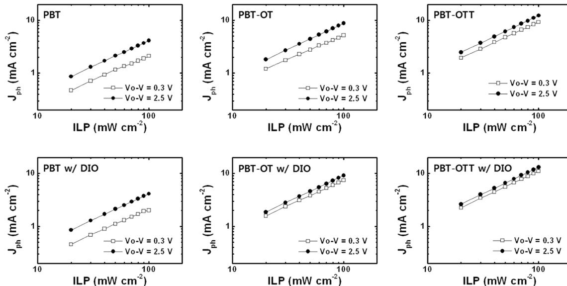
**Figure S6.** Incident light power-dependent photocurrent plots of OPVs for calculating S factors.
