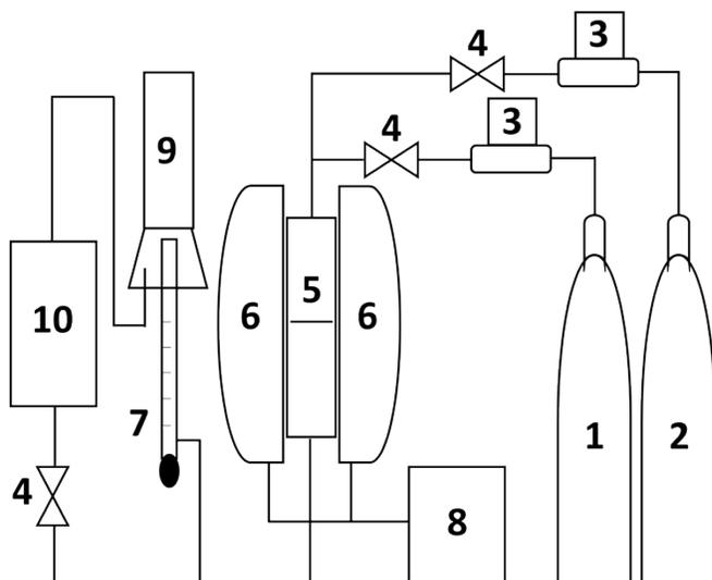
1: Nitrogen 2: Carbon dioxide 3: Mass flow controller 4: Valve
