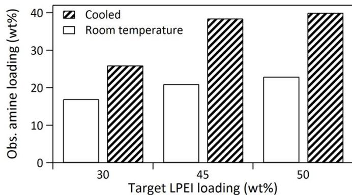
**Fig. S2** The impact of cooling stage on the observed PEI loadings. PEI loadings from the TGA increased because cooled amine is easily recovered from glassware.
