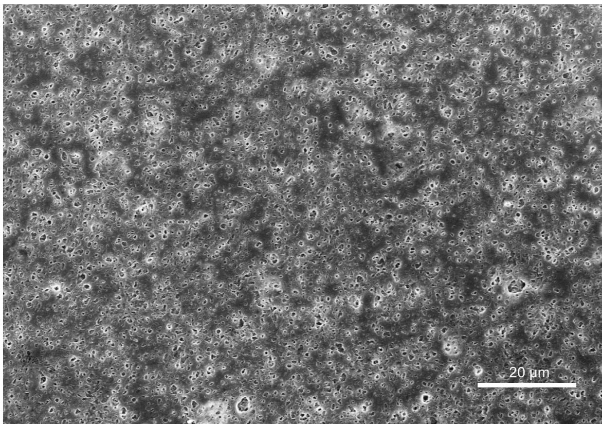
**Figure S2.** SEM image (top-view) of a piece of PVdF-HFP membrane shows the highly porous structure.
