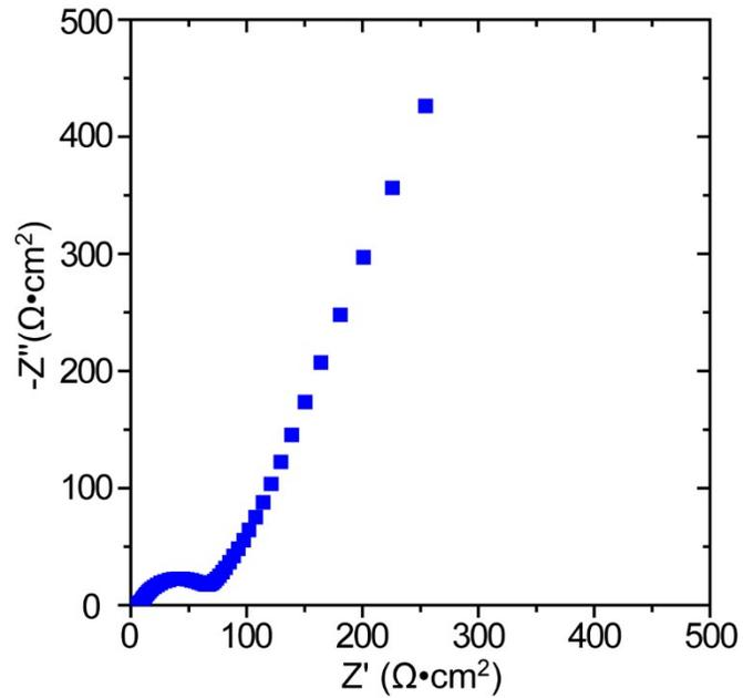
**Figure S1.** EIS curve of the integrated Al leaf/ LFP cathode in a half cell with lithium metal anode and PVdF-HFP gel electrolyte.
