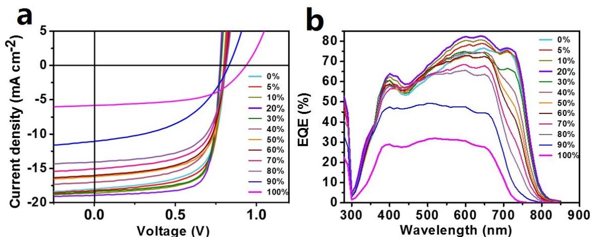
**Figure S1.** a)  $J$ - $V$  curves of ternary organic solar cells with different weight ratios of PDT2FBT-ID under AM 1.5 G illumination ( $100 \text{ mW cm}^{-2}$ ). b) The corresponding EQE spectra of ternary organic solar cells.
