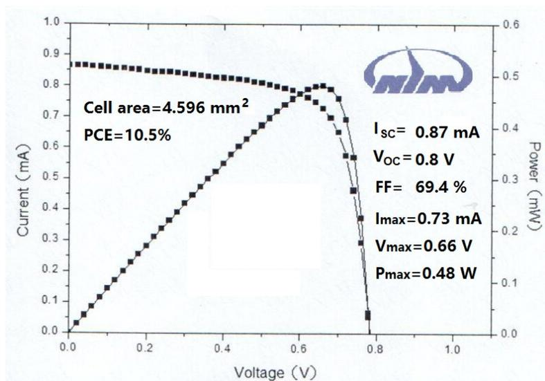
**Figure S9.** I-V curve and Power-V curve for certification.
