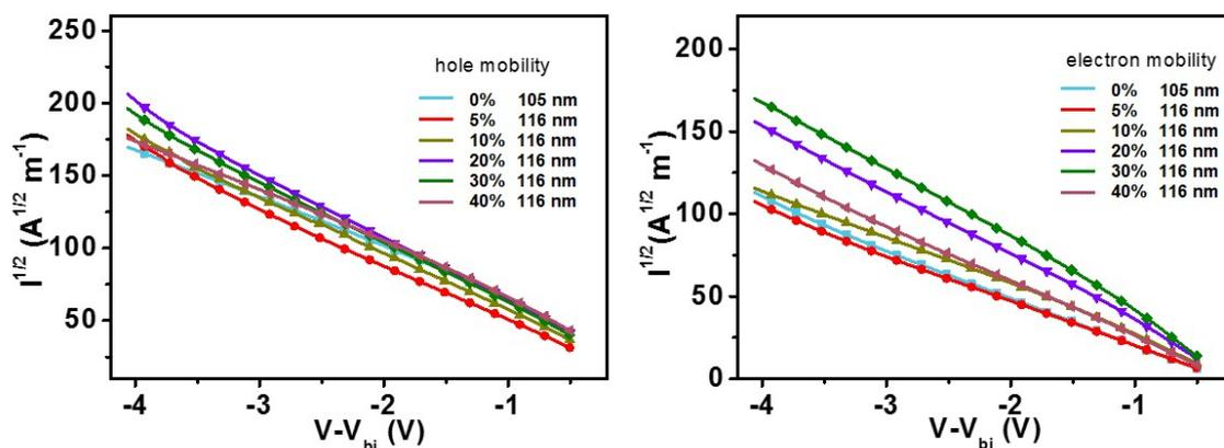
**Figure S4.** SCLC measured  $J^{1/2} - V - V_{bi}$  curves under dark condition for ternary active layers with different weight ratios of PDT2FBT-ID in CB solution, a) hole-only devices and b) electron-only devices.
