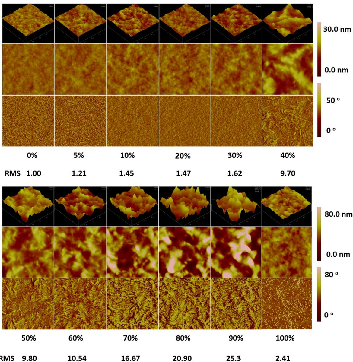
**Figure S6.** AFM topography images and phase images obtained in tapping mode of PTB7-Th:PDT2FBT-ID:PC<sub>71</sub>BM blend films with various weight ratio of PDT2FBT-ID.
