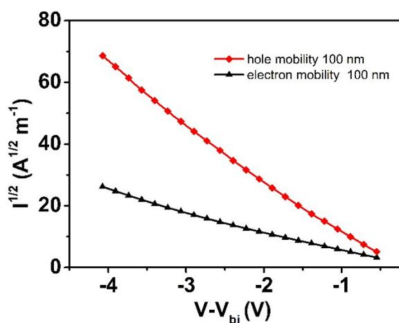
**Figure S5.** Hole and electron mobility of PDT2FBT-ID/PC<sub>71</sub>BM blend films from chloroform solution.
