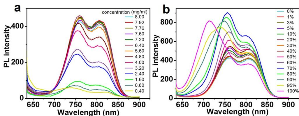
**Figure S2.** The photoluminescence properties of a) Referenced neat PTB7-Th films obtained from CB solution with different concentration. b) PTB7-Th/PDT2FBT-ID blend films obtained from CB solution with different doping ratio of PDT2FBT-ID, and the total concentration of PTB7-Th/PDT2FBT-ID is 8 mg/ml.
