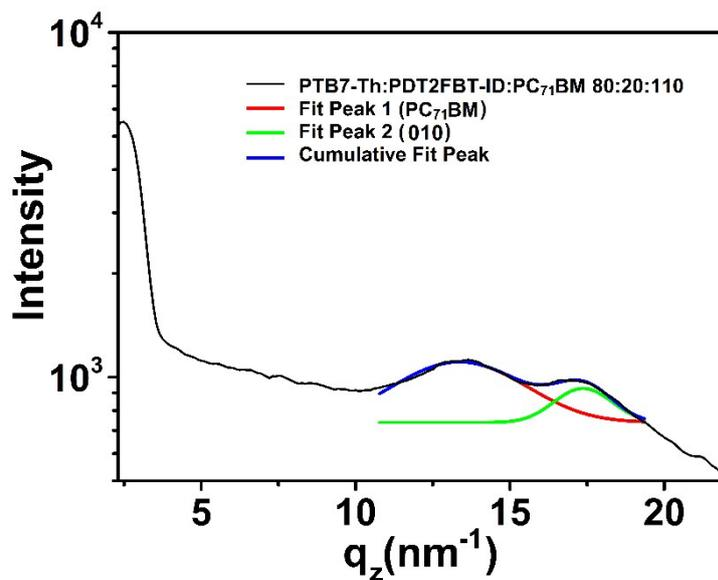
**Figure S8.** An example of Gaussian fitting for out-of-plane cut. The  $\pi$ - $\pi$  stacking distance and the FWHM of the  $\pi$ - $\pi$  stacking peak (010) were obtained from the fitting.
