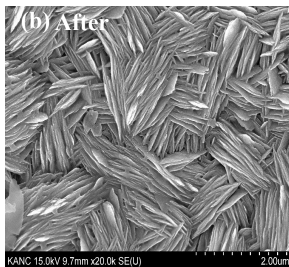
Fig. S9: (a) Chronoamperometry stability test measured at 1.77 V/RHE and (b) SEM image after the stability measurement of the CuO nanosheet electrode in a 0.2M borate buffer solution.
