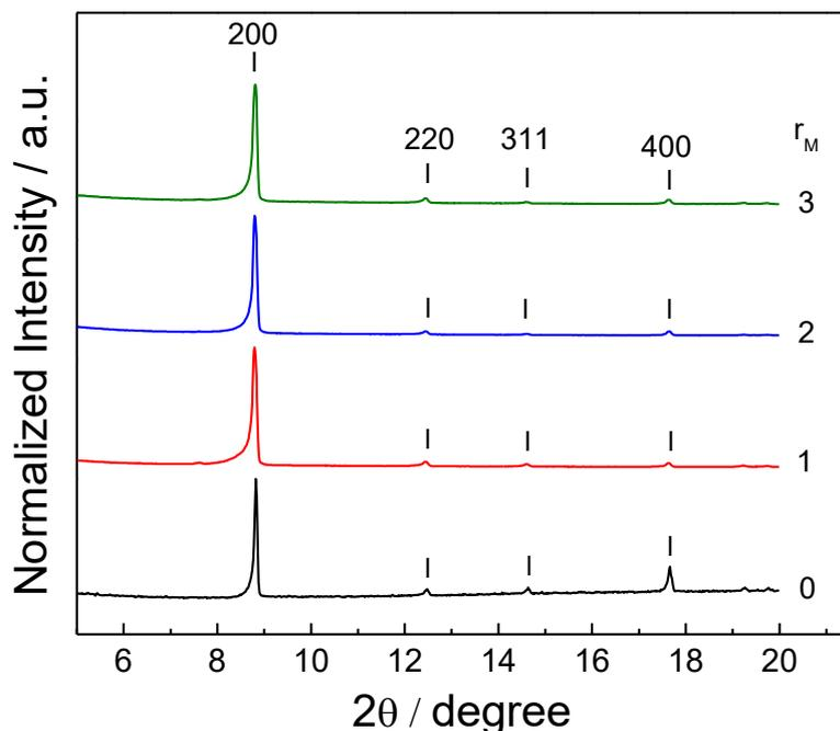
**Figure S30** XRD patterns of **Zn-DM** films fabricated at 40 °C via integration of coordination modulation with LPE fabrication process; using  $\text{Zn}_4\text{O}(\text{OAc})_6$  0.5 mM and  $\text{H}_2\text{DM}$  0.5 mM as precursor solutions, and acetic acid as coordination modulator by mixing it with the  $\text{H}_2\text{DM}$  solutions with various  $r_M$  ratio (corresponding with the growth data in Figure S29)
