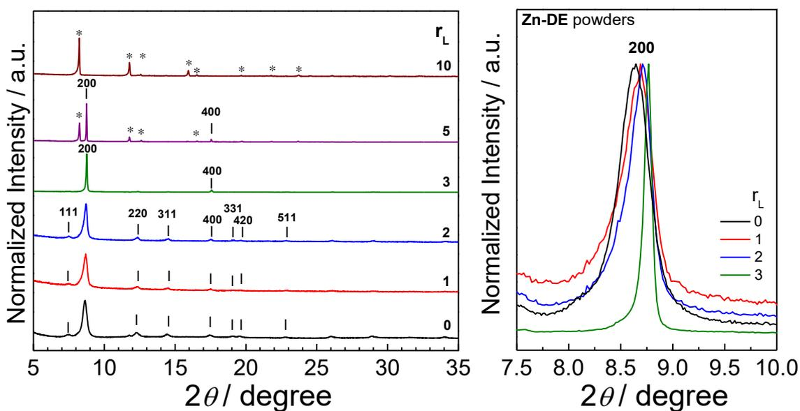
**Figure S3** Powder X-ray diffraction patterns for **Zn-DE** powders synthesized by combining coordination modulation with ligand replacement approach at 50 °C using acetic acid as the modulator with  $r_L = 0 - 10$ . The numbers in the figure indicate the Miller indices of the diffractions.
