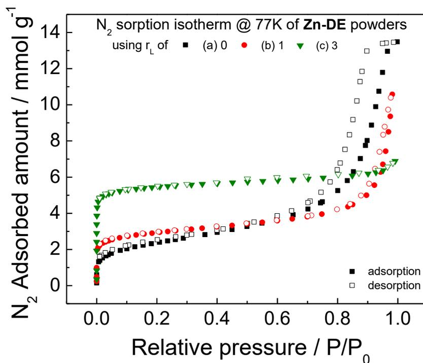
**Figure S9** N<sub>2</sub> sorption isotherm at 77 K of the Zn-DE powders synthesized at 50°C by integrating coordination modulation with the ligand replacement approach using  $r_L$  ratio of (a) 0, (b) 1 and (c) 3.
