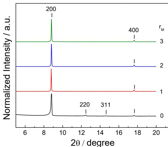
**Figure S14** Powder X-ray diffraction patterns (XRD) of Zn-ME films fabricated at 40 °C via integration of coordination modulation with LPE fabrication process; using  $Zn_4O(OAc)_6$  of (a) 0.5 mM and (b) 1.0 mM,  $H_2ME$  0.5 mM as precursor solutions and acetic acid as coordination modulator by mixing it with the  $Zn_4O(OAc)_6$  solutions with  $r_M = 0 - 3$ .
