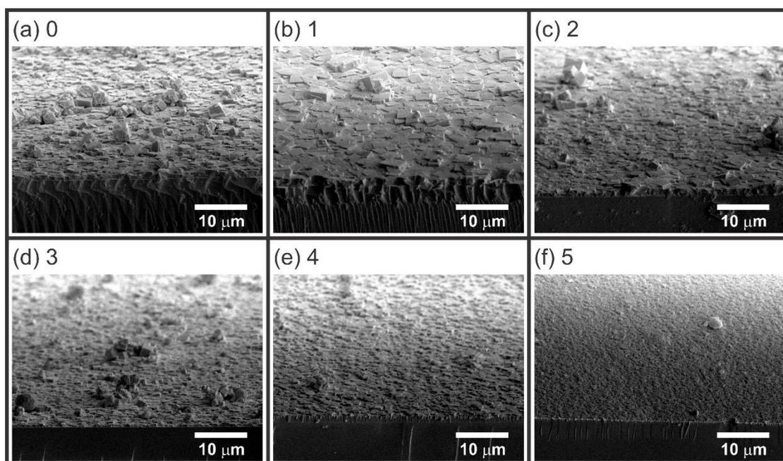
**Figure S11** Cross-sectional view SEM images of **Zn-DM** films fabricated at 40 °C via integration of coordination modulation with LPE fabrication process; using  $\text{Zn}_4\text{O}(\text{OAc})_6$  0.5 mM,  $\text{H}_2\text{DM}$  0.5 mM as precursor solutions and acetic acid as coordination modulator by mixing it with the  $\text{Zn}_4\text{O}(\text{OAc})_6$  solutions with  $r_M = 0 - 5$ .
