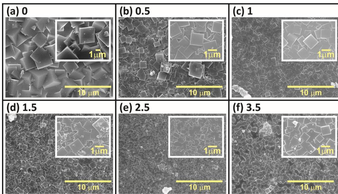
**Figure S27** SEM images of the surfaces of **Zn-DM** films fabricated at 40 °C with various  $r_M$  ratio via integration of coordination modulation with LPE fabrication process on the pre-deposited, self-seeding **Zn-DM** layer fabricated without using the modulator for 5 cycles.
