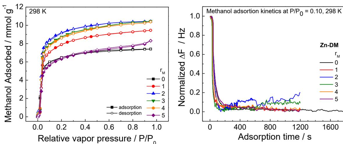
**Figure S12** Methanol sorption isotherms at 25 °C and adsorption kinetics at  $P/P_0 = 0.10$  measured using the environmentally controlled quartz crystal microbalance (QCM) of **Zn-DM** films fabricated at 40 °C via integration of coordination modulation with LPE fabrication process; using  $Zn_4O(OAc)_6$  0.5 mM,  $H_2DM$  0.5 mM as precursor solutions and acetic acid as coordination modulator by mixing it with the  $Zn_4O(OAc)_6$  solutions with  $r_M = 0 - 5$ .
