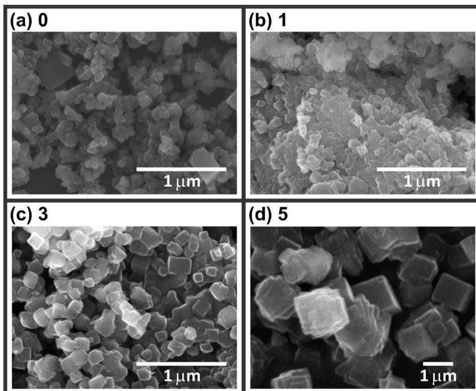
**Figure S4** Scanning electron microscopy (SEM) images of **Zn-DM** powders synthesized at 50°C by (a) ligand replacement approach without using the modulator ( $r_L = 0$ ) comparing with **Zn-DM** powders synthesized by integrating coordination modulation into the procedure using acetic acid as the modulator with  $r_L$  of (b) 1, (c) 3 and (d) 5.
