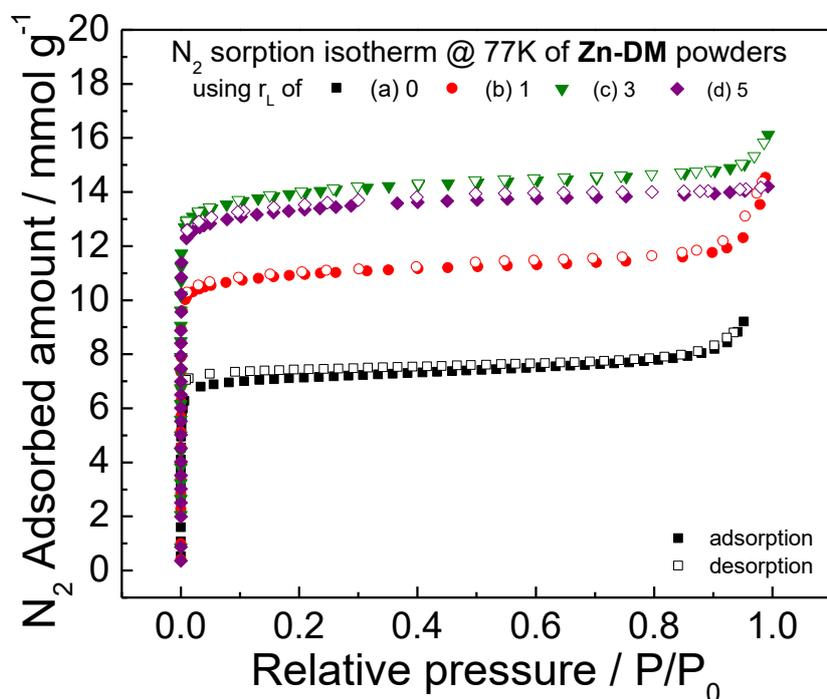
**Figure S7**  $N_2$  sorption isotherm at 77 K of the **Zn-DM** powders synthesized at 50°C by integrating coordination modulation with the ligand replacement approach using  $r_L$  ratio of (a) 0, (b) 1, (c) 3 and (d) 5.
