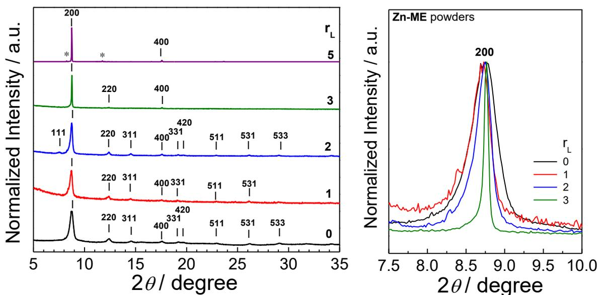
**Figure S2** Powder X-ray diffraction patterns for **Zn-ME** powders synthesized by combining coordination modulation with ligand replacement approach at 50 °C using acetic acid as the modulator with  $r_L = 0 - 5$ . The numbers in the figure indicate the Miller indices of the diffractions.
