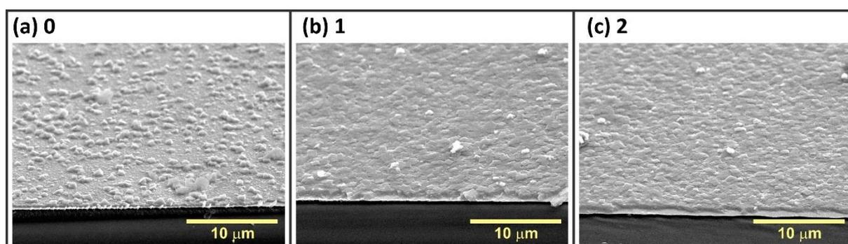
**Figure S21** Cross-sectional view SEM images of **Zn-DE** films fabricated at 40 °C via integration of coordination modulation with LPE fabrication process using  $r_M = 0 - 3$ .
