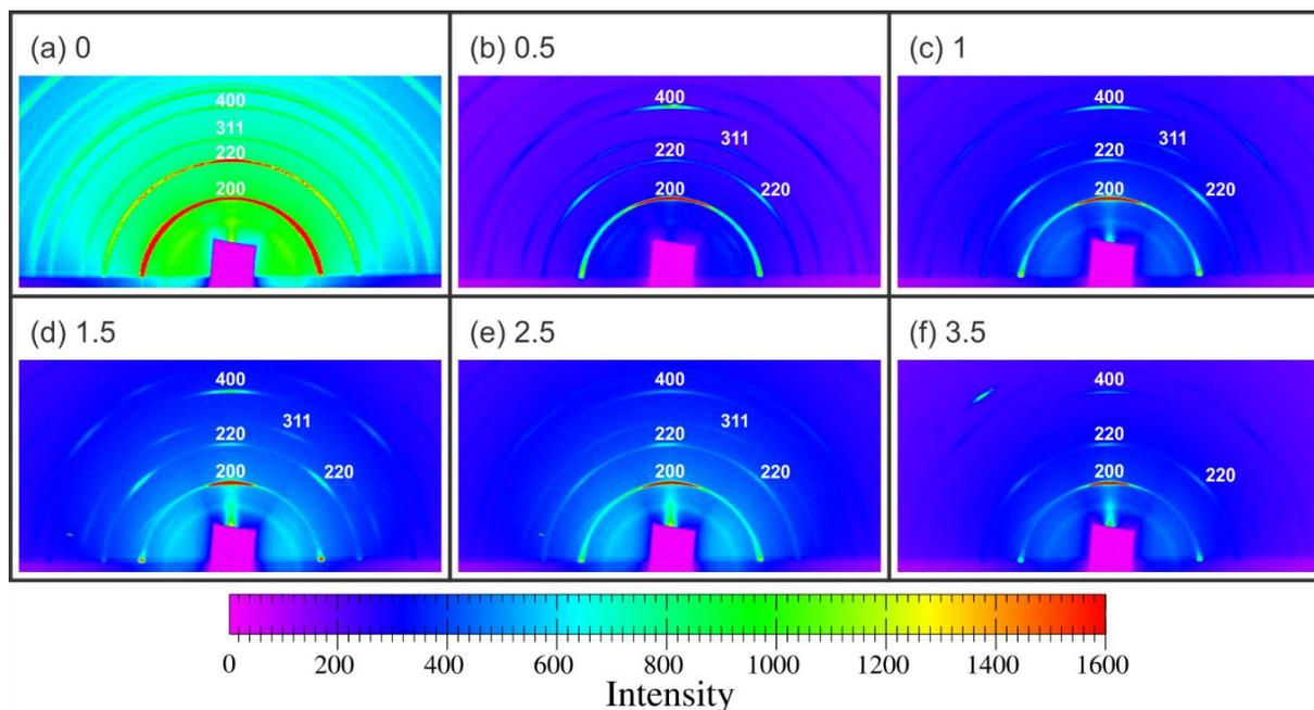
**Figure S26** GIXRD patterns of **Zn-DM** films fabricated at 40 °C with various  $r_M$  ratio by employing coordination modulation method in conjunction with LPE process on the pre-deposited, self-seeding **Zn-DM** layer fabricated without using the modulator for 5 cycles. Synchrotron parameters are X-ray wavelength 1.0013 Å, incidence angle 0.6° and refined sample-to-detector distance 487.3 mm.
