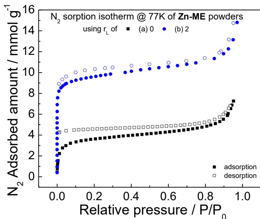
**Figure S8** N<sub>2</sub> sorption isotherm at 77 K of the Zn-ME powders synthesized at 50°C by integrating coordination modulation with the ligand replacement approach using  $r_L$  ratio of (a) 0 and (b) 2.
