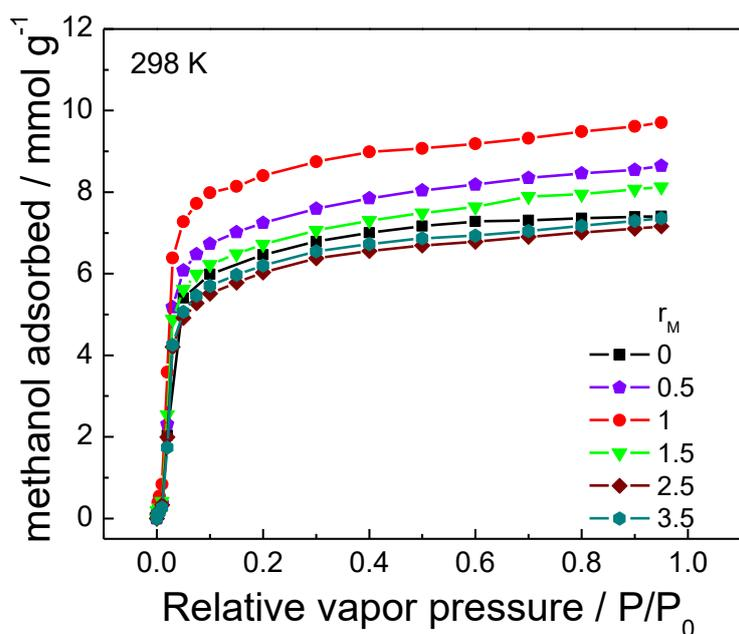
**Figure S28** Methanol adsorption isotherms at 25 °C using the environmentally controlled quartz crystal microbalance (QCM) of **Zn-DM** films fabricated at 40 °C with various  $r_M$  ratio via integration of coordination modulation with LPE fabrication process on the self-seeding **Zn-DM** layer fabricated without using the modulator for 5 cycles
