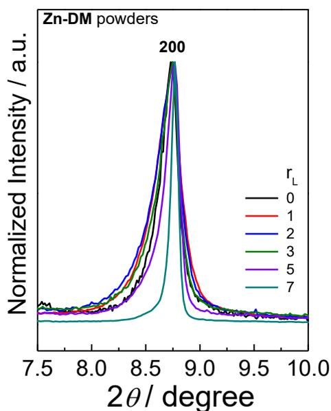
**Figure S1** Powder X-ray diffraction patterns for **Zn-DM** powders synthesized by combining coordination modulation with ligand replacement approach at 50 °C using acetic acid as the modulator with various modulator-to-linker molar ratio ( $r_L$ ) ranging from 1 to 30 comparing with the **Zn-DM** powder synthesized by ligand replacement approach without using the modulator. The numbers in the figure indicate the Miller indices of the diffractions.
