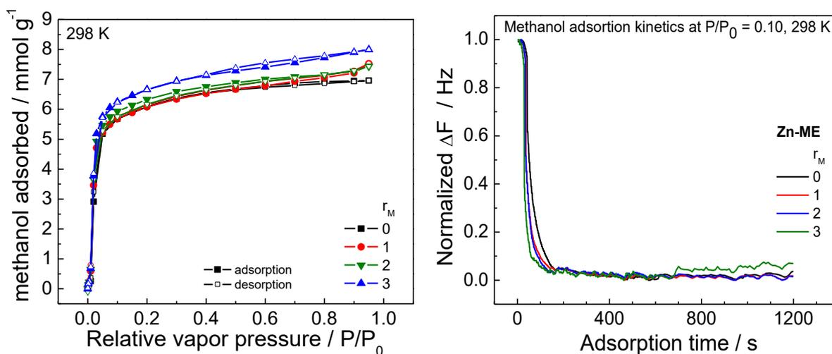
**Figure S18** Methanol sorption isotherms at 25 °C and adsorption kinetics at  $P/P_0 = 0.10$  measured using the environmentally controlled quartz crystal microbalance (QCM) of **Zn-ME** films fabricated at 40 °C via integration of coordination modulation with LPE fabrication process; using  $Zn_4O(OAc)_6$  0.5 mM,  $H_2DM$  0.5 mM as precursor solutions and acetic acid as coordination modulator by mixing it with the  $Zn_4O(OAc)_6$  solutions with  $r_M = 0 - 3$ .
