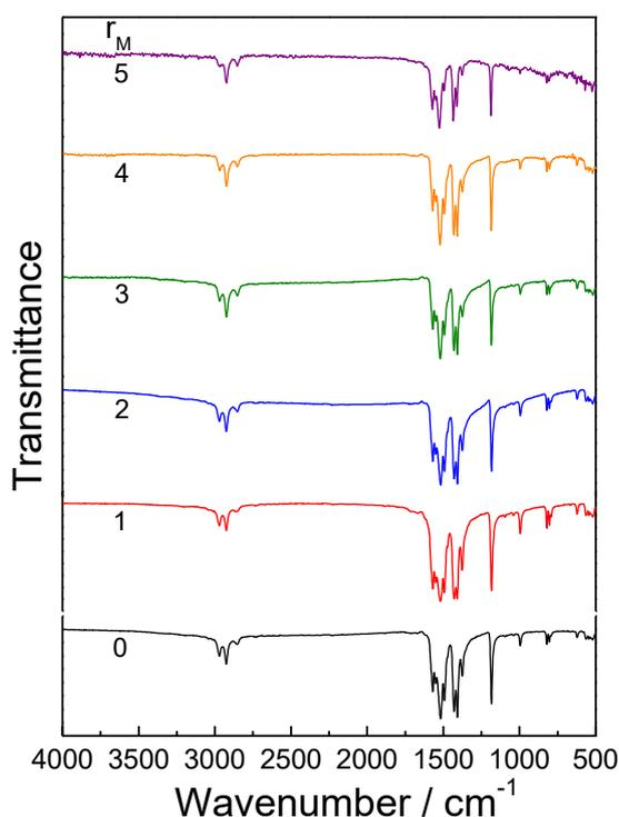
**Figure S13** Infrared reflection absorption spectra (IRRAS) of **Zn-DM** films fabricated at 40 °C via integration of coordination modulation with LPE fabrication process; using  $Zn_4O(OAc)_6$  0.5 mM,  $H_2DM$  0.5 mM as precursor solutions and acetic acid as modulator by mixing it with the  $Zn_4O(OAc)_6$  solutions with  $r_M = 0 - 5$ .
