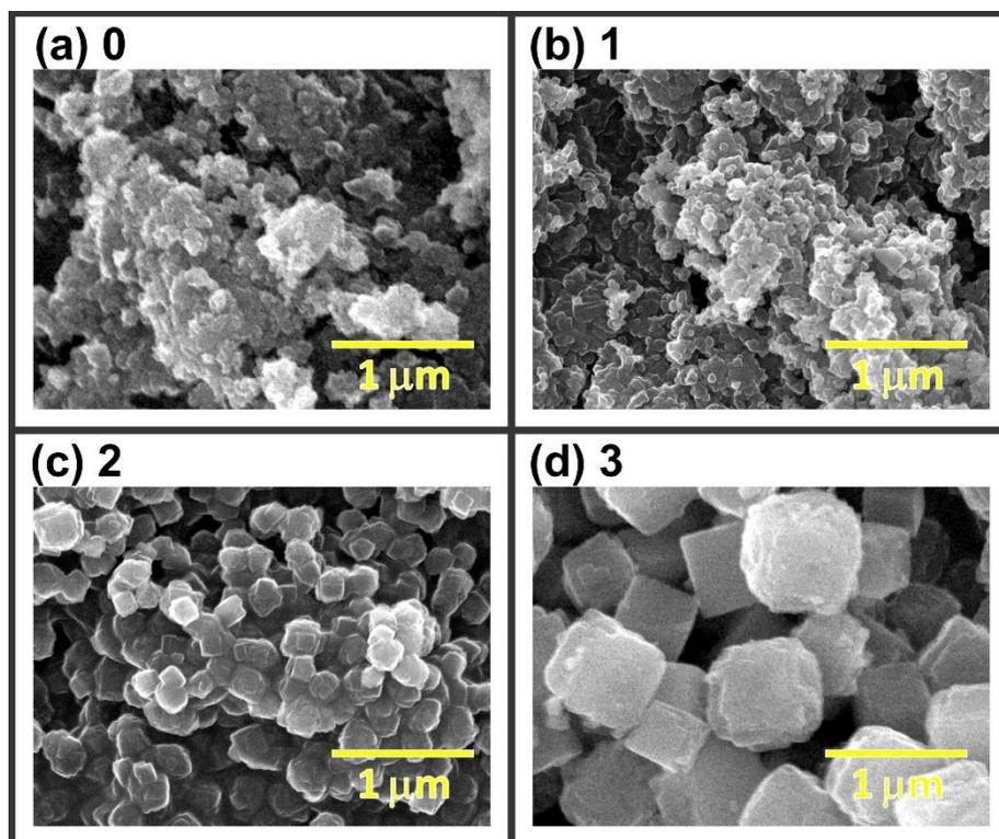
**Figure S5** Scanning electron microscopy (SEM) images of **Zn-ME** powders synthesized at 50°C by (a) ligand replacement approach without using the modulator ( $r_L = 0$ ) comparing with **Zn-ME** powders synthesized by integrating coordination modulation into the procedure using acetic acid as the modulator with  $r_L$  of (b) 1, (c) 2 and (d) 3.
