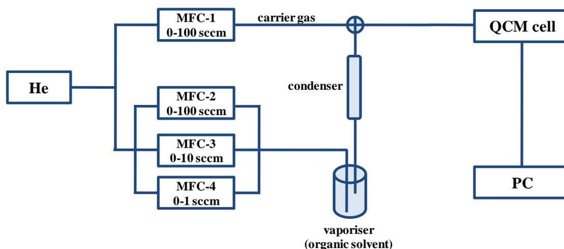
**Scheme S1** Schematic experimental setup of an environmental controlled quartz crystal microbalance (BEL-QCM) used for organic vapor adsorption experiments of MOF thin films
