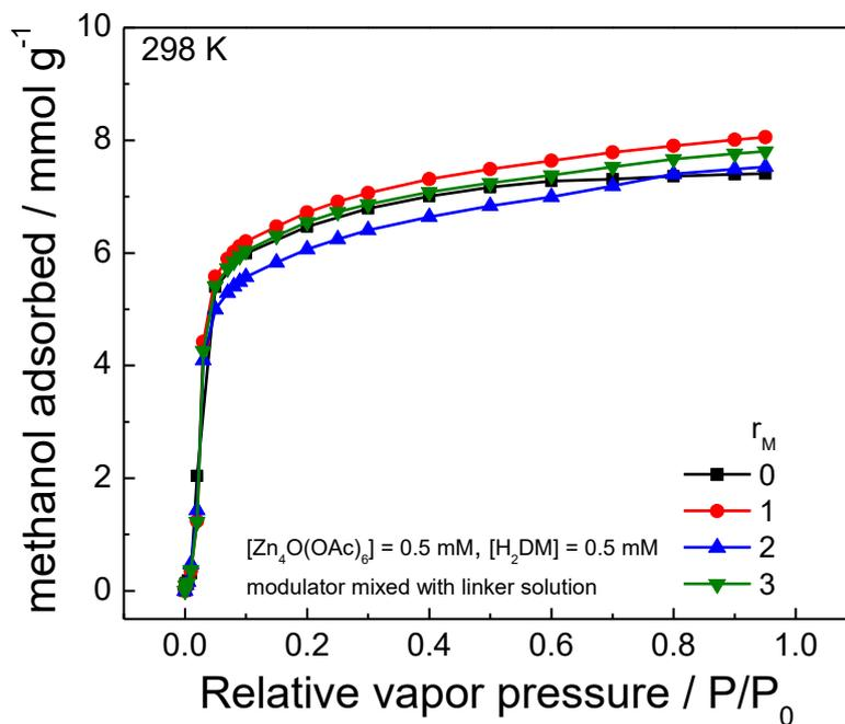
**Figure S31** Methanol adsorption isotherms at 25 °C using the environmentally controlled quartz crystal microbalance (QCM) of **Zn-DM** films fabricated at 40 °C via integration of coordination modulation with LPE fabrication process without self-seeding layer; using  $\text{Zn}_4\text{O}(\text{OAc})_6$  0.5 mM and  $\text{H}_2\text{DM}$  0.5 mM as precursor solutions and acetic acid as coordination modulator by mixing it with the  $\text{H}_2\text{DM}$  solution with various  $r_M$  ratio
