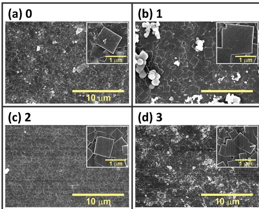
**Figure S20** SEM images of the surfaces of **Zn-DE** films fabricated at 40 °C via integration of coordination modulation with LPE fabrication process; using  $\text{Zn}_4\text{O}(\text{OAc})_6$  0.5 mM,  $\text{H}_2\text{DE}$  0.5 mM and acetic acid as coordination modulator by mixing it with the  $\text{Zn}_4\text{O}(\text{OAc})_6$  solutions with  $r_M = 0 - 3$ .
