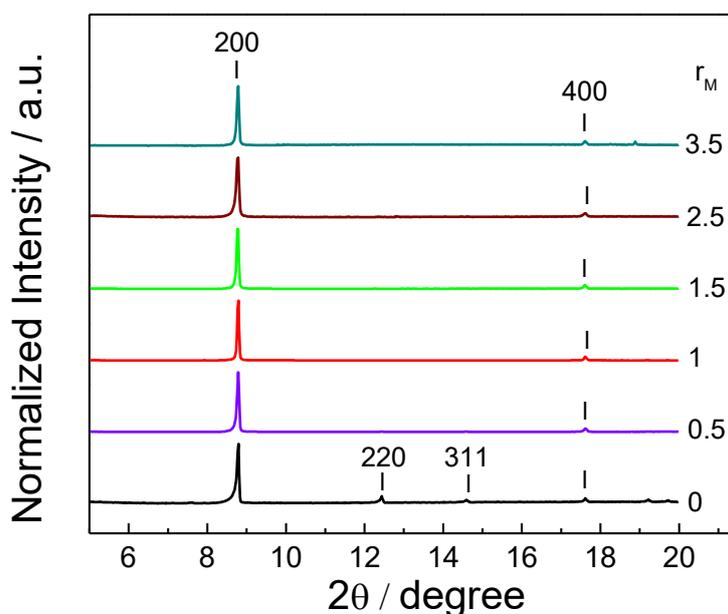
**Figure S25** XRD patterns of **Zn-DM** films fabricated at 40 °C with various  $r_M$  ratio via integration of coordination modulation with LPE fabrication process on the pre-deposited, self-seeding **Zn-DM** layer fabricated without using the modulator for 5 cycles (corresponding with the growth data in Figure S24)
