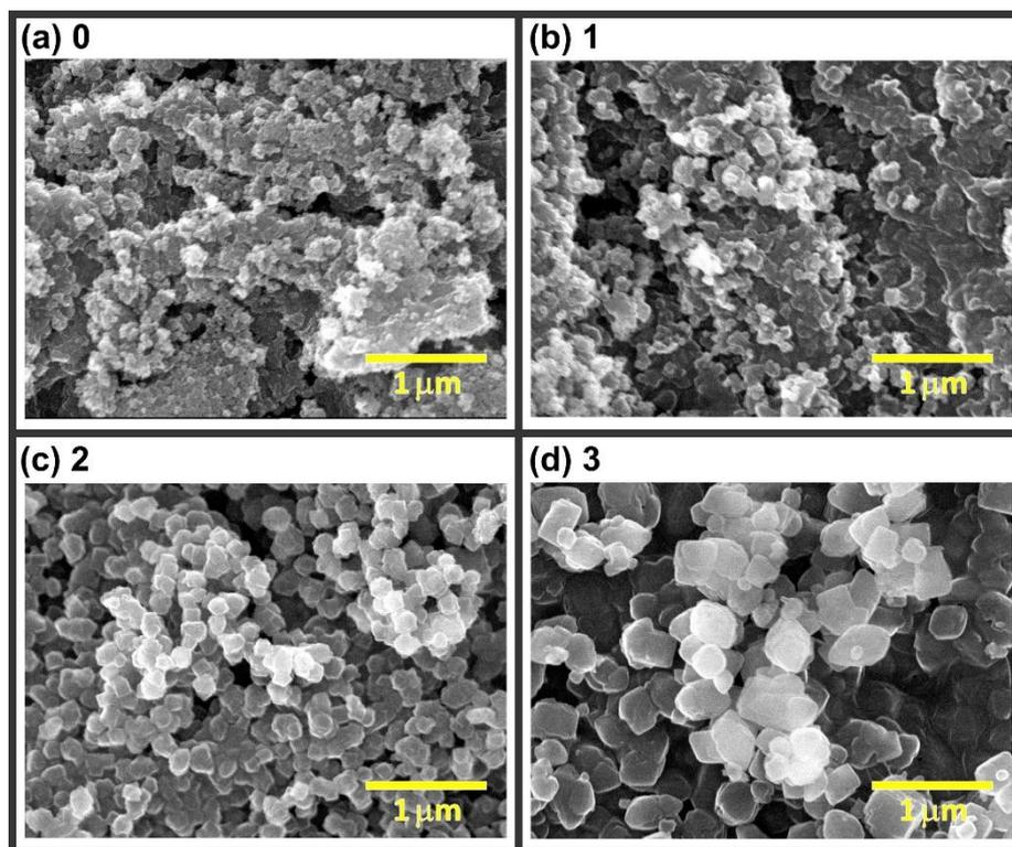
**Figure S6** Scanning electron microscopy (SEM) images of **Zn-DE** powders synthesized at 50°C by (a) ligand replacement approach without using the modulator ( $r_L = 0$ ) comparing with **Zn-DE** powders synthesized by integrating coordination modulation into the procedure using acetic acid as the modulator with  $r_L$  of (b) 1, (c) 2 and (d) 3.
