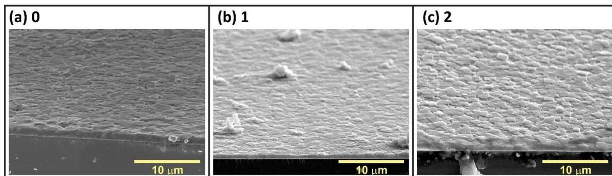
**Figure S16** Cross-sectional view SEM images of **Zn-ME** films fabricated at 40 °C via integration of coordination modulation with LPE fabrication process using  $r_M = 0 - 3$ .
