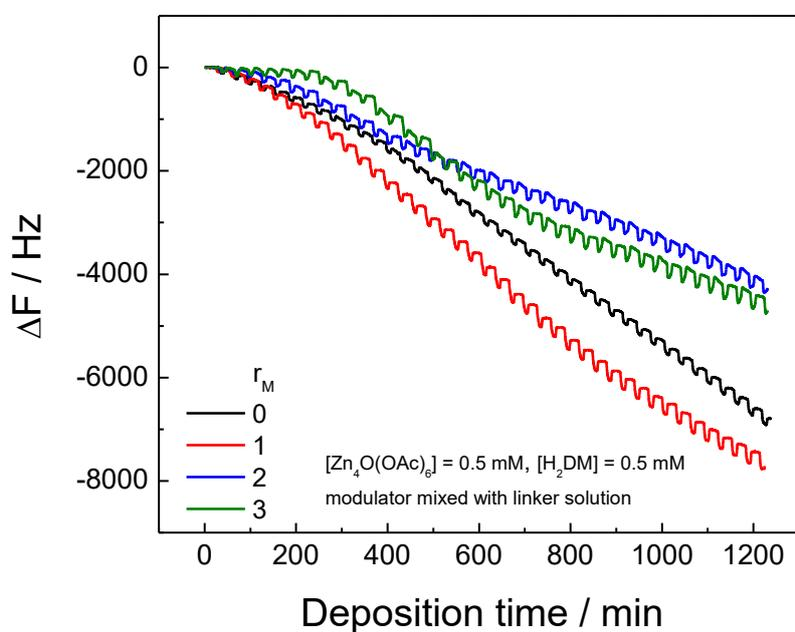
**Figure S29** In-situ monitoring of QCM frequency during the fabrication of **Zn-DM** films at 40 °C via integration of coordination modulation with LPE fabrication process without seeding layer; using  $Zn_4O(OAc)_6$  0.5 mM and  $H_2DM$  0.5 mM as precursor solutions, and acetic acid as coordination modulator by mixing it with the  $H_2DM$  solutions with various  $r_M$  ratio
