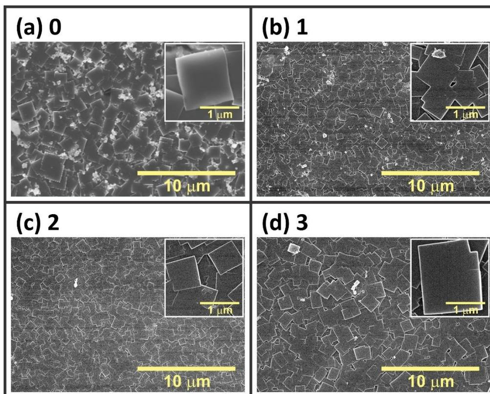
**Figure S15** SEM images of the surfaces of Zn-ME films fabricated at 40 °C via integration of coordination modulation with LPE fabrication process; using  $Zn_4O(OAc)_6$  0.5 mM,  $H_2ME$  0.5 mM and acetic acid as coordination modulator by mixing it with the  $Zn_4O(OAc)_6$  solutions with  $r_M = 0 - 3$ .
