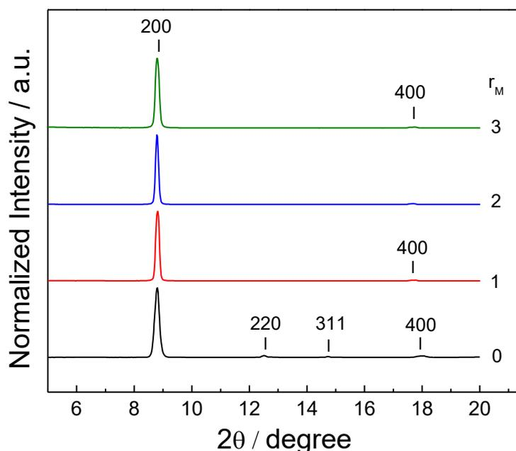
**Figure S19** Powder X-ray diffraction patterns (XRD) of **Zn-DE** films fabricated at 40 °C via integration of coordination modulation with LPE fabrication process; using  $Zn_4O(OAc)_6$  of (a) 0.5 mM and (b) 1.0 mM,  $H_2DE$  0.5 mM as precursor solutions and acetic acid as coordination modulator by mixing it with the  $Zn_4O(OAc)_6$  solutions with  $r_M = 0 - 3$ .
