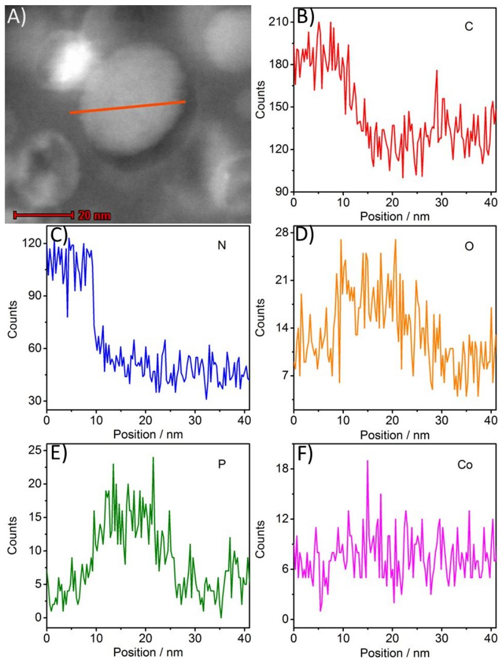
**Fig. S7** A) STEM image of VB-Na-500. B-F) The C, N, O, P and Co elemental-linear images of the orange line in A).
