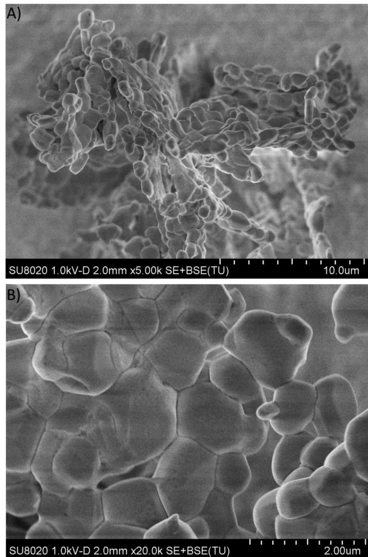
**Fig. S1** Typical SEM images of freeze-dried VB-NaCl assemble.
