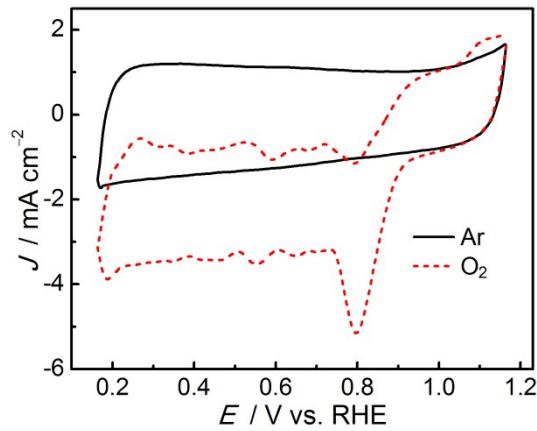
**Fig. S17** CV curves of MPC-900 in Ar- and  $\text{O}_2$ -saturated 0.1 M KOH aqueous solution with a scan rate of  $50 \text{ mV s}^{-1}$ .
