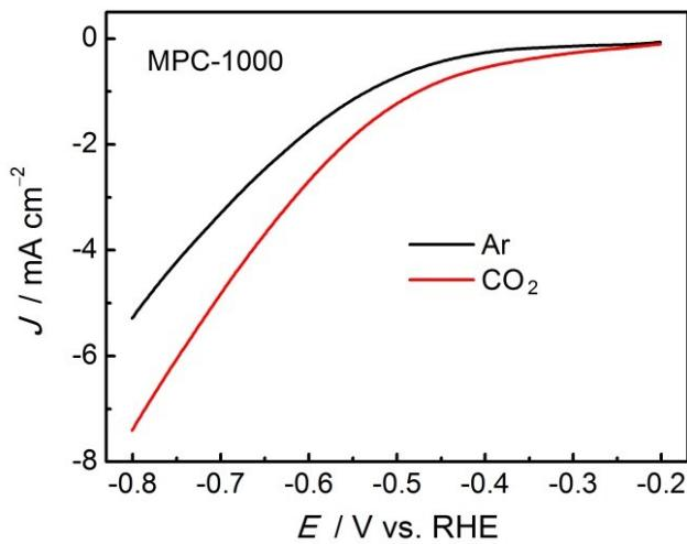
**Fig. S19** LSV curves of MPC-1000 in Ar- and CO<sub>2</sub>-saturated 0.1 M KHCO<sub>3</sub> solution with scan rate of 5 mV s<sup>-1</sup>.
