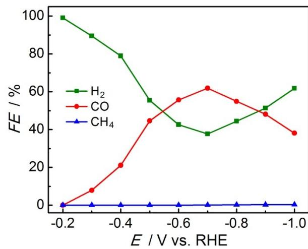
**Fig. S20** FE of MPC-1000 for H<sub>2</sub>, CO, and CH<sub>4</sub> at different applied potentials in CO<sub>2</sub>-staurated 0.1 M KHCO<sub>3</sub>.
