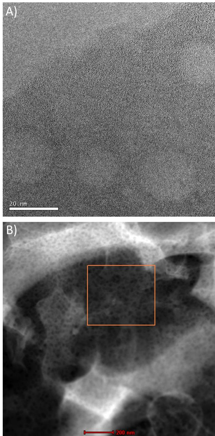
**Fig. S2** A) Magnified TEM image and B) STEM image of MPC-900.
