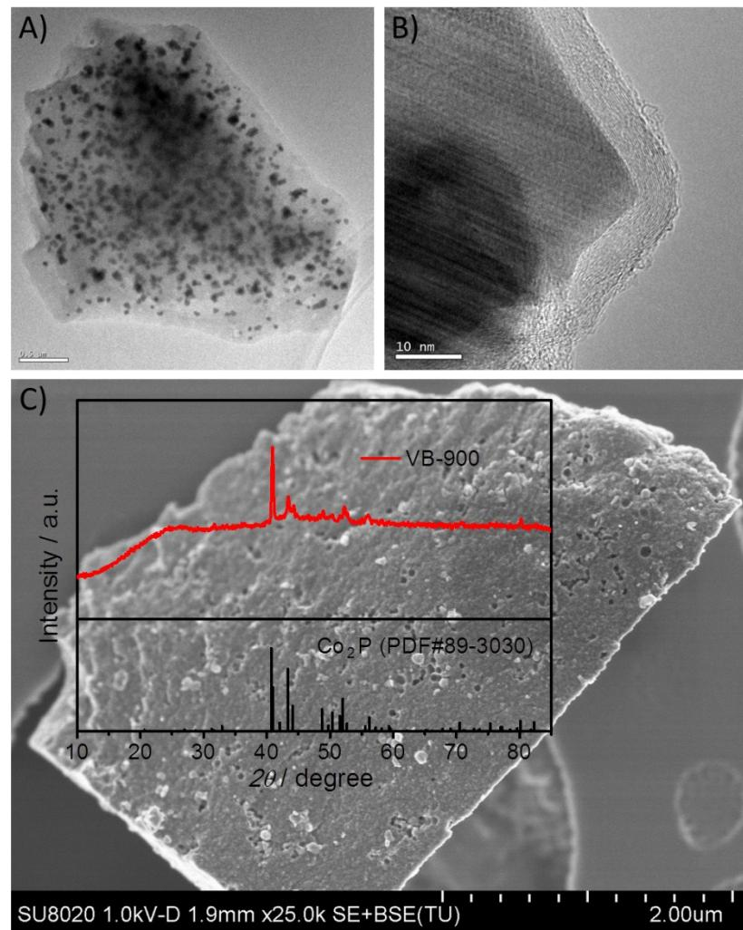
**Fig. S3** A) TEM, B) HRTEM and C) SEM images of VB-900. Insert of C) is XRD pattern of VB-900.
