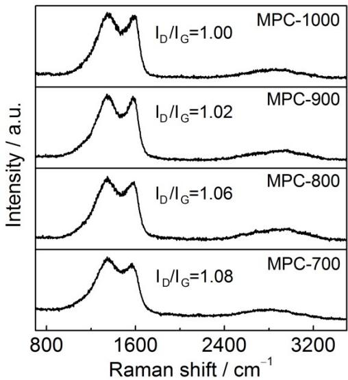
**Fig. S14** Raman spectra of MPCs. It is observed that the value of ID/IG for MPCs decrease significantly when annealing temperature above 900 °C, suggesting that the graphitization degree is enhanced.
