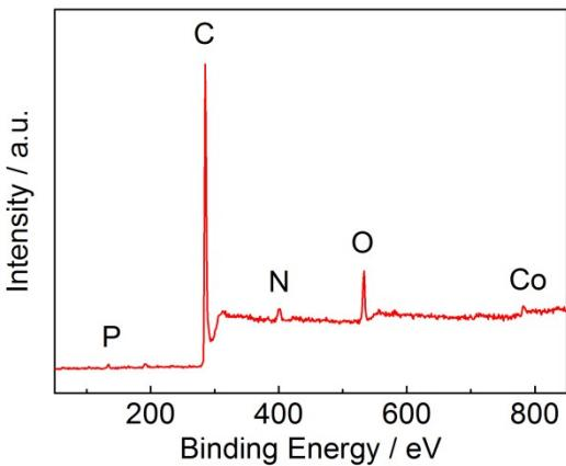
**Fig. S15** XPS survey spectra of MPC-900.
