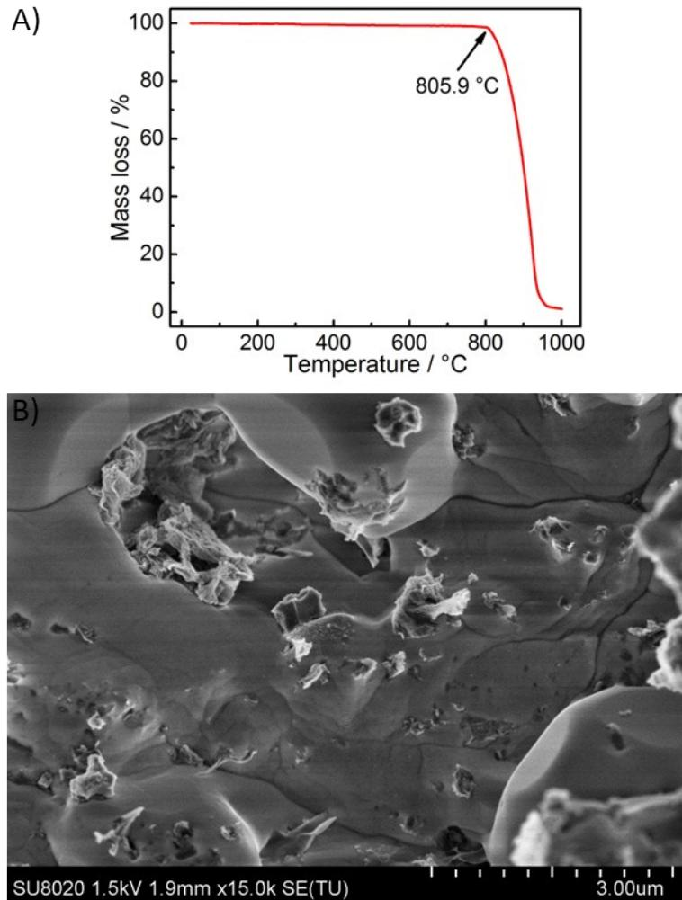
**Fig. S13** A) TGA curve of VB-NaCl. B) SEM image and photograph (inset of B) of MPC-900 before removing of NaCl. This morphology indicates that MPC-900 is sealed inside in NaCl molten salts.
