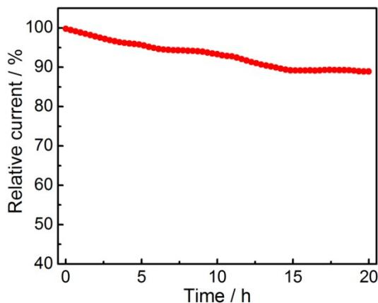
**Fig. S18** Chronoamperometric responses for ORR durability evaluation on MPC-900 electrode with the rotation rate of 1600 rpm at 0.76 V in O<sub>2</sub>-saturated 0.1 M KOH solution.
