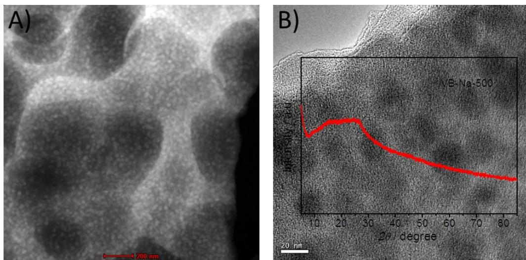
**Fig. S6** A) STEM and B) TEM images of VB-Na-500. Insert of B) is the XRD pattern of VB-Na-500.
