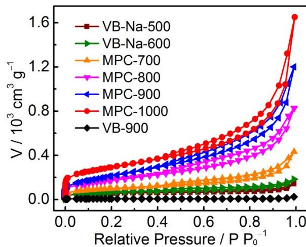
**Fig. S12** N<sub>2</sub> adsorption/desorption isotherms and VB-900, VB-Na-X and MPCs.
