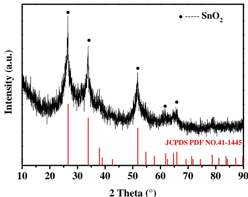
Fig. S2 XRD pattern of  $\text{SnO}_2/3\text{DC}$
