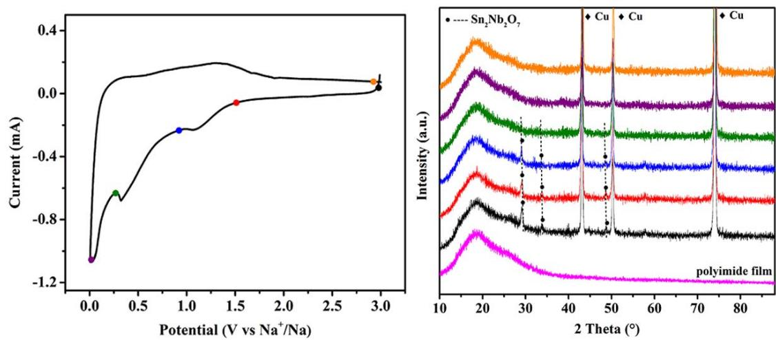
Fig. S12 Ex-situ XRD patterns obtained at different state of the first discharge-charge process to understand the structural change of M-Sn<sub>2</sub>Nb<sub>2</sub>O<sub>7</sub>/SnO<sub>2</sub>@3DC electrode
