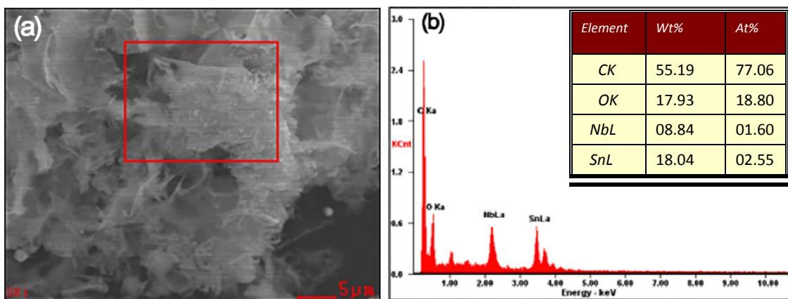
Fig. S4 (a) Low-magnified SEM image of as-synthesized  $\text{SnO}_2/\text{Sn}_2\text{Nb}_2\text{O}_7@3\text{DC}$ ; (b) EDX spectrum of red wire frame area in (a).
