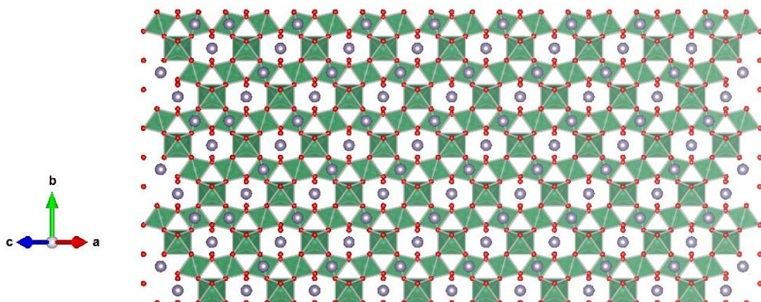
Fig. S1 Typical crystal structure of  $\text{Sn}_2\text{Nb}_2\text{O}_7$  looking from the crystal direction of [101].
