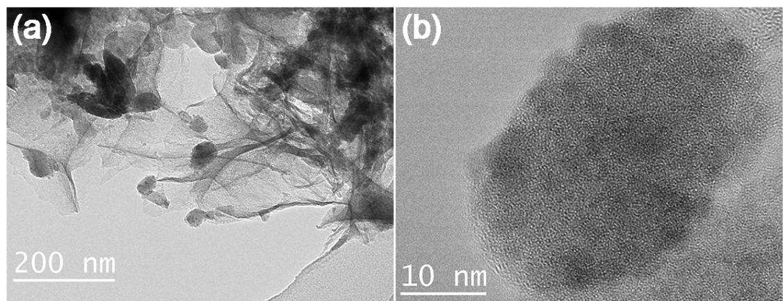
Fig. S14 (a) TEM image and (b) HRTEM image of M-Sn<sub>2</sub>Nb<sub>2</sub>O<sub>7</sub>/SnO<sub>2</sub>@3DC electrode after rate performance test.
