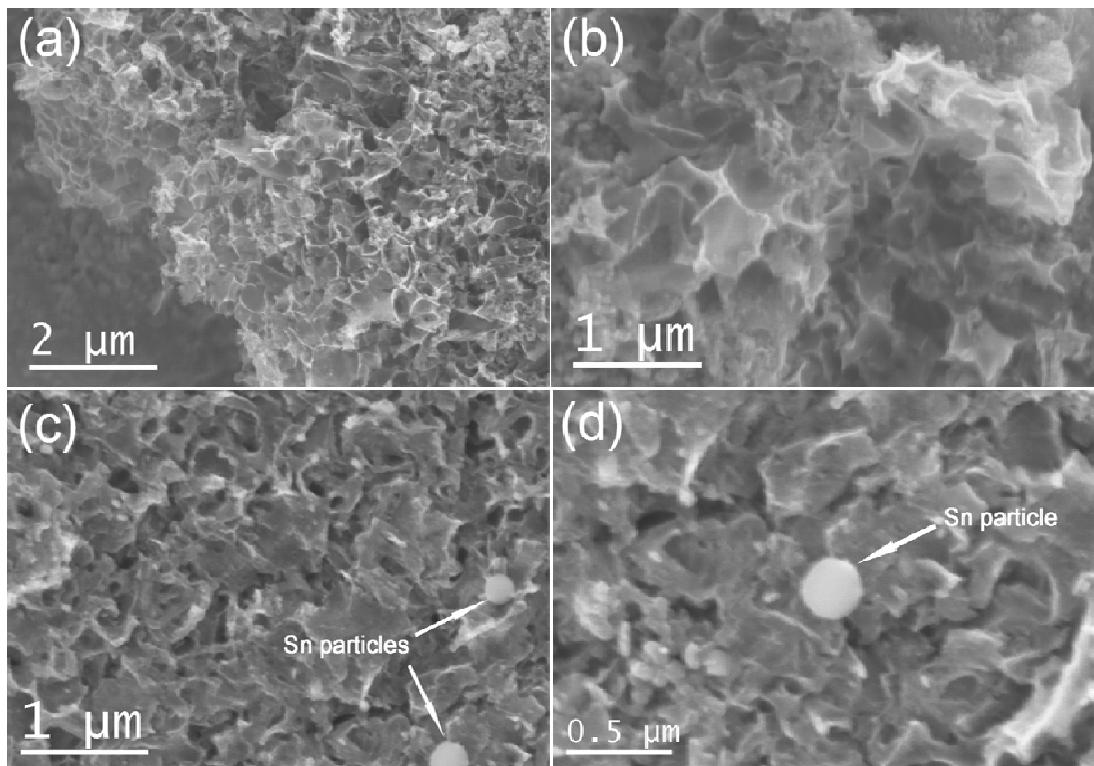
Fig. S9 (a, b) Typical SEM images of a M-Sn<sub>2</sub>Nb<sub>2</sub>O<sub>7</sub>/SnO<sub>2</sub>@3DC electrode after 100 electrochemical cycles; (c, d) Typical SEM images of a SnO<sub>2</sub>/3DC electrode after 100 electrochemical cycles.
