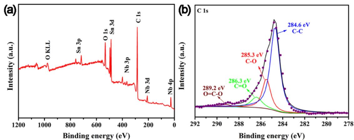
Fig. S6 (a) XPS survey scan of  $\text{SnO}_2/\text{Sn}_2\text{Nb}_2\text{O}_7@3\text{DC}$  hybrids; (b) High resolution XPS spectra for C.
