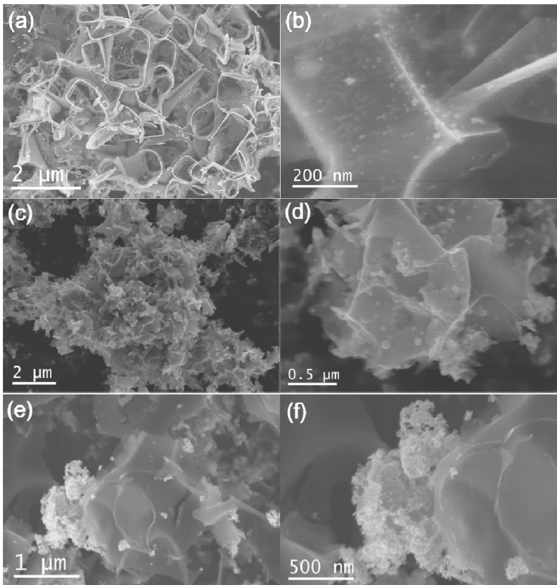
Fig. S5 Typical SEM images of (a, b) SnO<sub>2</sub>/3DC; (c, d) Nb<sub>2</sub>O<sub>5</sub>/3DC and (e, f) SnO<sub>2</sub>/Nb<sub>2</sub>O<sub>5</sub>/3DC.
