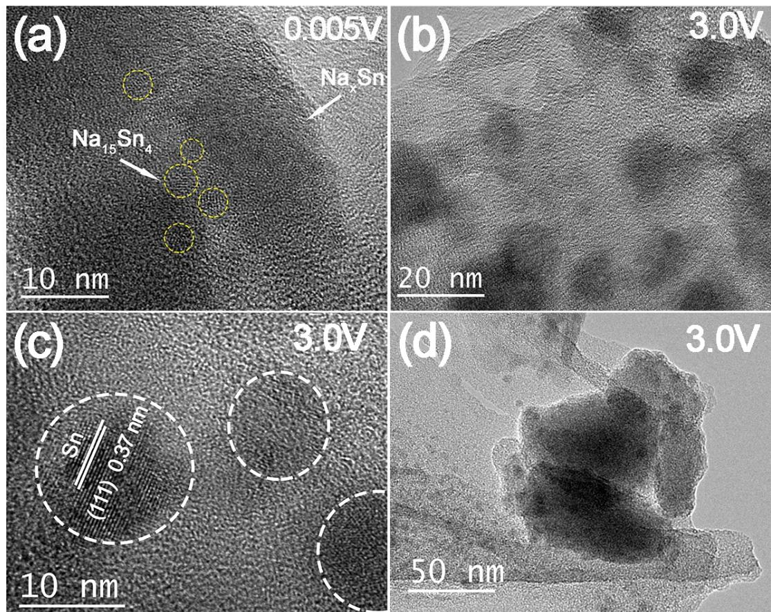
Fig. S13 (a) HRTEM image of M-Sn<sub>2</sub>Nb<sub>2</sub>O<sub>7</sub>/SnO<sub>2</sub>@3DC electrode material obtained at the discharged voltage of 0.005V; (b, c) charged voltage of 3.0V and (d) TEM image at the charged voltage of 3.0V.
