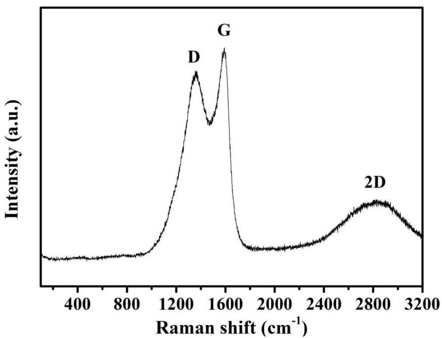
Fig. S3 Raman spectrum of  $\text{SnO}_2/\text{Sn}_2\text{Nb}_2\text{O}_7@3\text{DC}$  hybrids.
