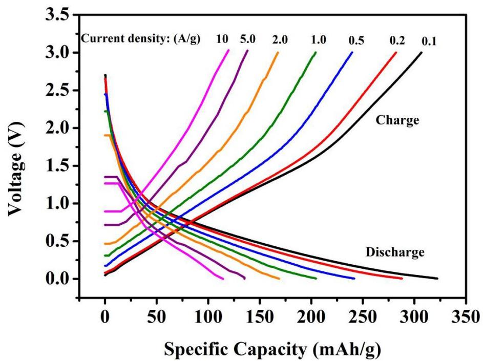
Fig. S8 Galvanostatic discharge/charge profiles of the  $\text{M-Sn}_2\text{Nb}_2\text{O}_7/\text{SnO}_2@3\text{DC}$  electrode at various current densities of  $0.1, 0.2, 0.5, 1.0, 2.0, 5.0$ , and  $10 \text{ A g}^{-1}$ .
