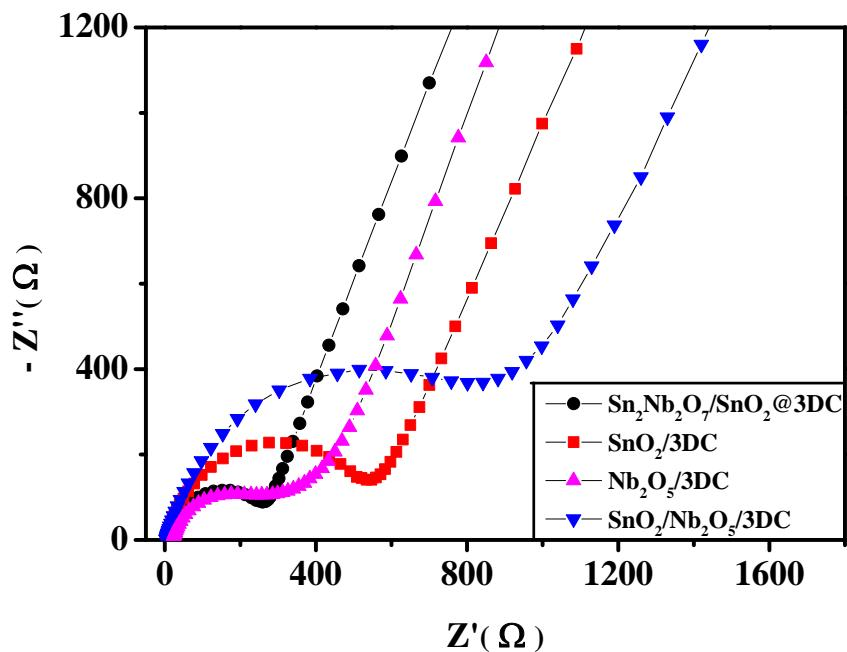
Fig. S11 Nyquist plots of M- $\text{Sn}_2\text{Nb}_2\text{O}_7/\text{SnO}_2@3\text{DC}$ ,  $\text{SnO}_2@3\text{DC}$ ,  $\text{Nb}_2\text{O}_5/3\text{DC}$  and mechanical mixing of  $\text{SnO}_2/\text{Nb}_2\text{O}_5/3\text{DC}$  electrodes after the rate tests over the frequency range from  $100 \text{ kHz}$  to  $10 \text{ mHz}$ .
