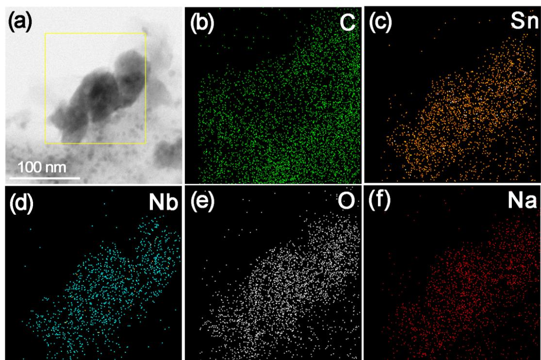
Fig. S15 (a) STEM BF image and the corresponding elemental mapping images of (b) carbon; (c) tin; (d) niobium; (e) oxygen and (f) sodium.
