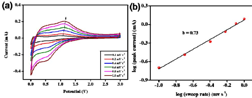
Fig. S10 (a) Cyclic voltammetry curves of  $\text{SnO}_2@3\text{DC}$  electrode at different scan rate ranging from  $0.1$  to  $1.0 \text{ mV}^{-1}$ ; (b) Plot of  $\log(i)$  vs  $\log(v)$  of anodic peaks (red spheres) and corresponding  $b$ -value determination (black lines) according to the power law ( $i = av^b$ ). The  $b$  value is  $0.73$  indicating that the electrochemical reactions of  $\text{SnO}_2@3\text{DC}$  electrode is mainly diffusion-controlled.
