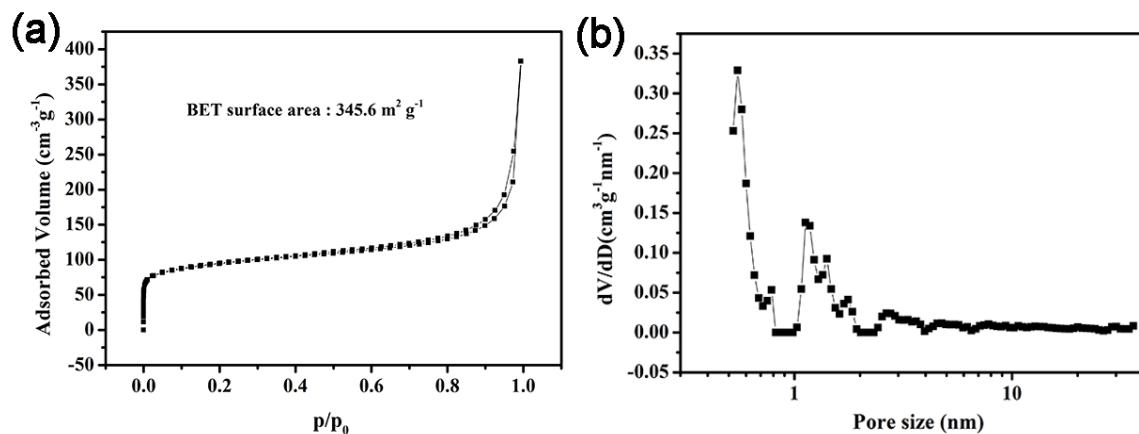
Fig. S7 (a) Nitrogen adsorption-desorption isotherms and (b) DFT pore size distribution curve of  $\text{SnO}_2/\text{Sn}_2\text{Nb}_2\text{O}_7@3\text{DC}$ .
