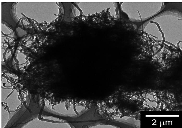
Fig.S1. The typical TEM image of the prepared CNT-NWs@Na<sub>3</sub>TM composite.
