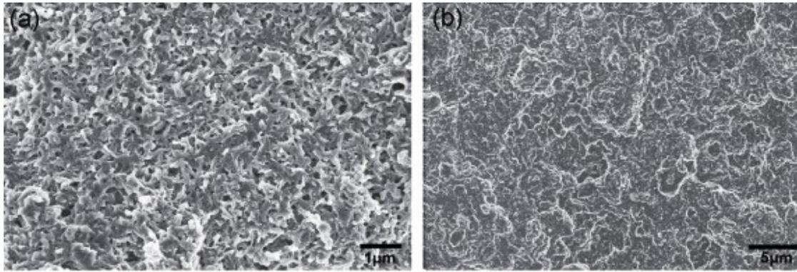
**Fig. S5.** The SEM images of the CNT-NWs@Na<sub>3</sub>TM electrodes after 100 cycles tested at 0.5 A g<sup>-1</sup>.
