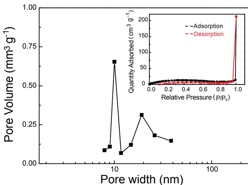
**Fig. S4.** The pore size distribution pattern of the pure Na<sub>3</sub>TM microparticles calculated from the corresponding N<sub>2</sub> adsorption/desorption isotherm (inset).
