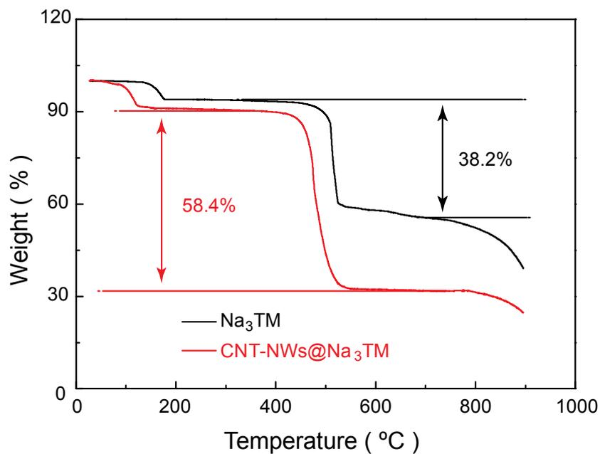
**Fig. S3.** The comparison of TGA curves between the prepared CNT-NWs@Na<sub>3</sub>TM composite and pure Na<sub>3</sub>TM. Both tests were carried out under the air atmosphere at the heating rate of 10 °C/min.
