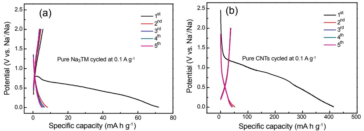
**Fig. S6.** The galvanostatic charge/discharge curves of the initial 5 cycles for the electrode of (a) pure Na<sub>3</sub>TM material and (b) pure CNTs material at the current density of 0.1 A g<sup>-1</sup> between 0.01 V and 2 V vs. Na<sup>+</sup>/Na.
