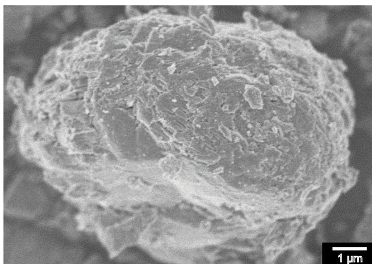
**Fig. S2.** The SEM image of pure Na<sub>3</sub>TM microparticles.
