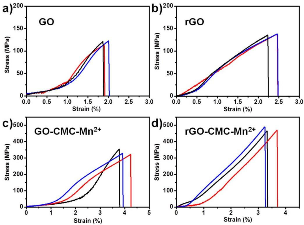
**Figure S4.** The stress-strain curves of pure GO film, rGO film, GO-CMC-Mn<sup>2+</sup> nanocomposites, and rGO-CMC-Mn<sup>2+</sup> bioinspired nanocomposites, demonstrating the resultant rGO-CMC-Mn<sup>2+</sup> nanocomposites have excellent mechanical properties, superior to GO, rGO and GO-CMC-Mn<sup>2+</sup> materials.
