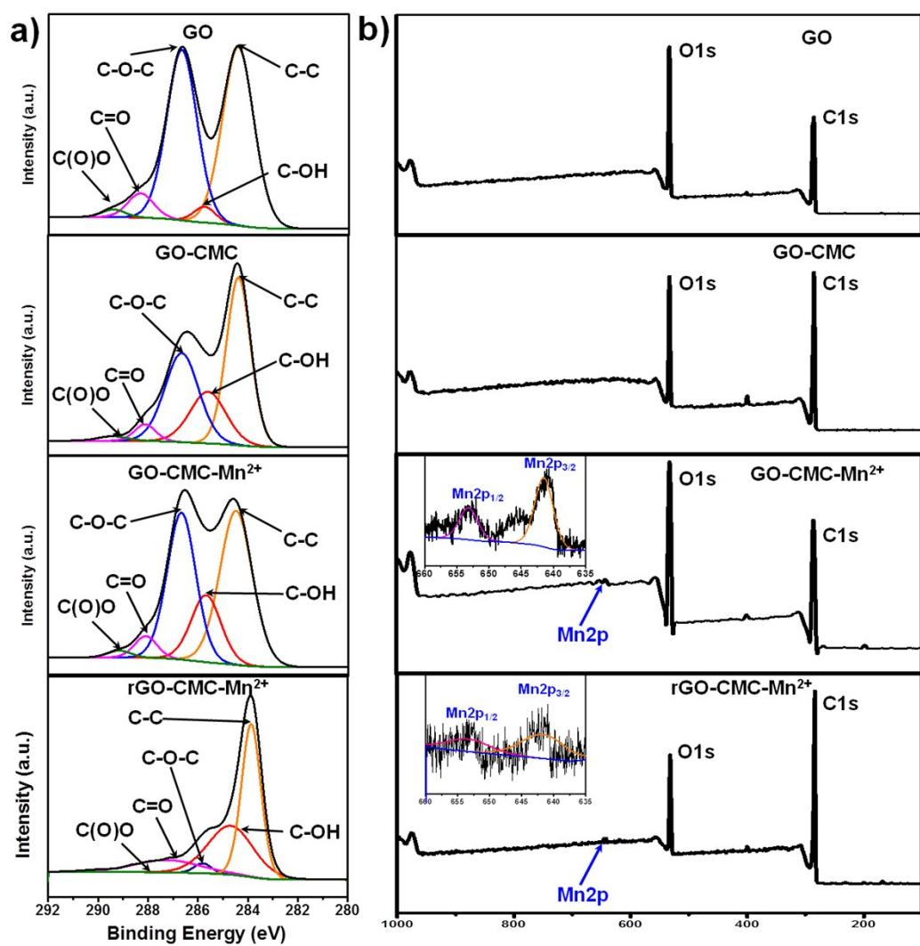
**Figure S3.** (a) C1s XPS survey spectra of pure GO film, GO-CMC, GO-CMC- $\text{Mn}^{2+}$  and rGO-CMC- $\text{Mn}^{2+}$  nanocomposites and (b) the corresponding whole spectrum.
