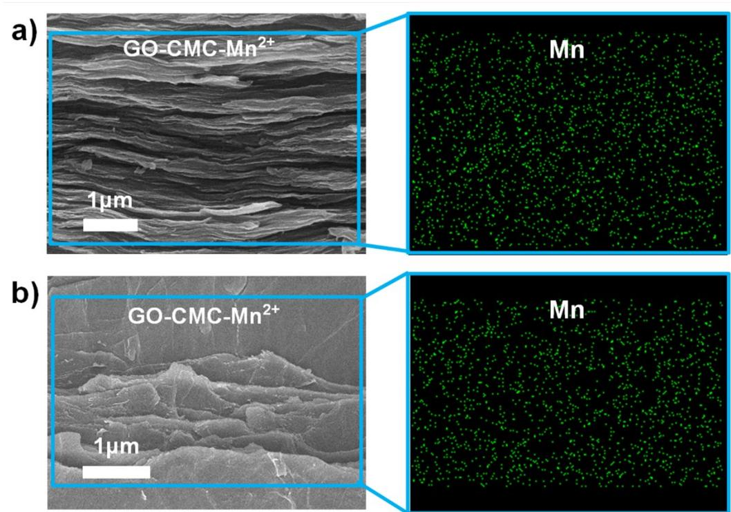
**Figure S7.** a) The cross-section morphology and EDS of the GO-CMC-Mn<sup>2+</sup> nanocomposites. b) The vertical view morphology and EDS of the GO-CMC-Mn<sup>2+</sup> nanocomposites. The EDS results indicate the uniform distribution of Mn element in the GO-CMC-Mn<sup>2+</sup> nanocomposites.
