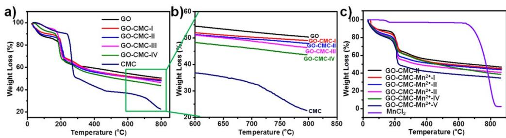
**Figure S1.** a) and b) TGA curves of pure GO and CMC films, and GO-CMC hybrid layered materials with different CMC contents. c) TGA curves of MnCl<sub>2</sub> power, GO-CMC-II and GO-CMC-Mn<sup>2+</sup> composite films with different Mn<sup>2+</sup> contents. The curves were obtained under the atmosphere of nitrogen with a temperature rising rate of 10°C·min<sup>-1</sup>.
