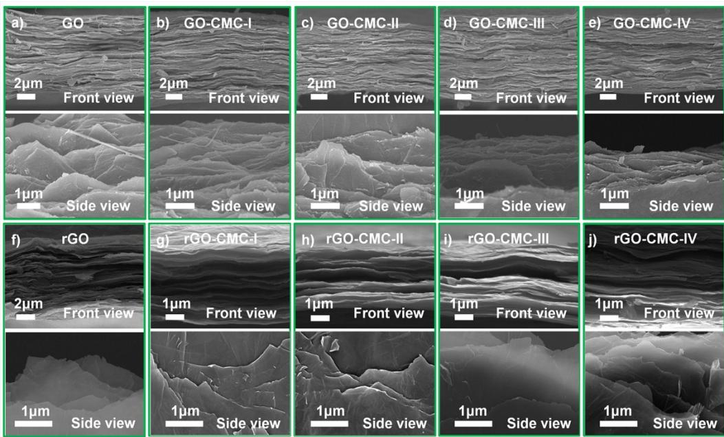
**Figure S5.** The front and side view fracture morphologies of pure GO film and GO-CMC nanocomposites, respectively. a) GO film, b) GO-CMC-I, c) GO-CMC-II, d) GO-CMC-III, e) GO-CMC-IV, f) rGO, g) rGO-CMC-I, h) rGO-CMC-II, i) rGO-CMC-III, and j) rGO-CMC-IV nanocomposites, respectively.
