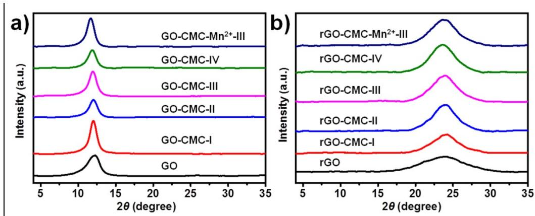
**Figure S2.** XRD spectrum of pure GO film, GO-CMC and GO-CMC-Mn<sup>2+</sup>-III composite films (a) before and (b) after chemical reduction, respectively. The  $d$ -spacing of the nanocomposites rises with the increasing of CMC polymer and the introducing of Mn<sup>2+</sup>.
