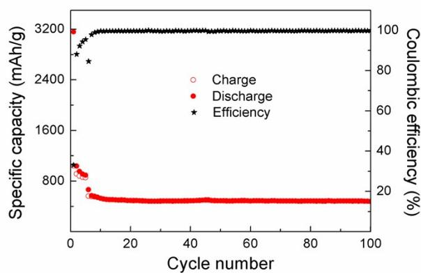
**Figure S4.** The cycle performance of the Si anode without Ti layer modification at  $2.0 \text{ A g}^{-1}$  after an initial activation at  $0.2 \text{ A g}^{-1}$  for 5 cycles.
