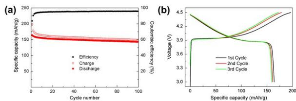
**Figure S10.** (a) Cycle performance of the casted  $\text{LiCoO}_2$  electrode at a current density of  $50 \text{ mA g}^{-1}$  over a potential window of  $3.0\text{-}4.5 \text{ V}$ . (b) Corresponding galvanostatic charge/discharge
