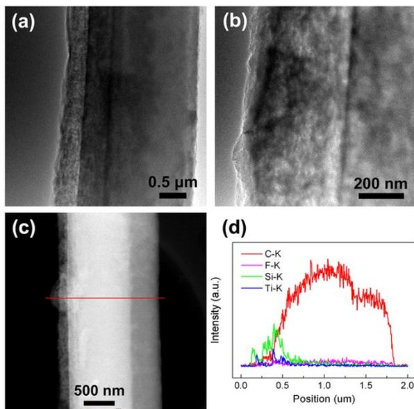
**Figure S8.** (a, b) TEM images, (c) STEM image and (d) corresponding EDX line scan curves of the Si electrode after 1000 cycles and another 300 cycles for rate test. It can be seen that the active Si material and Ti modification layer are still adhered onto the carbon foam framework after long-term cycle.
