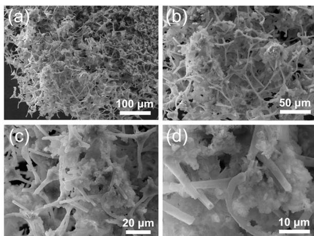
**Figure S7.** SEM images of the Si electrode after 1000 cycles and another 300 cycles for rate test. It can be found that the cycled electrode maintains its original three-dimensional network structure, and the active Si material is still adhered onto the carbon foam framework.
