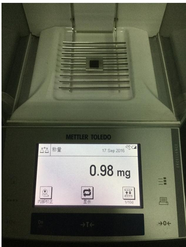
**Figure S2.** Optical photograph of one piece of carbon foam ( $1\times 1\times 0.1\text{ cm}^3$ ) on an analytical balance.
