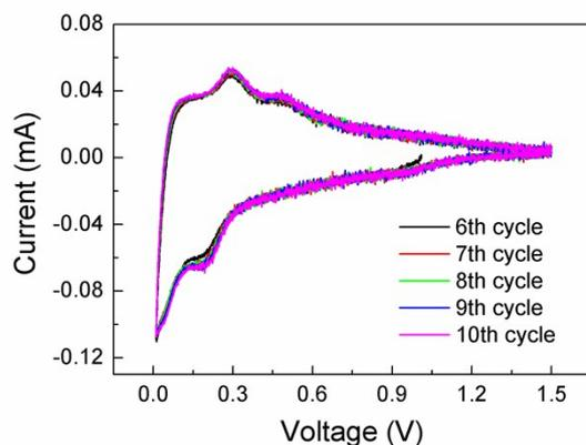
**Figure S6.** CV curves from the 6th to 10th cycle for the Si electrode tested at a scan rate of 0.02 mV s<sup>-1</sup> over a potential window of 0.01-1.5 V versus Li/Li<sup>+</sup>. The almost coincident CV profiles demonstrate that the electrode tends to stabilize after an activation in the initial several cycles.
