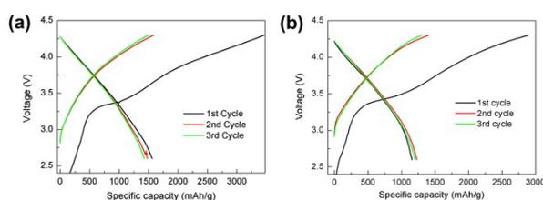
**Figure S11.** The initial three galvanostatic charge/discharge cycles of the Si/LCO full cell at (a) 1.0 A g<sup>-1</sup> and (b) 2.0 A g<sup>-1</sup>.
