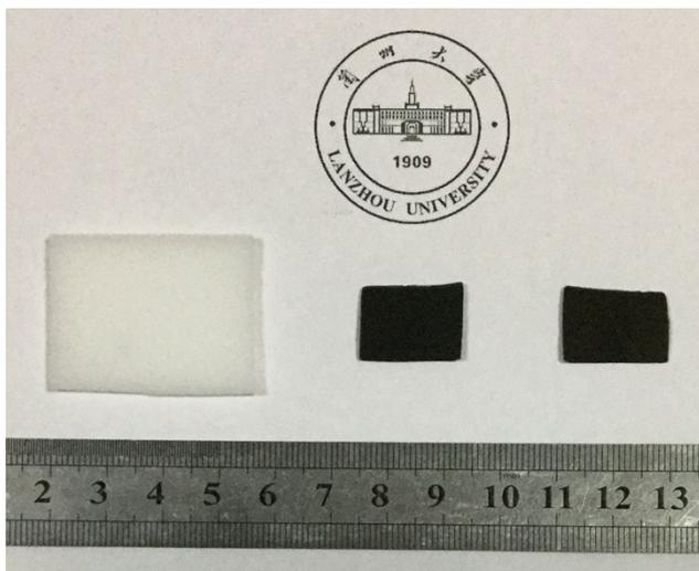
**Figure S1.** Optical photographs of the used melamine formaldehyde foam (left), carbon foam (middle) and as-deposited Si anode (right).
