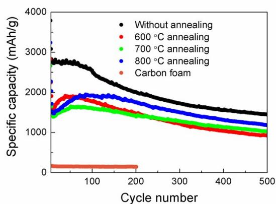
**Figure S5.** Cycle performances at a current density of  $2.0 \text{ A g}^{-1}$  for the carbon foam, Si electrode without annealing, and Si electrodes annealed respectively at 600, 700, and 800 °C.
