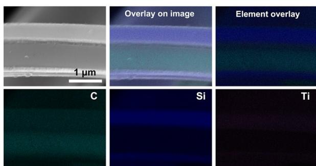
**Figure S3.** The EDS element mappings of the as-deposited carbon foam/Ti/Si electrode shown in the inset of Figure 2d. We can find the Ti layer and Si layer deposited on the carbon foam.
