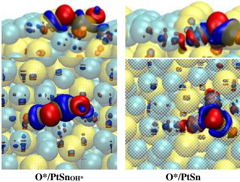
**Fig. S2** Induced charge of  $O^*$  on  $PtSnOH^*$  (denoted as a spectator  $OH^*$  on the  $PtSn$ ) and  $PtSn$ . The isosurface of  $\pm 0.02 |e|$  are shown in the opaque blue/red lobes. The Pt, Sn and O atoms are represented as transparent cyan, yellow and orange spheres, respectively. Less induced charge in  $O^*/PtSnOH^*$  interface indicates the weaker  $E_{ads}(O^*)$  on  $PtSnOH^*$  due to the lateral repulsion between the adsorbed  $O^*$  and spectator  $OH^*$ .
