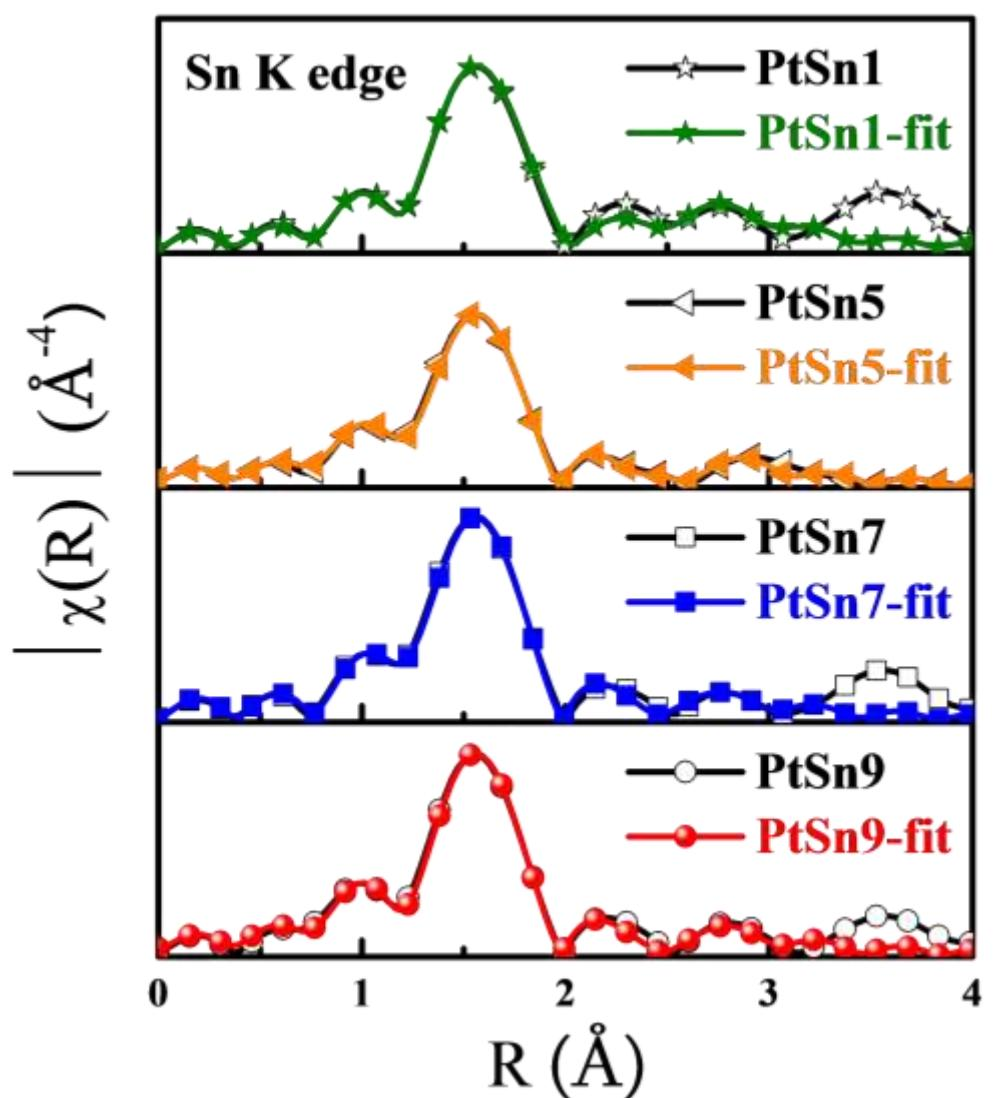
**Fig. S10** The EXAFS fitting results of as-prepared PtSn samples for Sn K edge.
