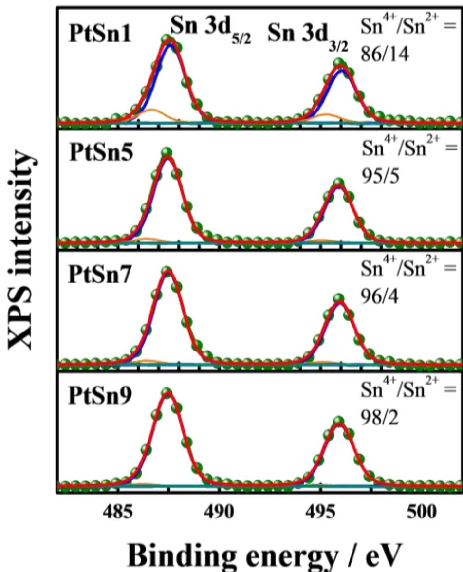
**Fig. S7** XPS spectra of Sn and fitting results for various PtSn samples.
