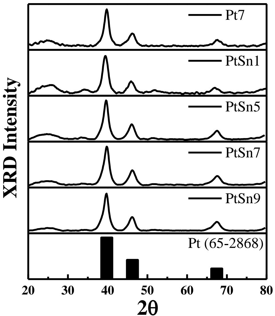
**Fig. S5** XRD patterns of Pt7 and various PtSn samples.
