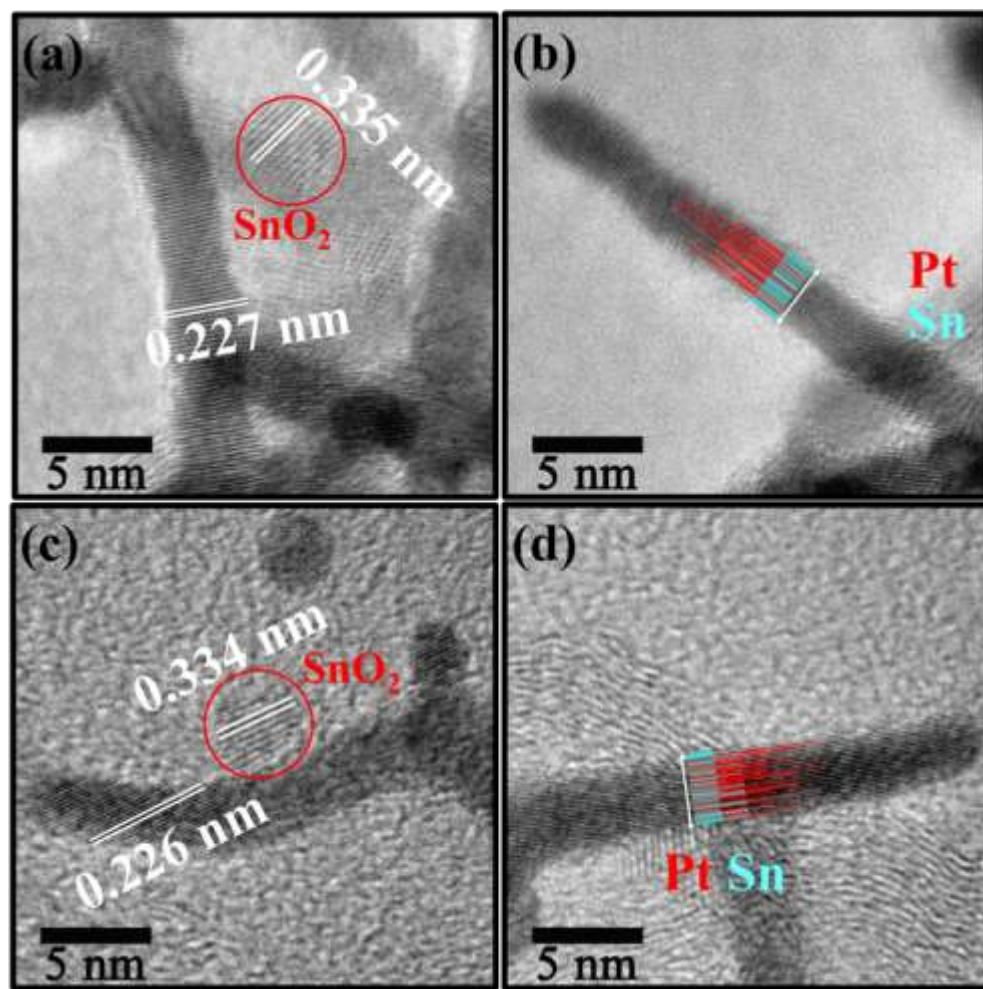
**Fig. S4** The local TEM micrographs and line scans results for as-prepared PtSn9 (a) and (b), and PtSn9 after ADT (c) and (d), respectively.
