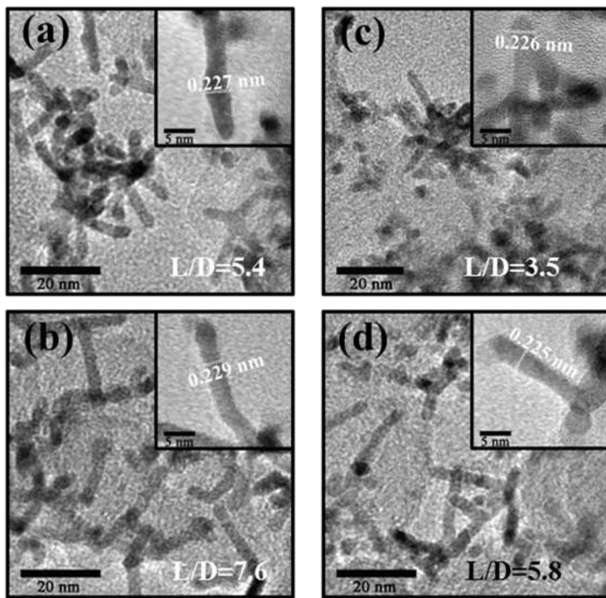
**Fig. S3** HRTEM micrographs of catalysts before and after ADT for PtSn5 (a) and (c), and PtSn7 (b) and (d), respectively.
