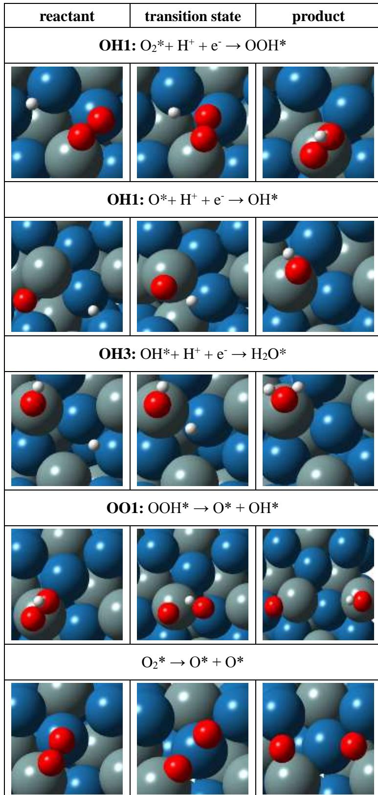
**Fig. S1.** Optimized structures for local minima and transition states of the five elementary steps in ORR on (a) Pt, (b)  $PtSn_{0^*}$  and (c) PtSn. The corresponding energetic results are listed in Table S1 and the related potential energy surfaces are compared in Fig. 1. Cyan, tan, red and white spheres are represented as Pt, Sn, O and H atoms, respectively. The spectator  $O^*$  in  $PtSn_{0^*}$  surface is marked by orange sphere.
