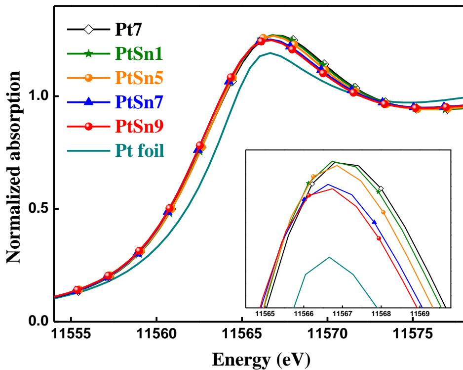
**Fig. S8** The XANES spectra of as-prepared PtSn samples for Pt L<sub>III</sub> edge.
